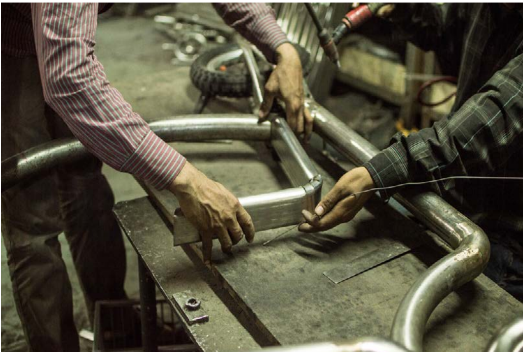
■ Checking the kids seat rear tube
