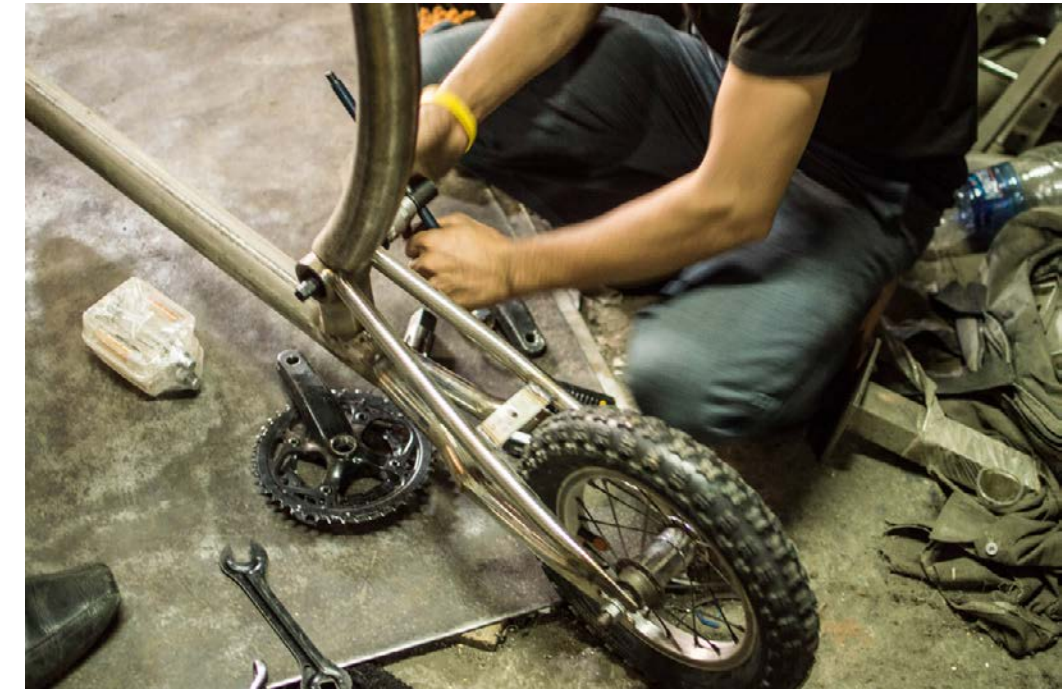
■ Fitting the bottom bracket and crankset
