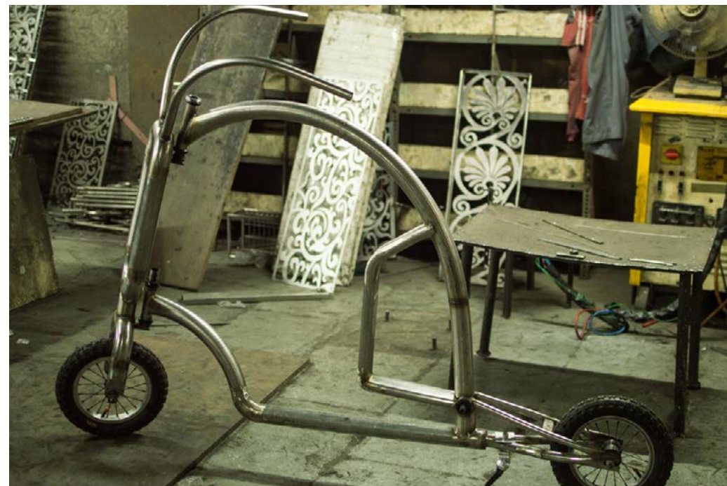
■ Frame before seat post fixing
