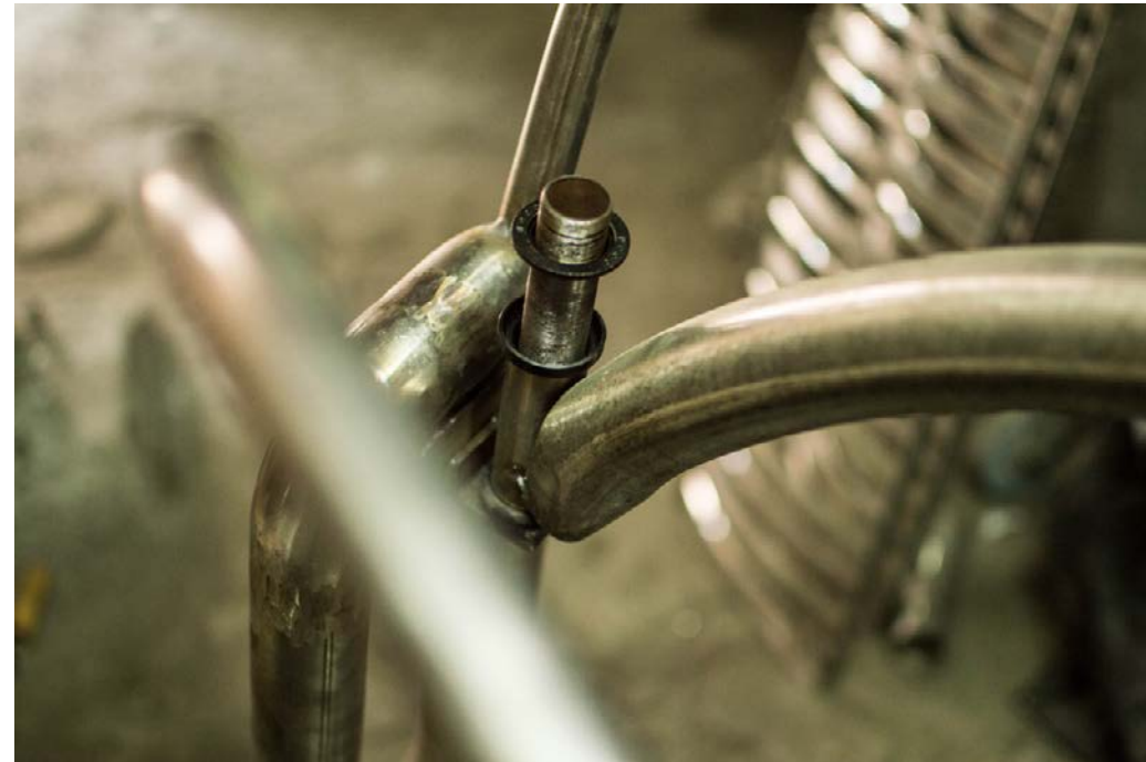
■ Head tube connection top tube
