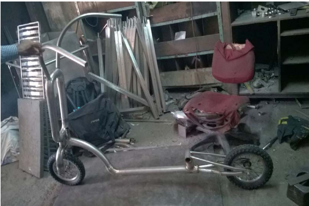
■ Fixing down tube and head tube
