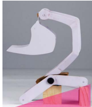
Work space stays upright during descend.
