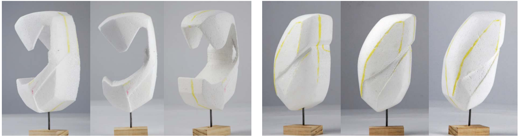
Form and volume verified on PS Foam mockups.
