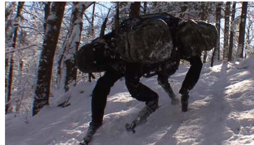
BigDog is a dynamically stable quadruped robot created in 2005 by Boston Dynamics.
