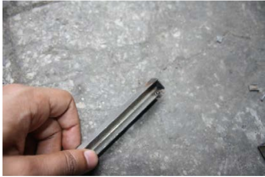
Half inch sided C-channels and square extruded SS cut out in required size
