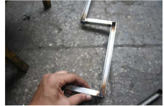
Square tubes and c-channels welded together forming a path for wiring
