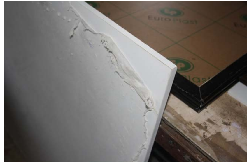
Corian laminate of same size pasted on all visible sides of the board
