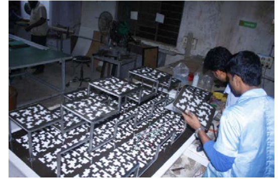
A total of 19 plates fixed into the slots, completing the assembly
