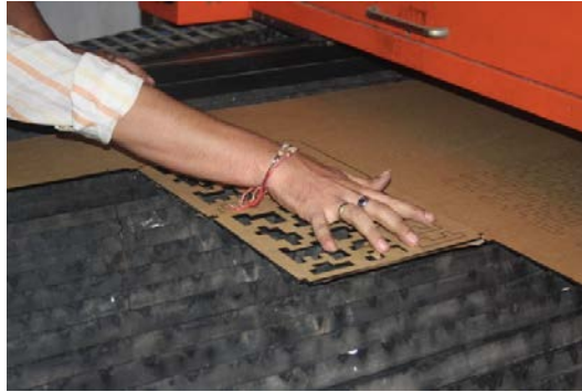
Patterned plates of 10in*8in (19 numbers) laser cut
