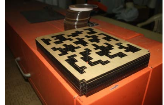
19 plates laser cut and the edges buffed for attaining good lighting later
