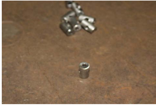
Lower fitment of steel cable to be welded on channel nodes for extra support
