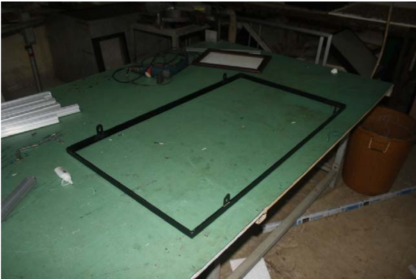
4 feet * 2 feet, one inch L-angle MS frame fabricated for fixing on top of the board, providing it extra strength and support
