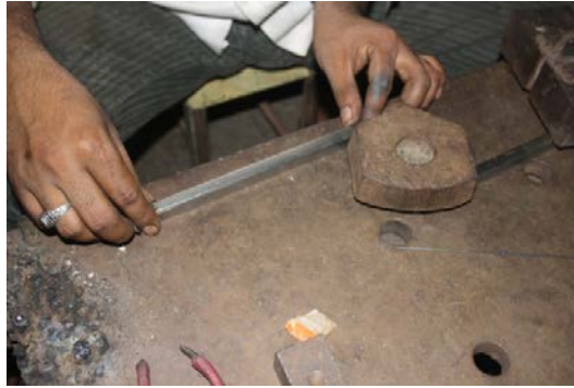
Open ends of C-channel packed and welded and polished (to house panels)
