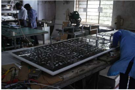
Acrylic plate and channels placed and screwed onto the board
