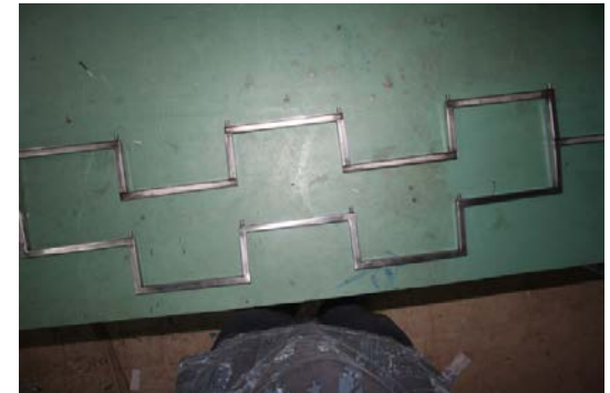
Channels welded together and buffed as per the given design
