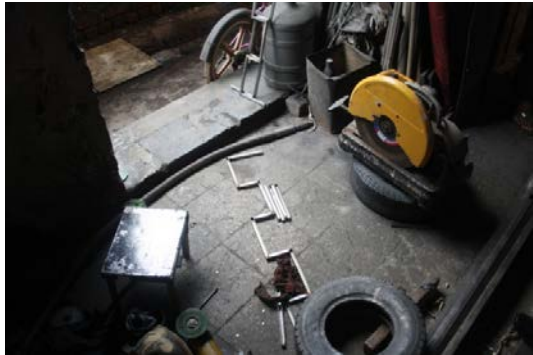
Total length fabricated and weld spots removed
