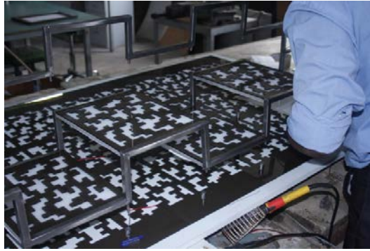
Light panels with patterns wired and fit in the C-channel slots
