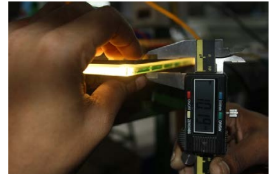
Total thickness of the panel is measured and maintained at 10mm
