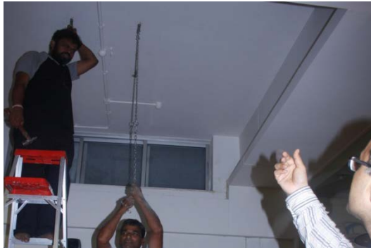
Hook strength tested by pulling at the suspender chains
