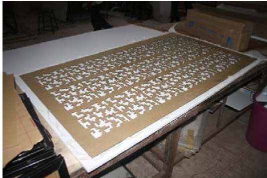
Approx 4.5ft*2.5ft panel of the same material laser cut for placing on top
