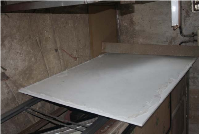
5 feet by 3 feet, half inch ply cut and finished to form the top board of the fixture
