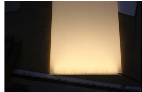
Light spreads out uniformly because of the frosted sheet
