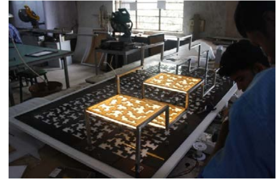
Testing done after placing each panel to ensure proper wiring throughout
