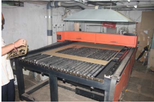
3mm clear grey acrylic sheet placed in the laser cutting machine
