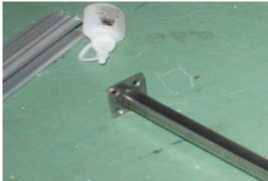
2mm thick SS plate with screw taps welded on both ends for fixing on board
