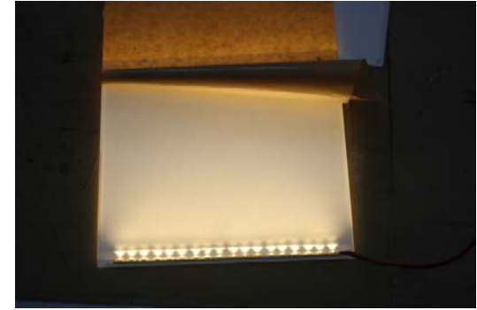
LED strip lighted up on one side for testing. Light spread still uneven
