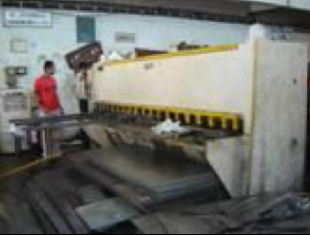
Shearing machine for cutting and flattening
