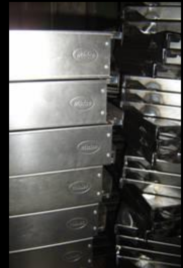
Emboss done during CNC punching
