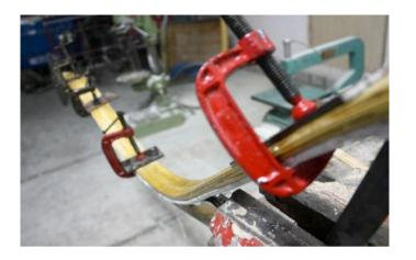
Fig47: the layers clamped with C-clamps are left overnight to set.
