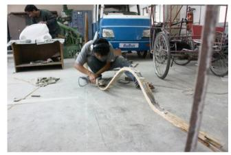
Fig49: finishing the bamboo strips
