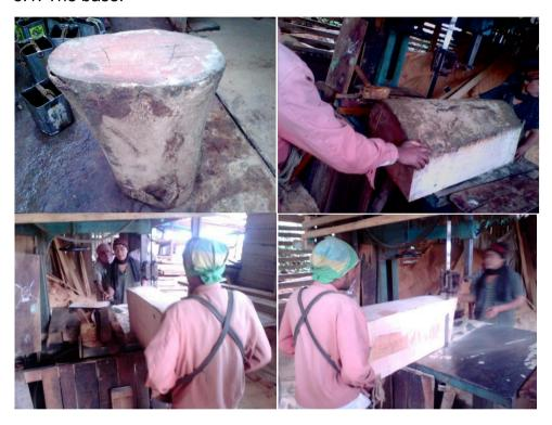
Fig33: cutting the block into size
