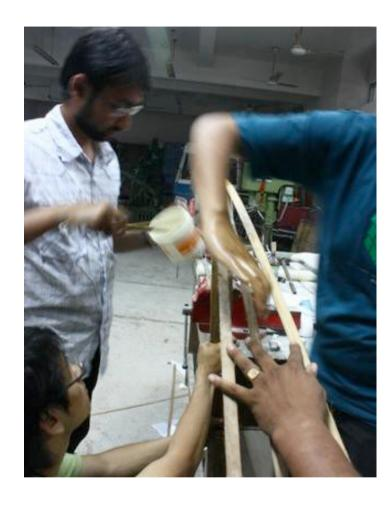
Fig46: bending the bamboo strips and gluing them in layers
