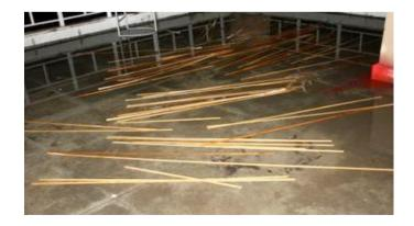
Fig45: the bamboo strips soaked in water before bending.
