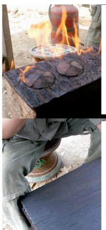
Fig40: leaving the excess wax to burn off
