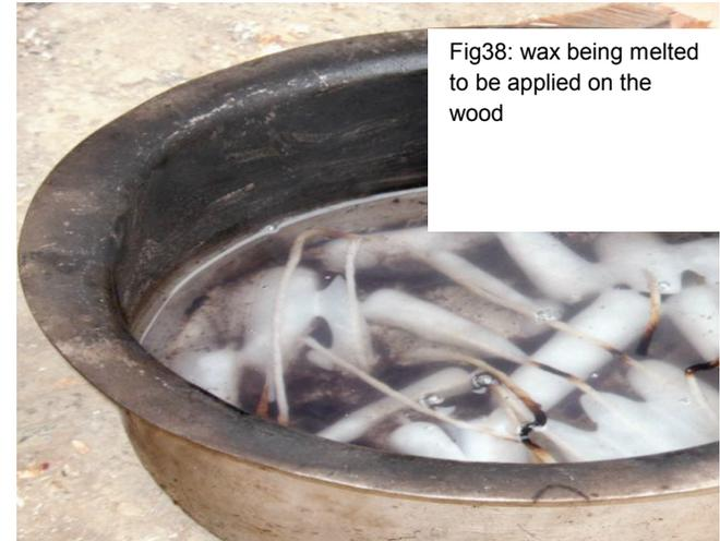
Fig38: wax being melted to be applied on the wood
