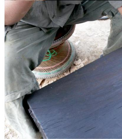
Fig41: sanding the surface to create the aged effect
