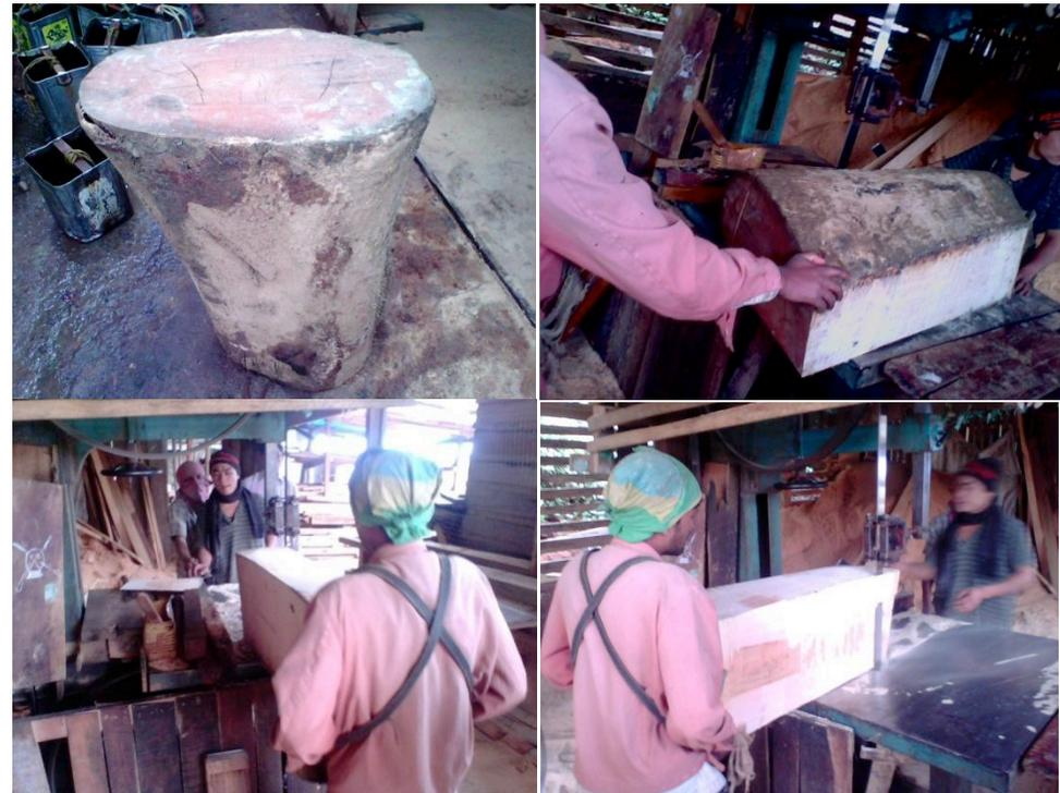
Fig33: cutting the block into size
