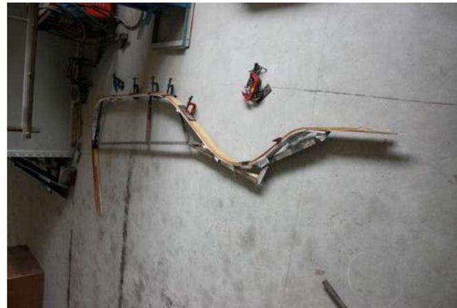
Fig48:the clamps are removed and the strip is separated from the die for finishing.
