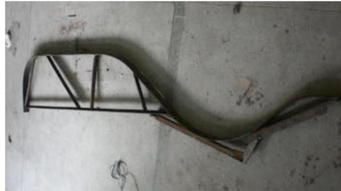
Fig44: metal frame for making the bamboo strips
