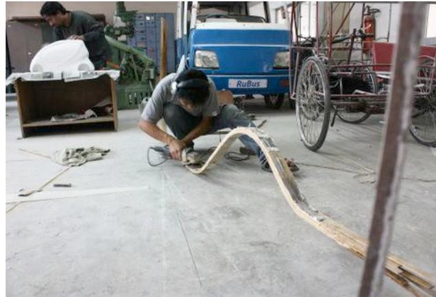
Fig49: finishing the bamboo strips
