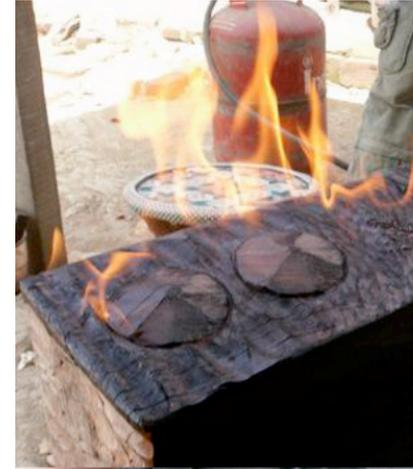
Fig40: leaving the excess wax to burn off
