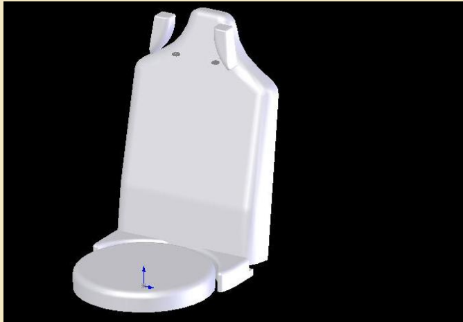
Fig Head rest fused with movable back rest, sleep support is static
