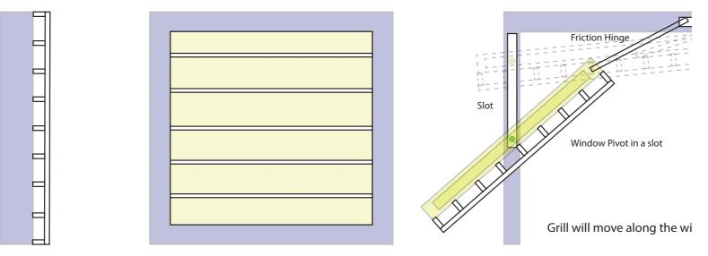
Grill bolted or welded to the frame
