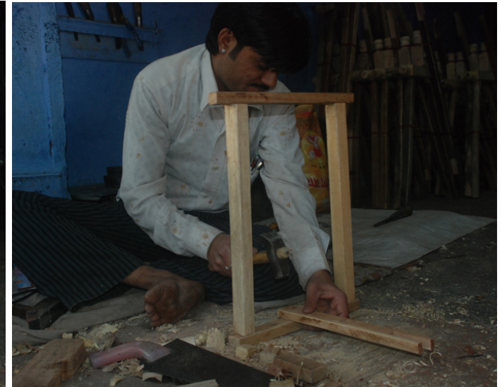
Putting the 14 inches piece at the base.
