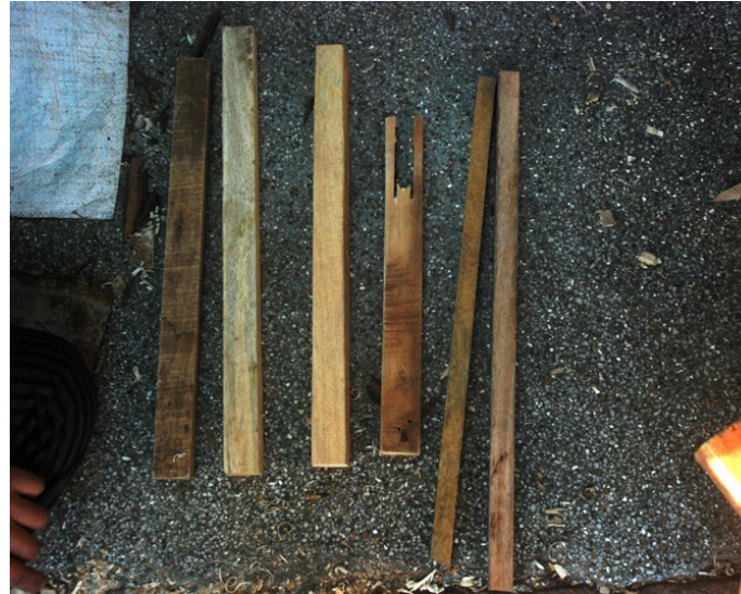
Parts of the final assemblage. 16"x2", 18"x2", 14" and 24" for the slant.
