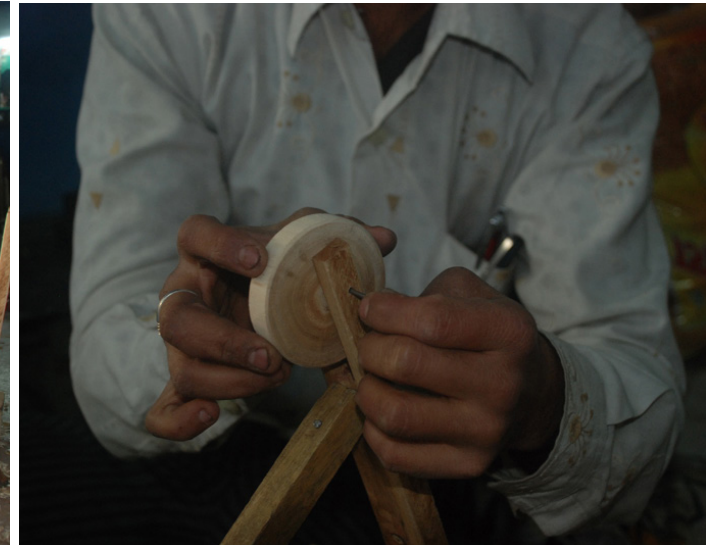
Fixing a wooden wheel, approximately 4 inches in diameter, between the slit of the base using a nail.
