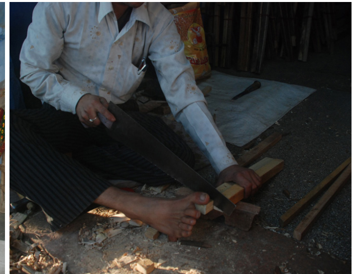
Levelling wood pieces to the desired length.
