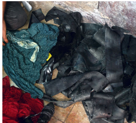
Bicycle tyre- tubes are used to seal the wrapping.
