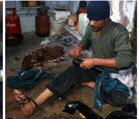
Wrapped tube then tied using strips of tyre- tube.
