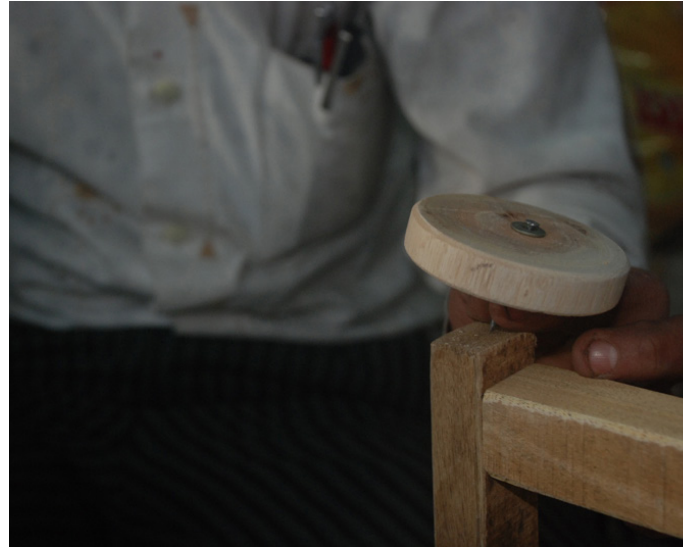
Fixing the wheel on the sides of the walker.
