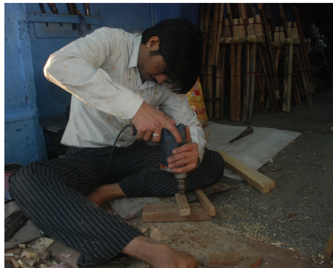
Making hole for joining the pieces.
