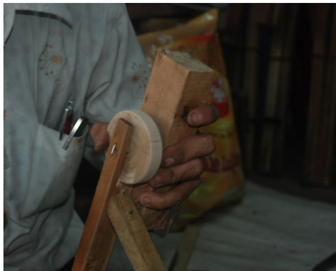
The nail is then bent to prevent the wheel from slipping out.
