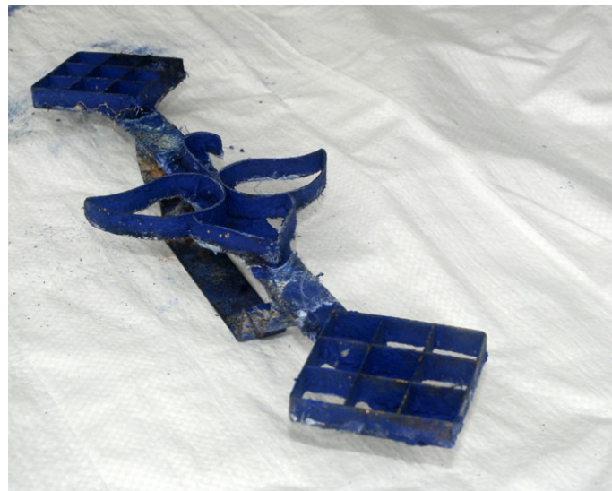
Closer look of a metal stencil, turned blue because of another natural dye, called 'Neel', generally used in washing for whitening the clothes.
