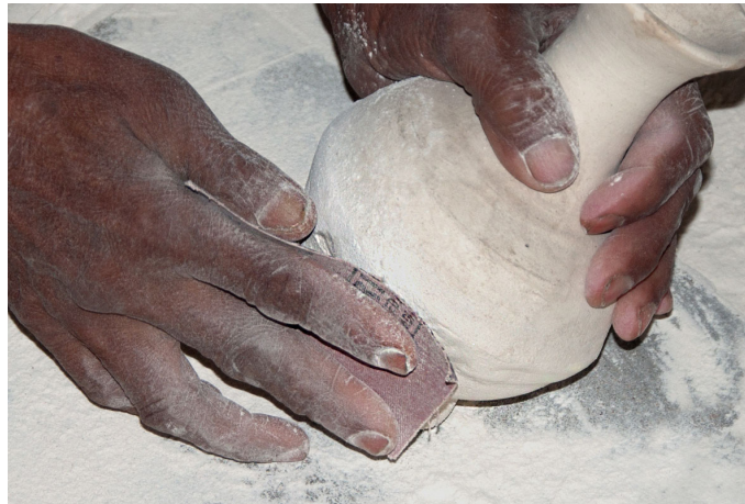
Line formed by extra dough is scrubbed off with sand paper and now vase is scrubbed all over and is ready for the outlines of design to be drawn.
