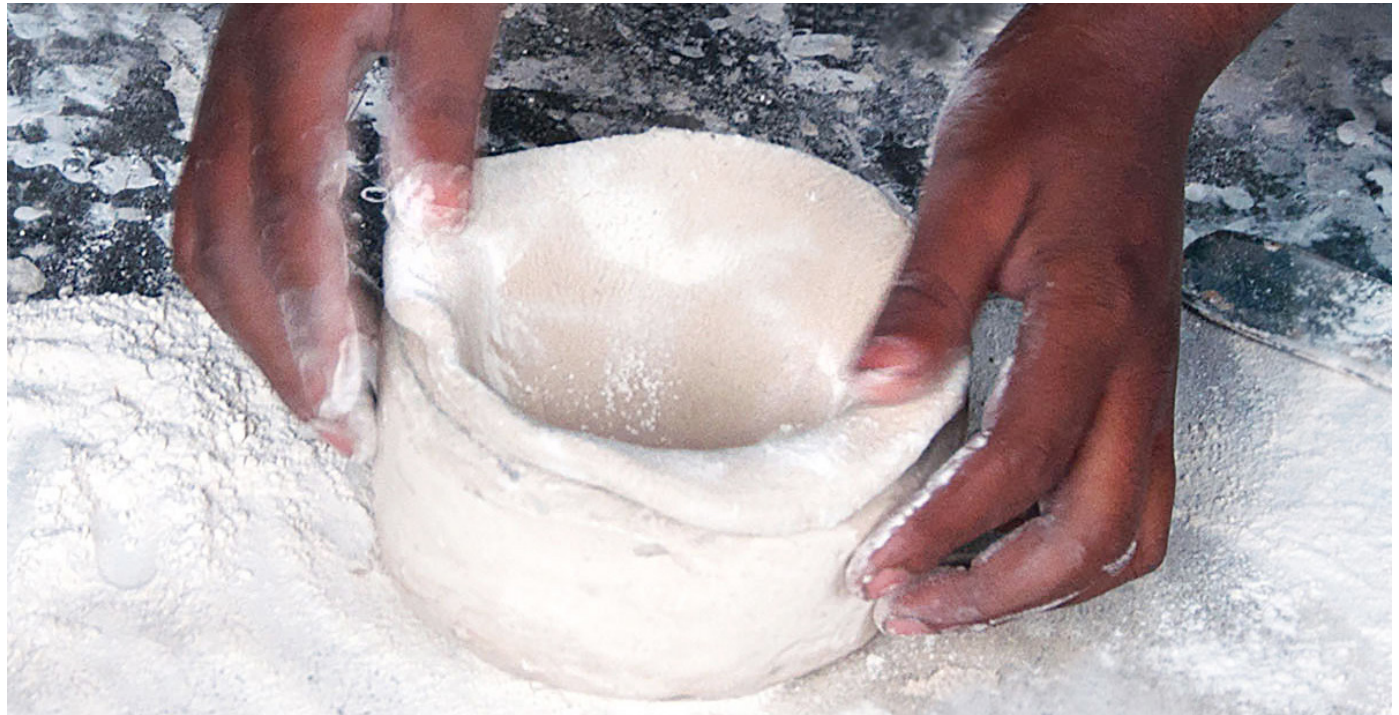
Flattened dough is placed on pop (Plaster of Paris) mold.
