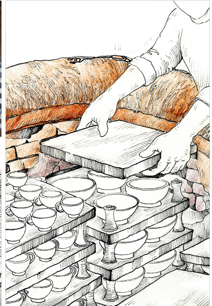
Placing the products in furnace evenly without making them touch each other.
