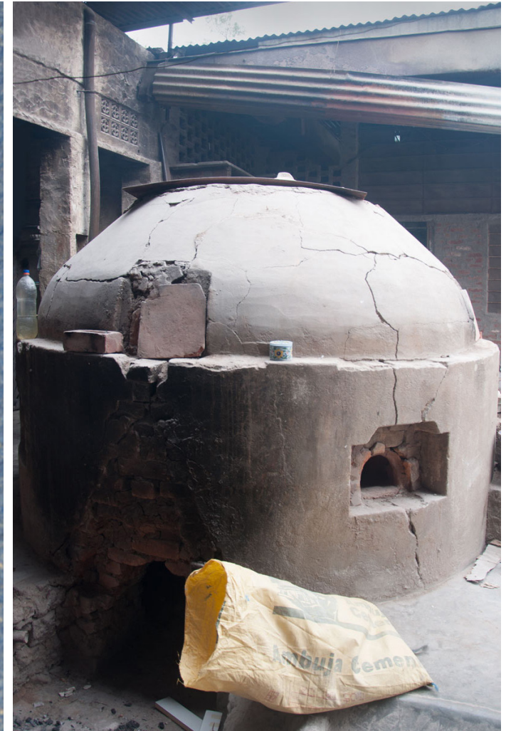
Heating kiln (Furnace)- to dry products to finished ones.
