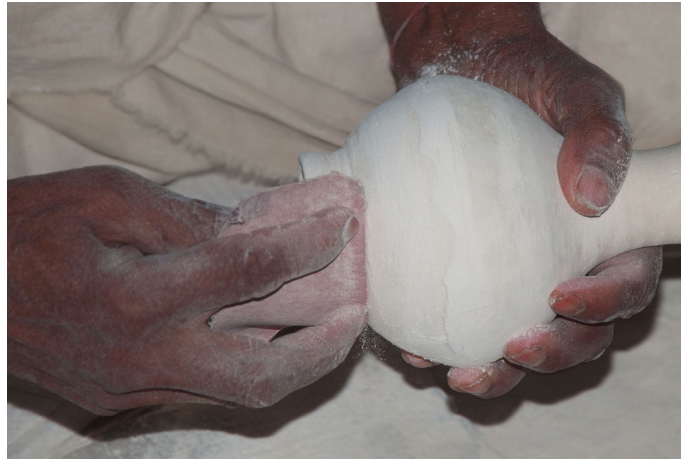
Sand paper is used for smoothening the surface of the product.
