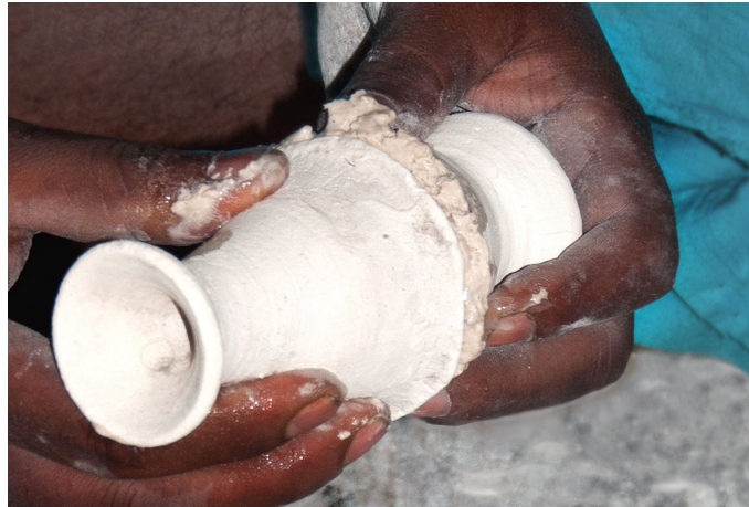
Attaching top and bottom parts of the product forms vase.
