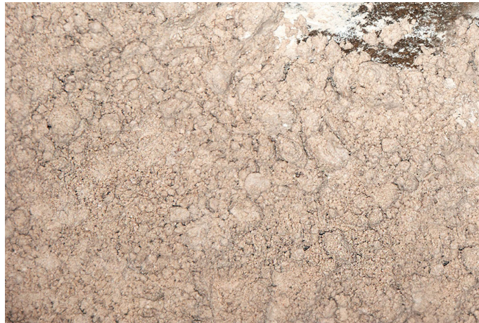
Dough (mixture of kanch stone, katira gond, edible gum, fullers earth, soda bicarbonate, and flour in proper amount, forms the dough).
