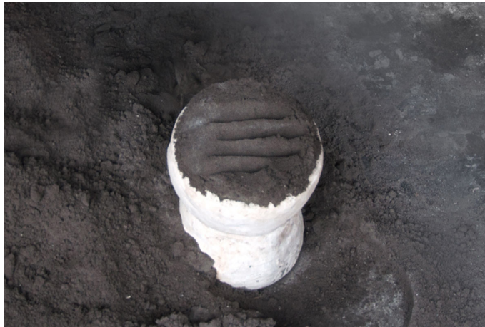
Dough is filled with charcoal to retain shape of mold.
