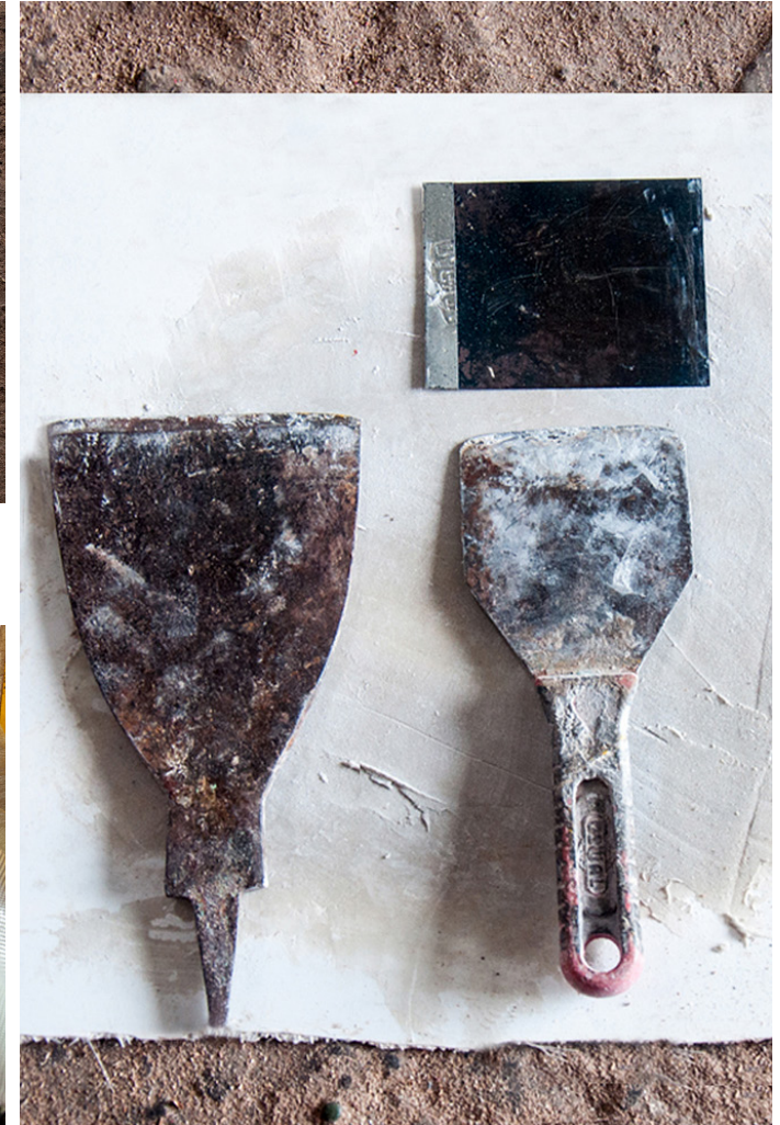
Different kinds of patti blades: These patti blades are used in applying the solution evenly.
