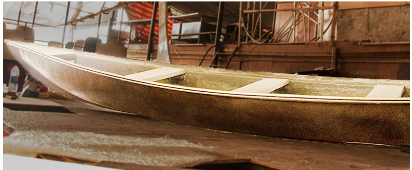
Canoe boat: Canoe boat is often used for recreation purpose. They are very lightweight with open top and both the ends of the boat are pointed.
