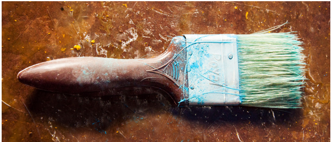
Brush: Brush is used for applying the solution of color, resin and chemicals accordingly.
