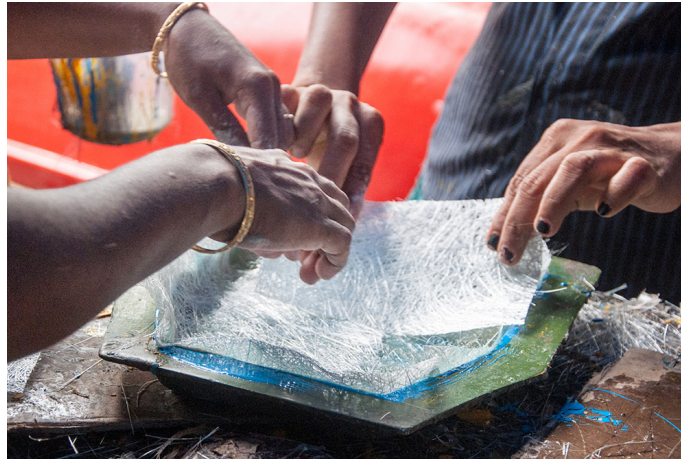
Fiber mats are being applied on the mould by the artisans.
