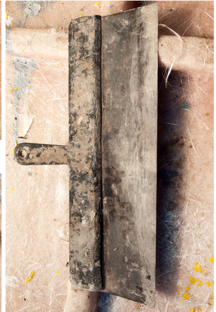
Big size patti blade: This big size patti blade is used in applying the solution evenly on the big surfaces of the boat.
