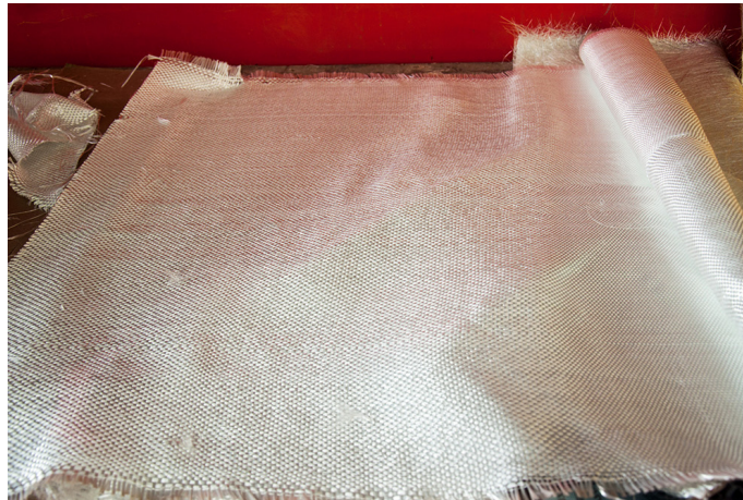
Heat-treated fiberglass mat: This mat is used to strengthen the product like exteriors of the boat. Ex: Base of the boat.
