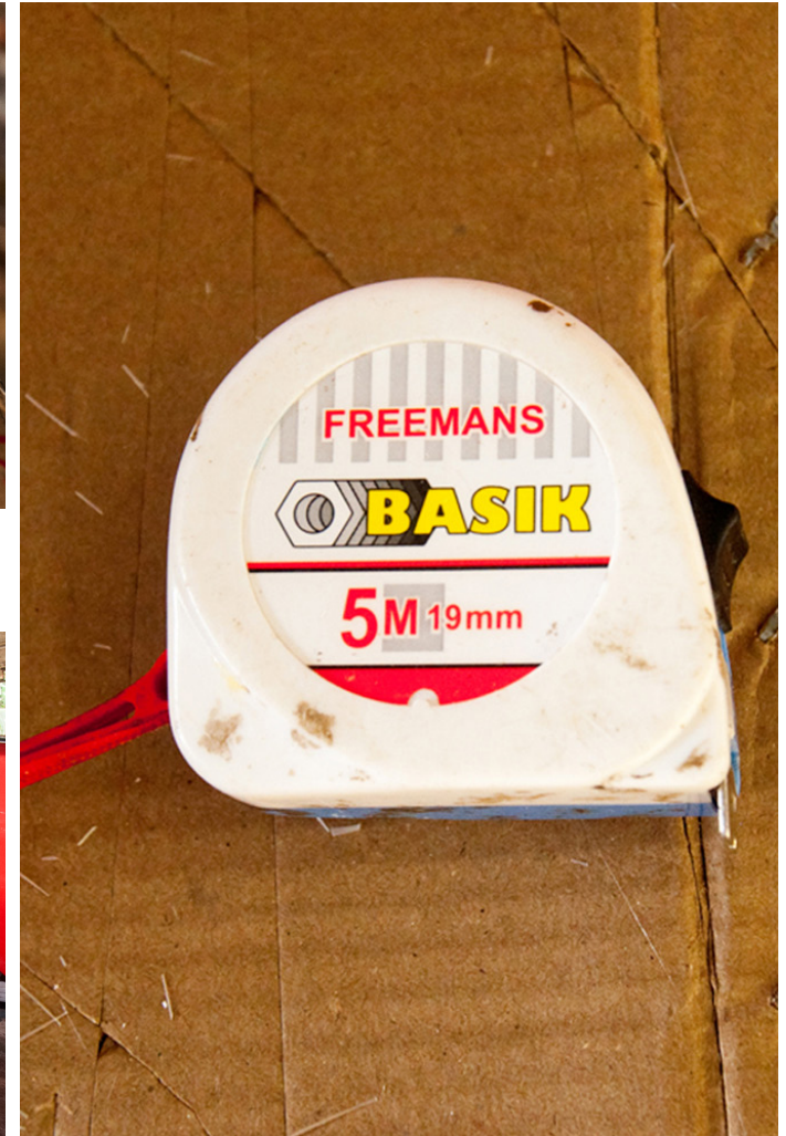
Measuring tape: Required in measuring the boat and its parts while building it.
