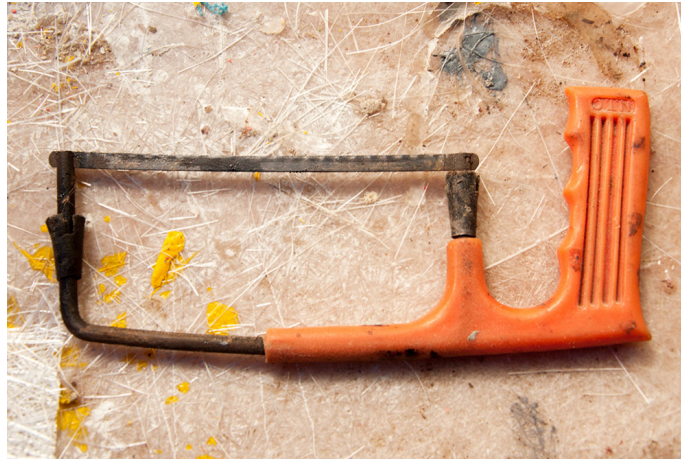
Hacksaw blade with blade holder: This blade is used in cutting the parts of the boat.
