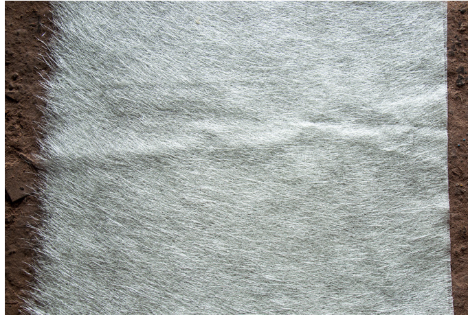
China fiberglass mat: This mat is used to strengthen the product like interiors of the boat.
