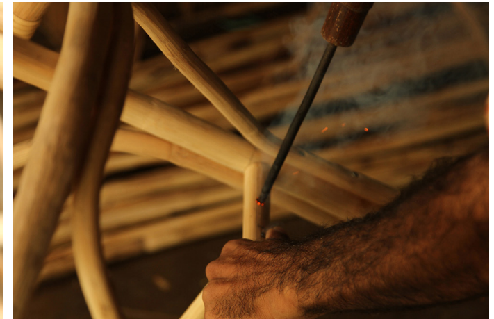
Hot iron rod is pierced through the lower frame of the furniture to create holes.
