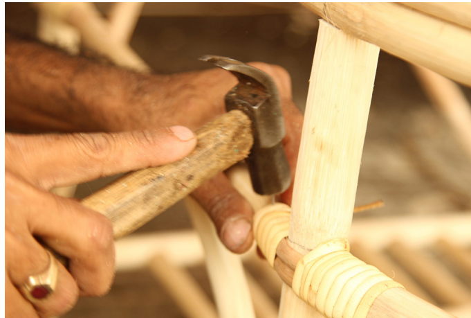
The end of the strip is nailed to the frame.
