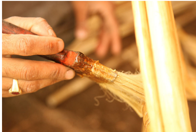
Varnish is applied on the final products for shine.
