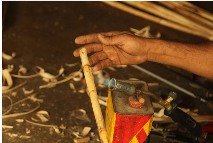
The cut bamboo stick is heated on a slow fire, with a flame touch.
