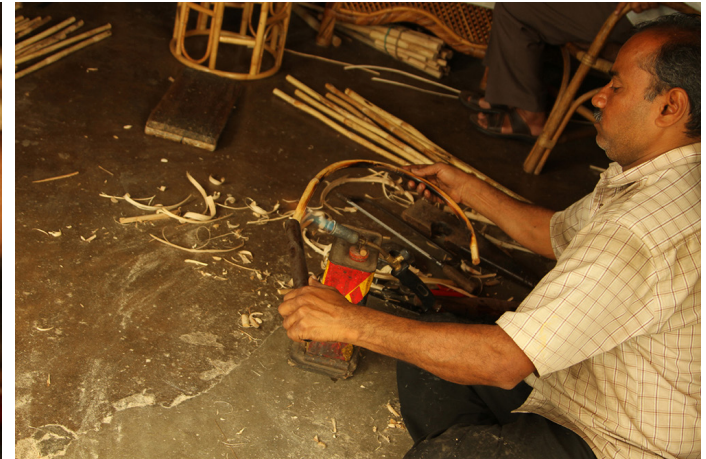
The heating process is done to make the bamboo flexible to bend them.
