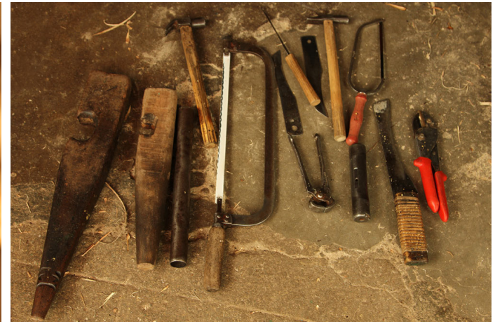
Different types of tools used for making bamboo furniture's.
