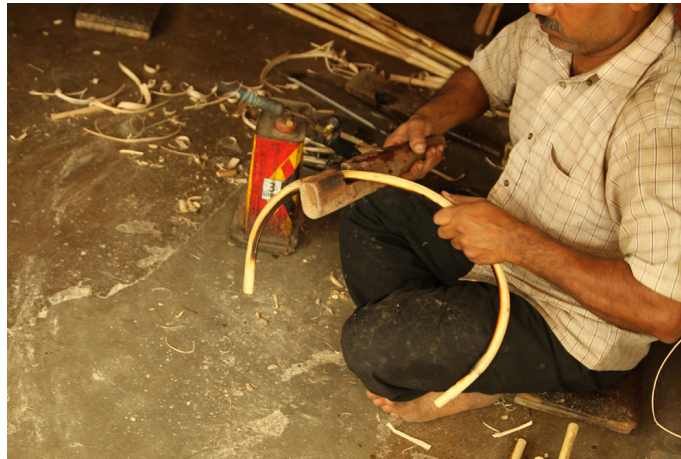
A wooden tool is used to bend the heated bamboo into required shape.
