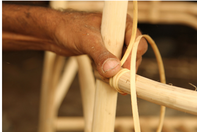
Thin strips are winded at the joints and edges for stiffness.
