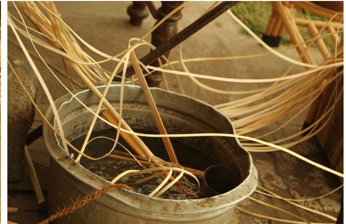
The bamboo strips are soaked in water for flexibility and avoid breakages while tying.
