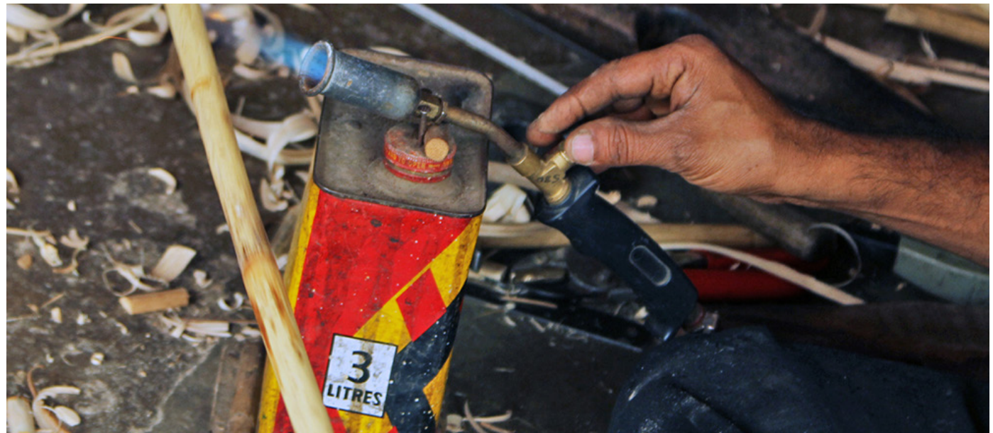
The bamboo sticks are heated for easy bent and flexibility.
