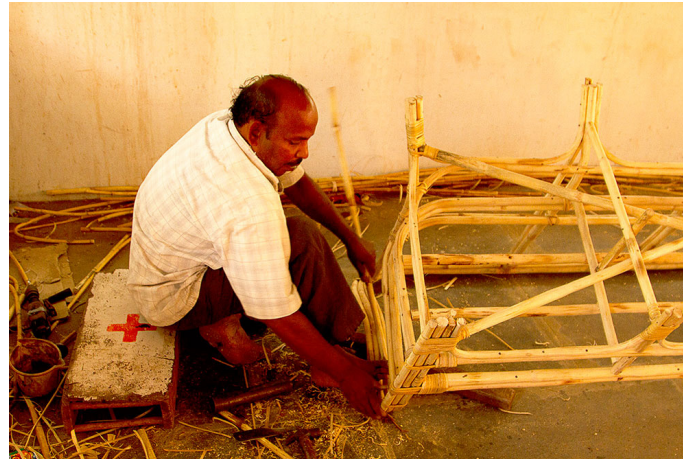
Basic structure of chair is build using various lengths of cane fasten to each other.
