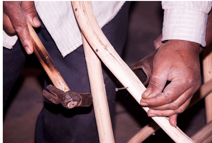
Quarter inch metal-nails also used as additional fasteners in the assembly.
