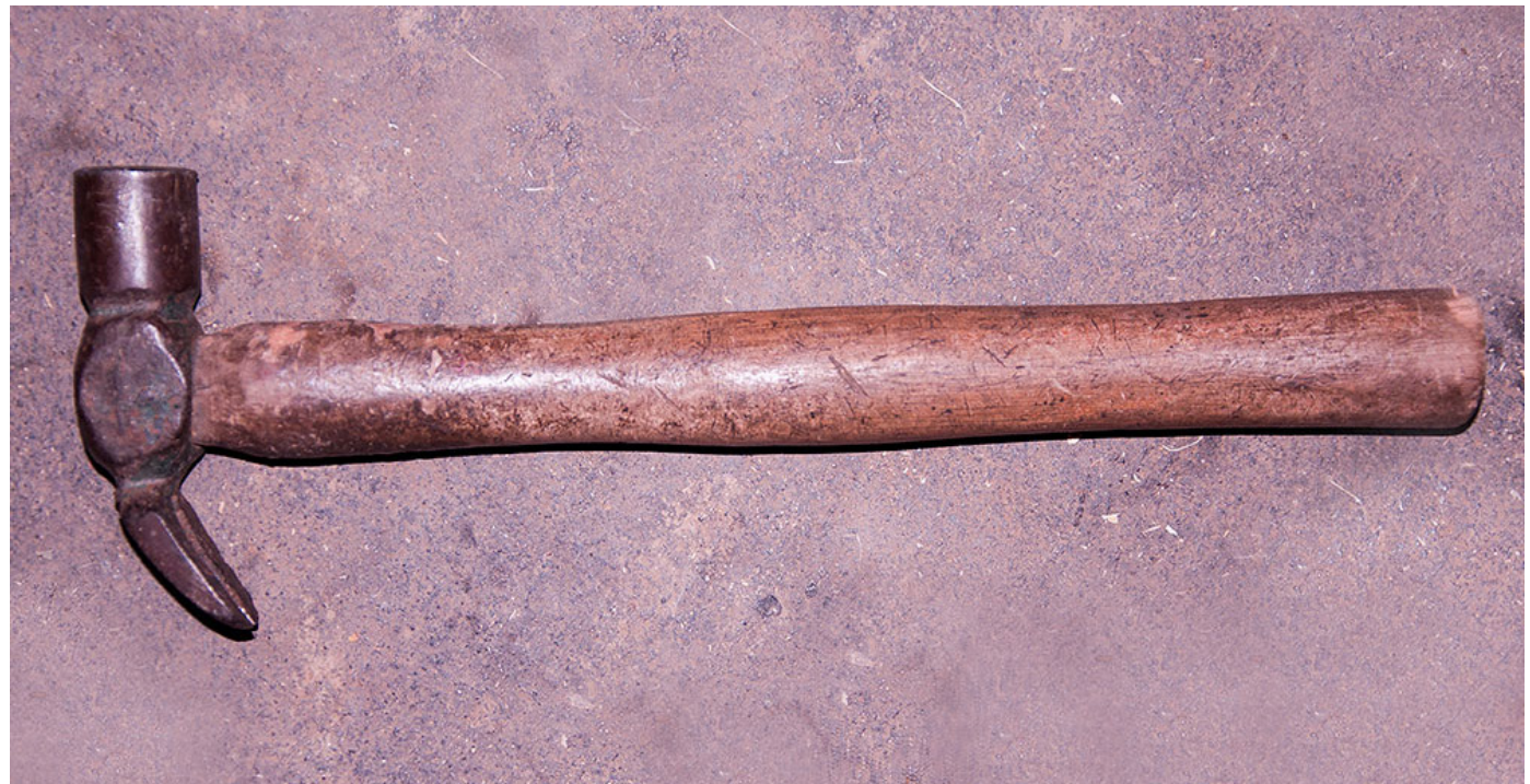
Claw hammer used for pounding nails into or extracting nails from cane pieces.
