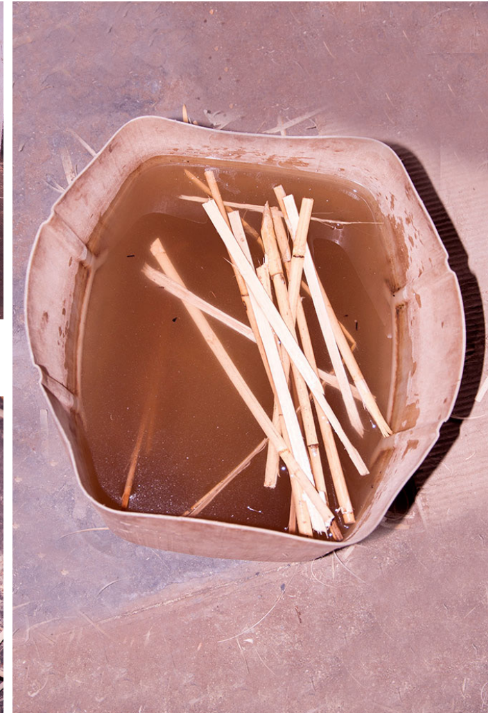
Sliced cane pieces are soaked in water to achieve the property of flexibility and softness.
