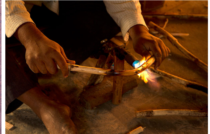
Flame torch is used to heat and bend cane when required.
