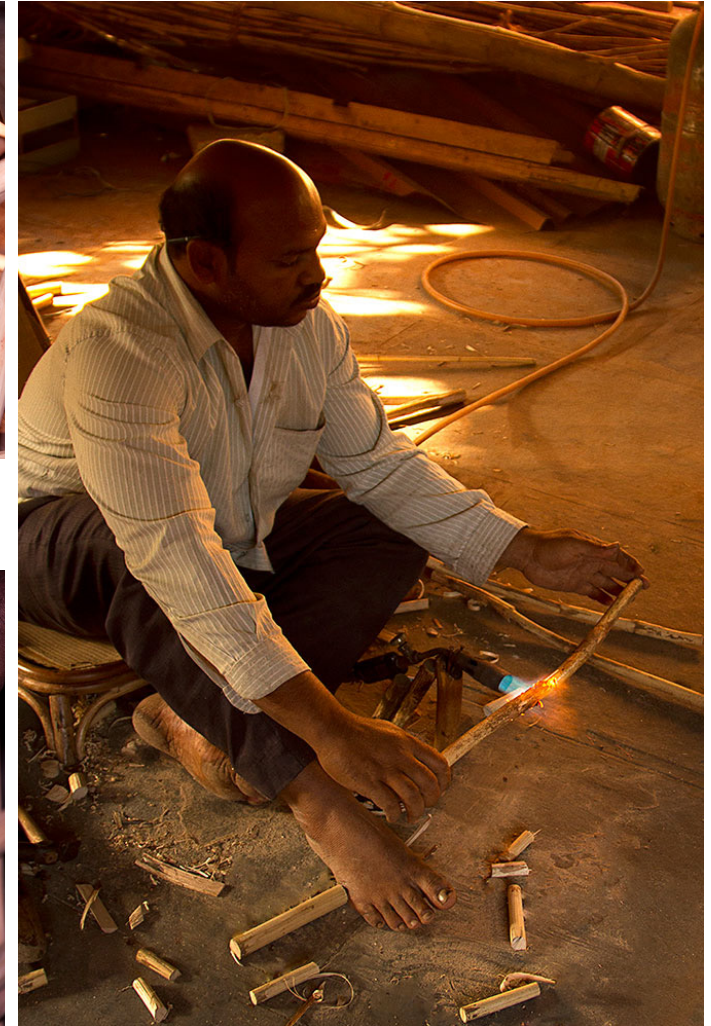
Generally flame torch is used for bending cane by heating the area.
