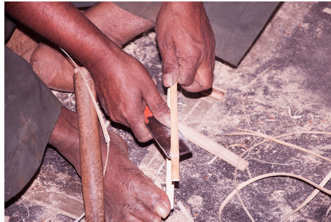
Slitting a the cane in symmetry which can be used in various motif.
