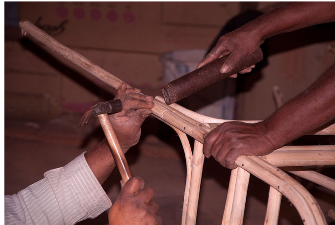
Generally half-an-inch metal nails are used to fasten cane with a support to avoid twisting.
