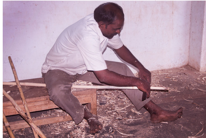
Skinning the raw cane using wide-blade to get a smooth finish.
