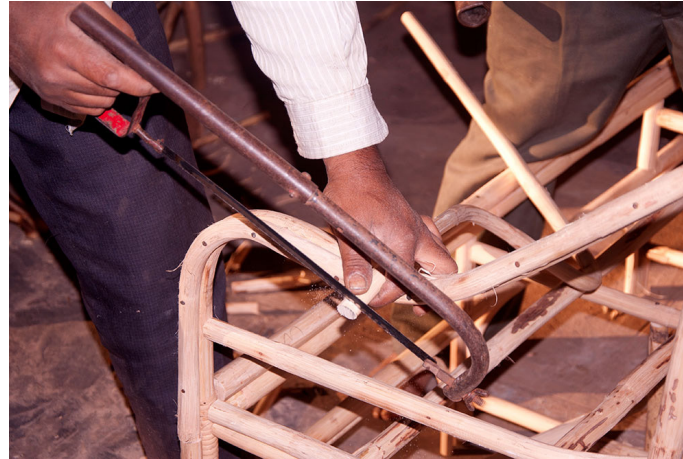
Hacksaw is used to cut the extra length.
