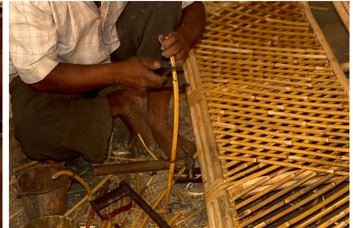
Young cane pieces are assembled in seating area and back rest after skinning.
