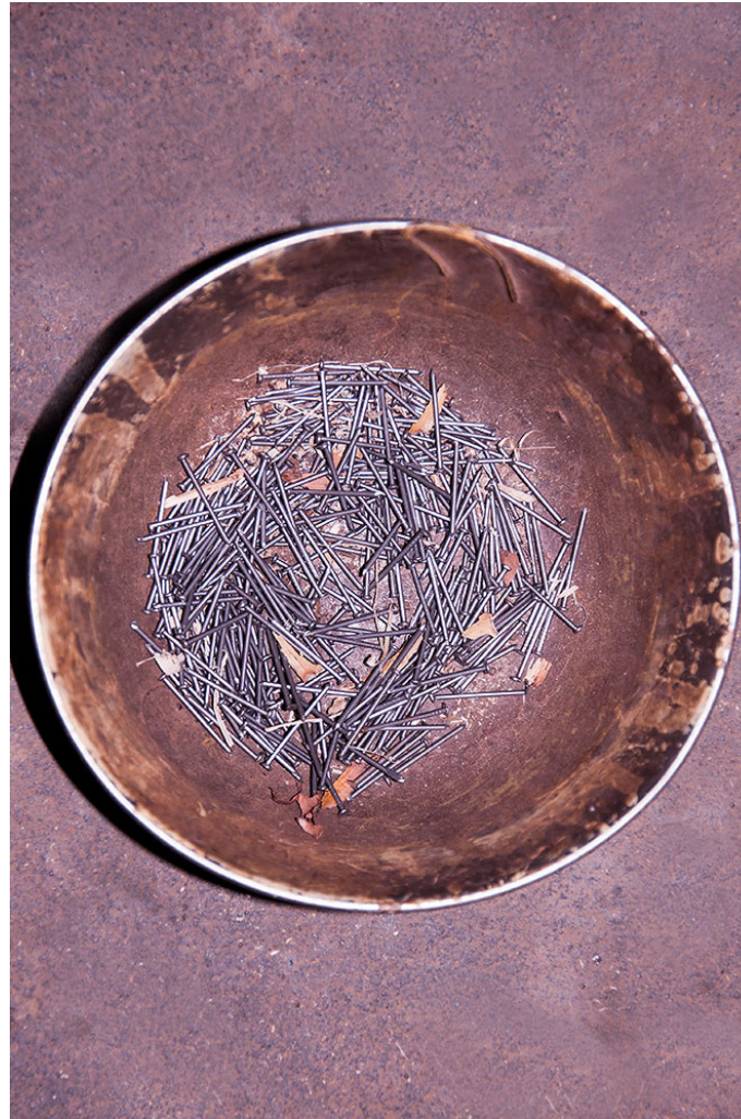
Metal nails of 1/4th, 1/2th and 3/4th size are used in assembling cane furniture.
