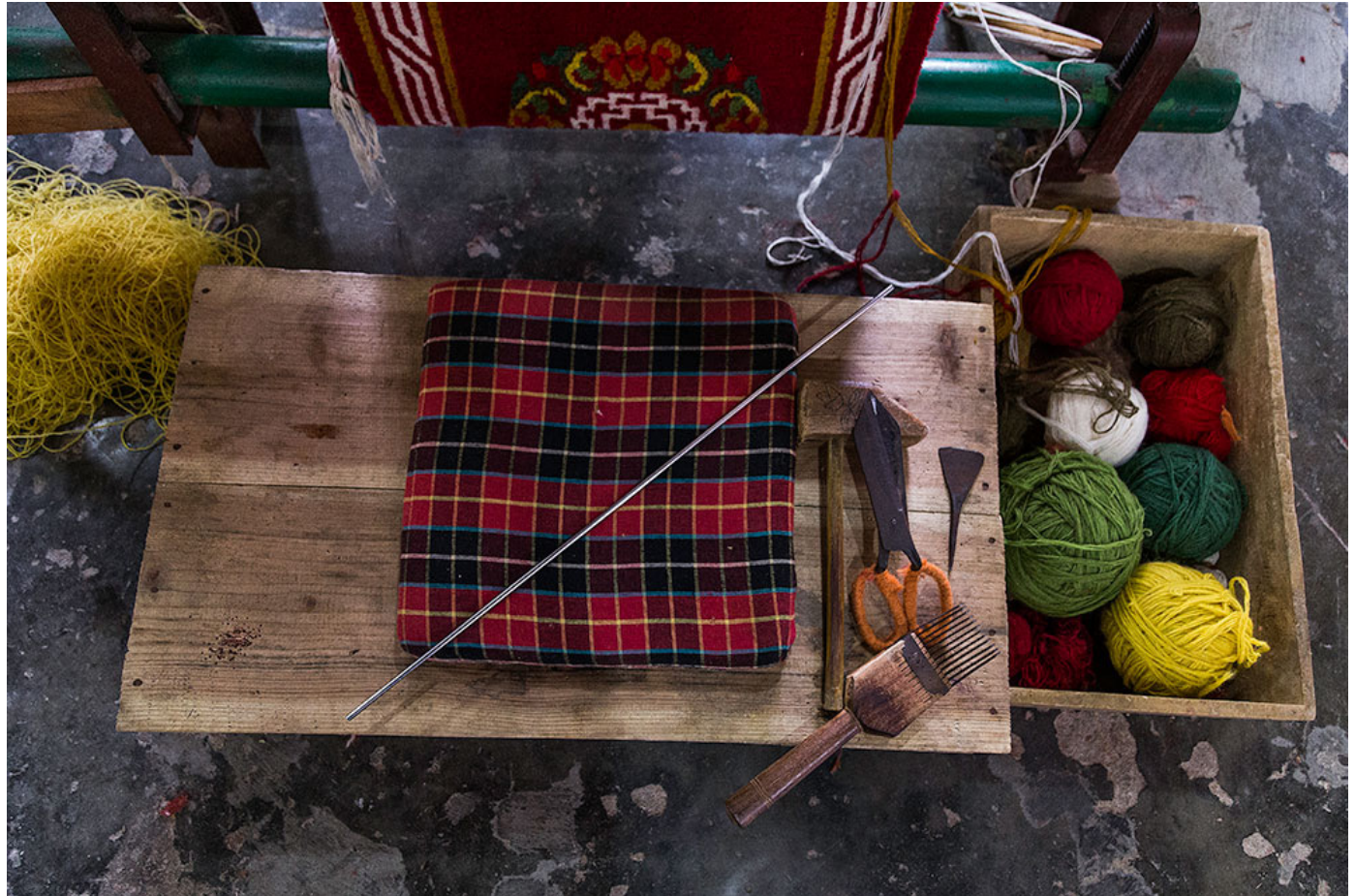
Tools used for weaving- wooden hammer to push the knots down, a special comb to separate the threads, a scissor to cut the extra threads.
