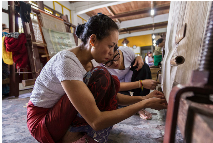
A skeleton of vertical threads is made known as warp or taan. It contains 101 threads for a width of 2 inch of carpet.
