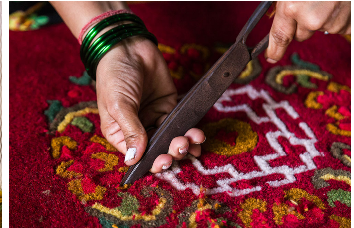
A special scissor is used to cut along the design giving it a 3D feel.
