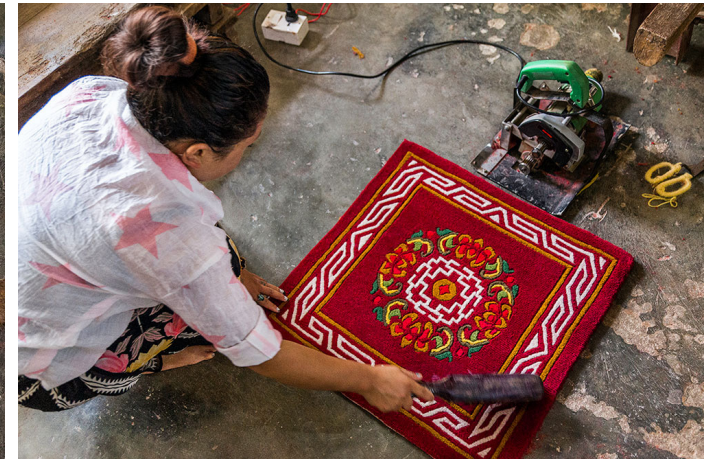
This brush is used in combination with the levelling machine to give finish to the carpet.
