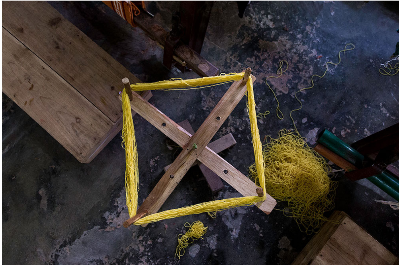
Wooden apparatus used to spin the loose wool known as phang.
