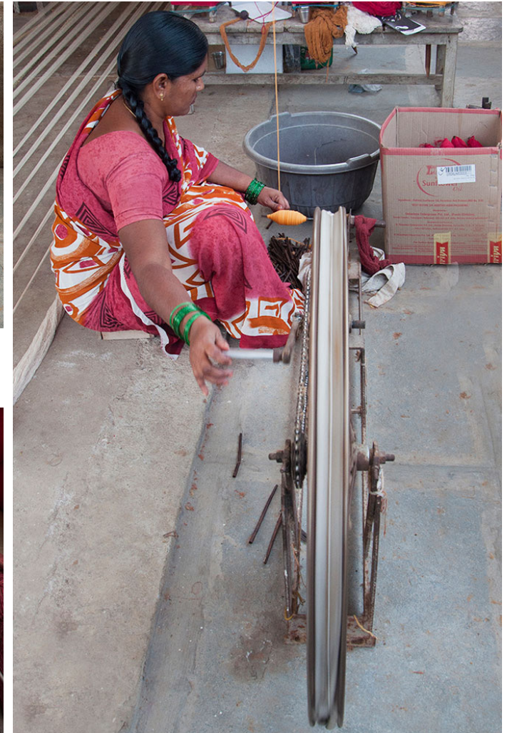
From the bamboo frame it is then transferred onto a pirn (small reel of thread, which goes into the shuttle).
