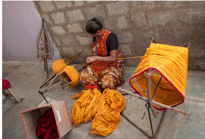
The dyed thread bundle, which is dried is put to a wheel where it is un - winded on to a bamboo frame.
