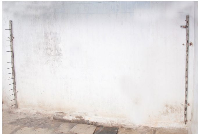
Image showing warping frame, framed onto a wall, where numerous thread are placed parallel to each other for vertical lines of thread to be placed on a loom's beam.
