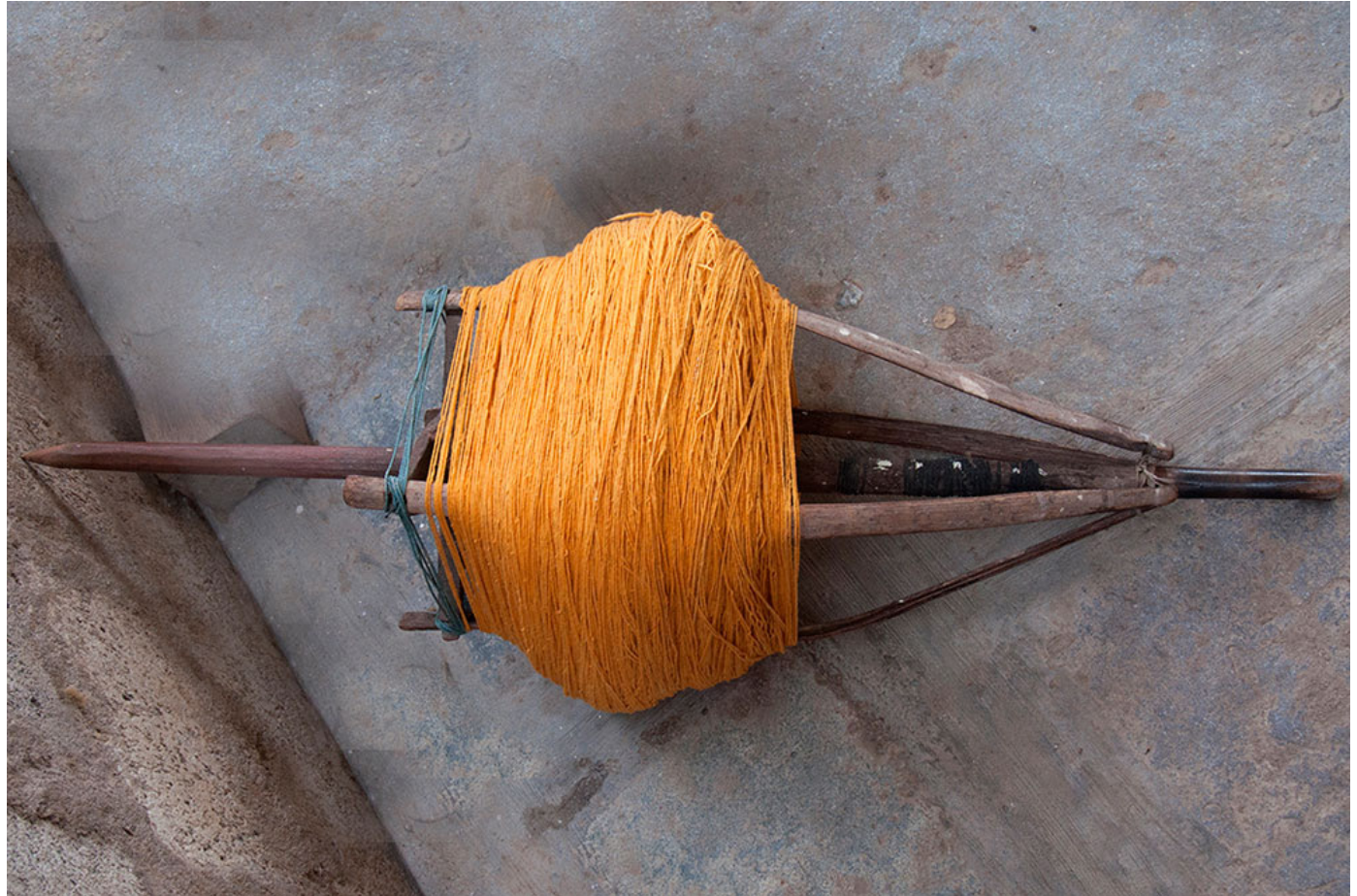
A bamboo frame onto which the bundles of threads are winded after dyeing.
