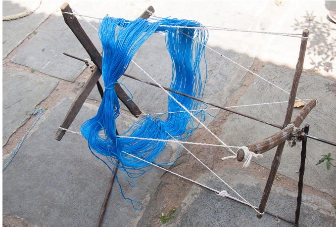
A wheel used in warping process, to unwind the thread bundles onto a bamboo frame.
