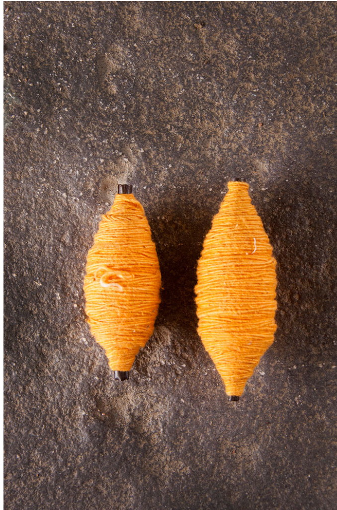
A pirn, which goes inside shuttle, used for horizontal weaving.
