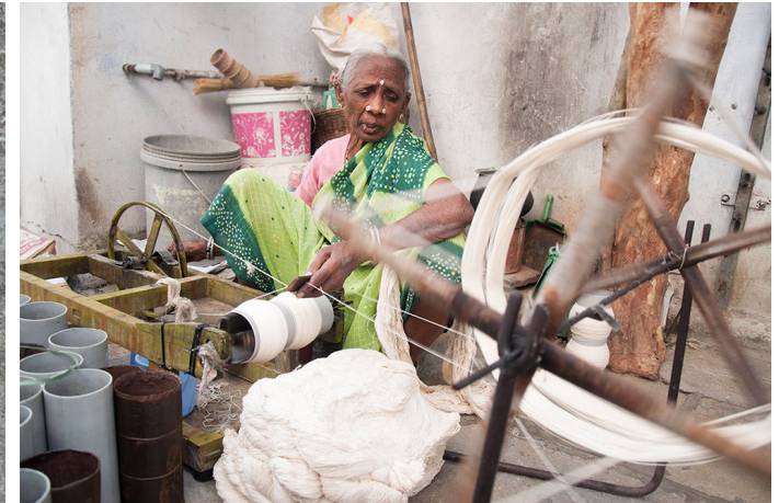
An artisan unwinding the thread bundle on a plastic pipe to make warping process.
