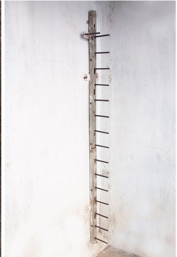
Warping beam used to make vertical bundle of thread lines, parallel to each other.
