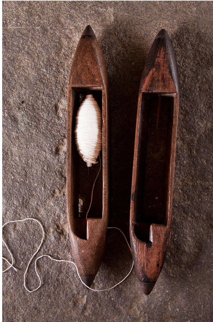
Large sized shuttles used In horizontal weaving, in which pirns (thread reels) are loaded.
