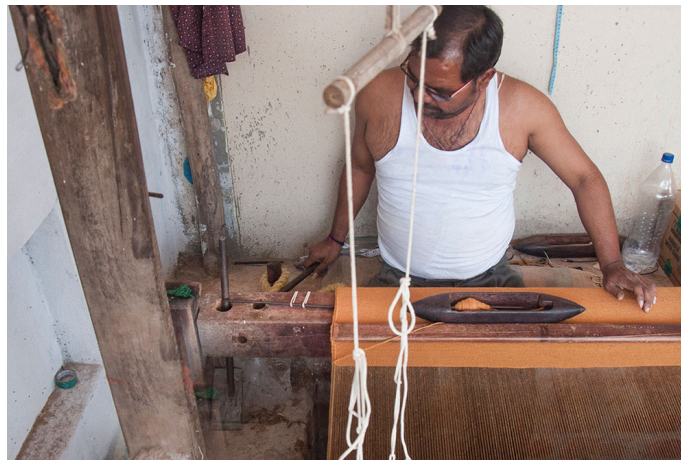
Artisan rolls the cloth as it is finished inch by inch with the help of a steel rod.
