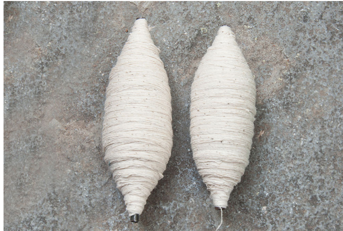
A typical pirn reels which goes into the shuttle, which helps in horizontal weaving.
