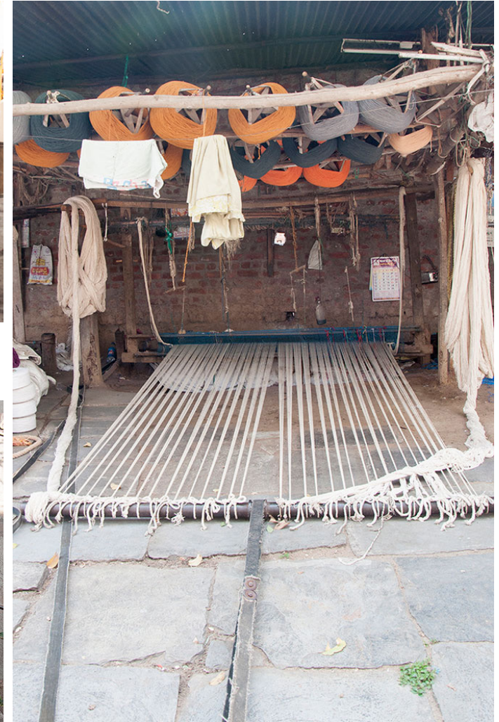
A typical pit loom used for weaving, by the artisans.
