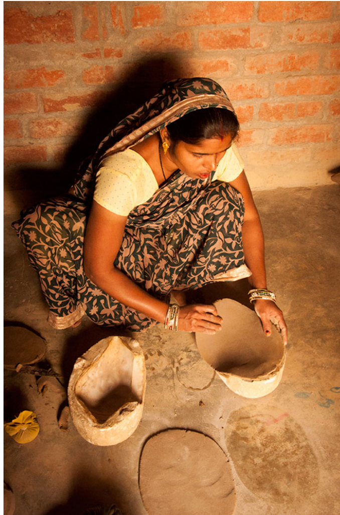
Placing clay inside the mold.
