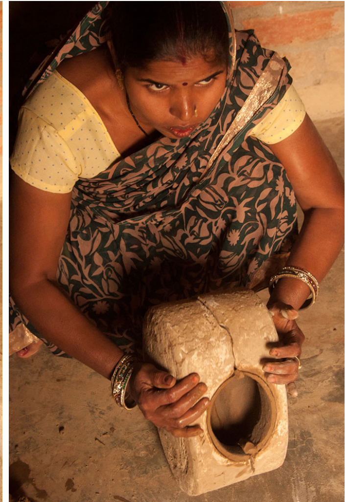
Both the molds are joined together to get a 3D clay model.
