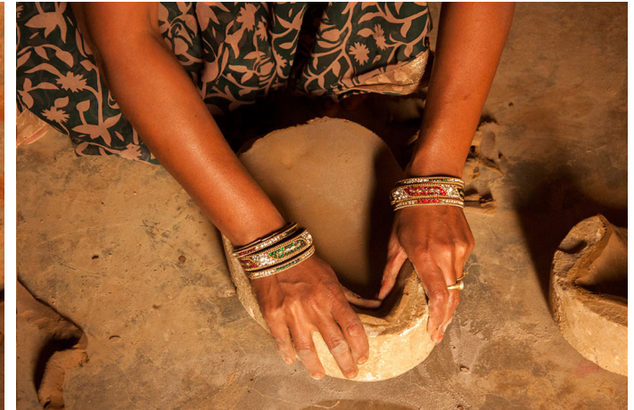
Pressing the clay to get the impression of design in mold.
