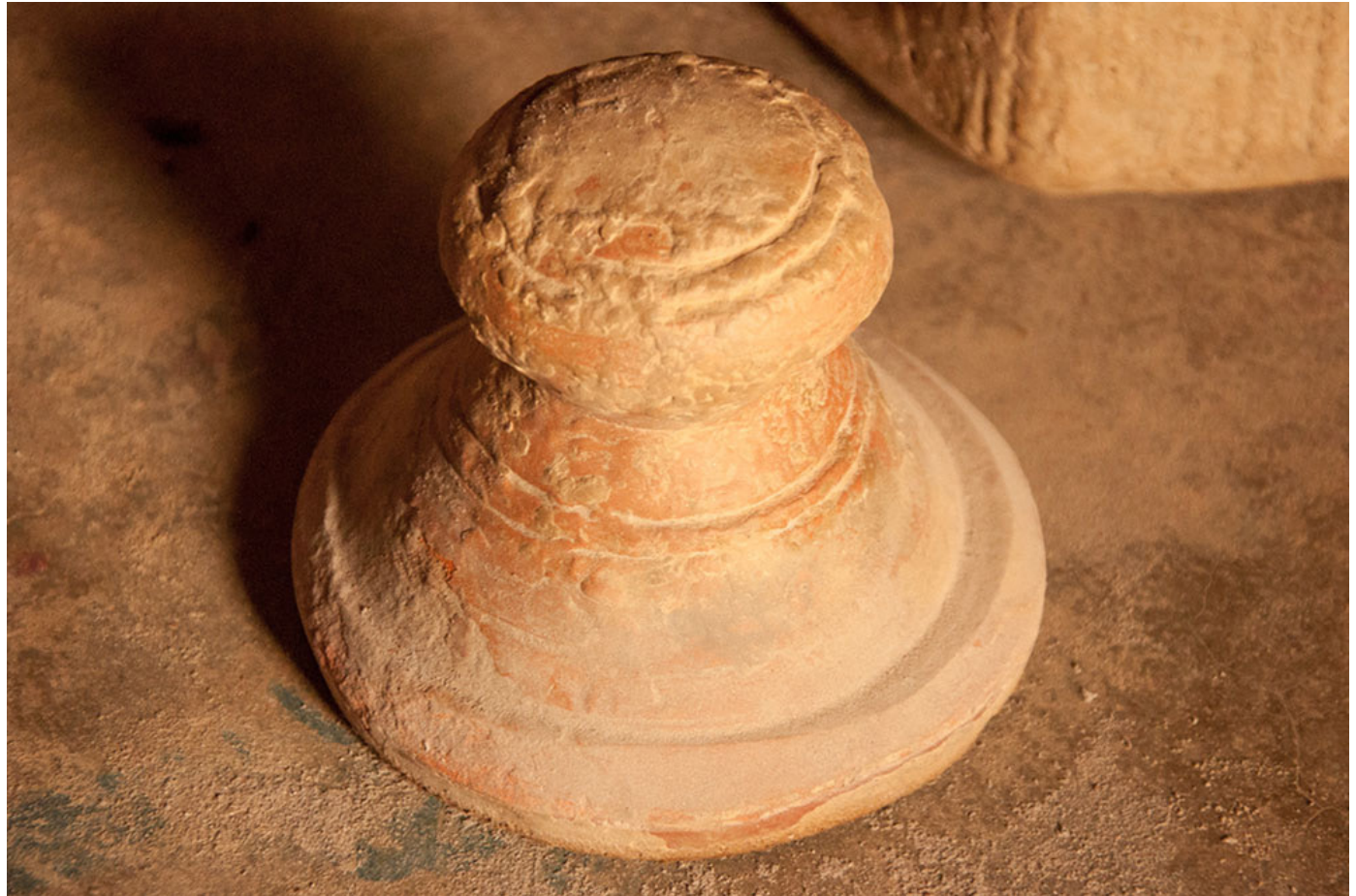
Mold used to level the clay.
