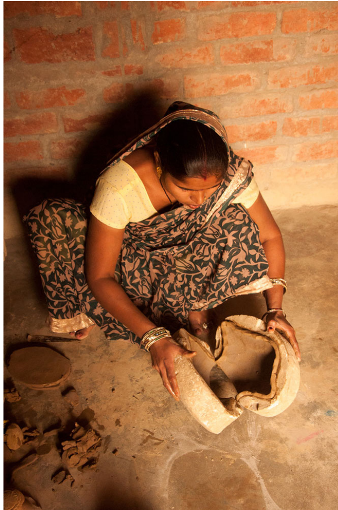
After placing the clay inside mold, mold is being closed.
