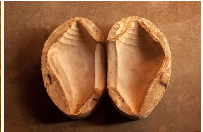
Plaster of Paris mold is used to make money box.
