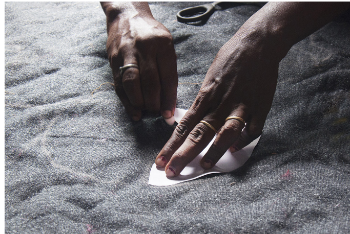
Marking on the fur using a paper cutout.
