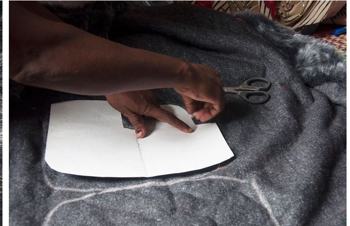
Marking edges along the cutout with a chalk.
