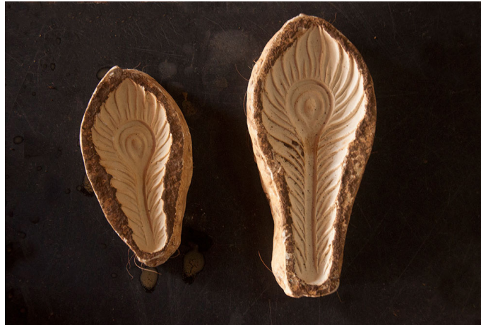
A view of mould made of Plaster of Paris.
