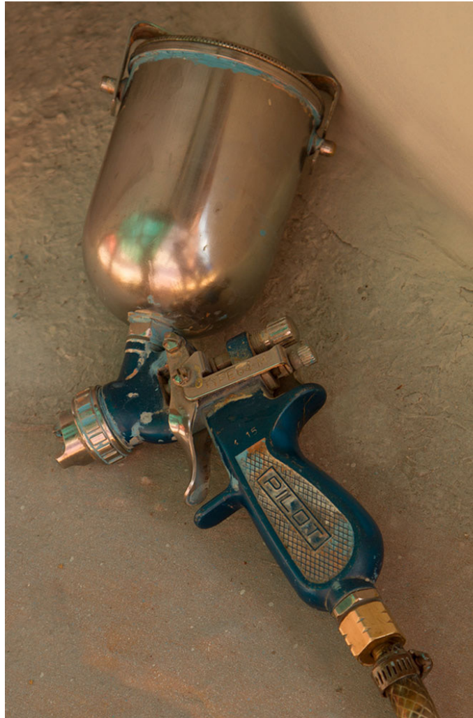
Paint spray gun is used to spray paint evenly.
