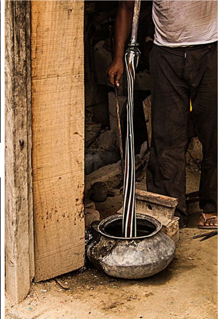
Molten glass is being dipped in water.
