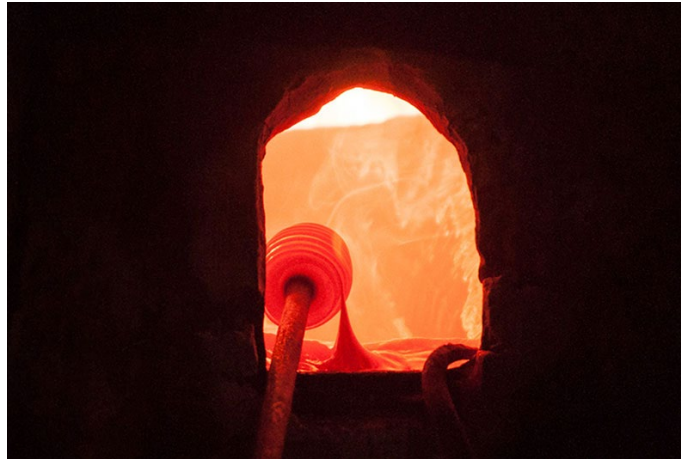
Molten glass collected on iron rod.
