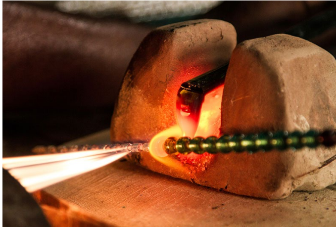
Torch process where the glass meets the metal to form a bead.
