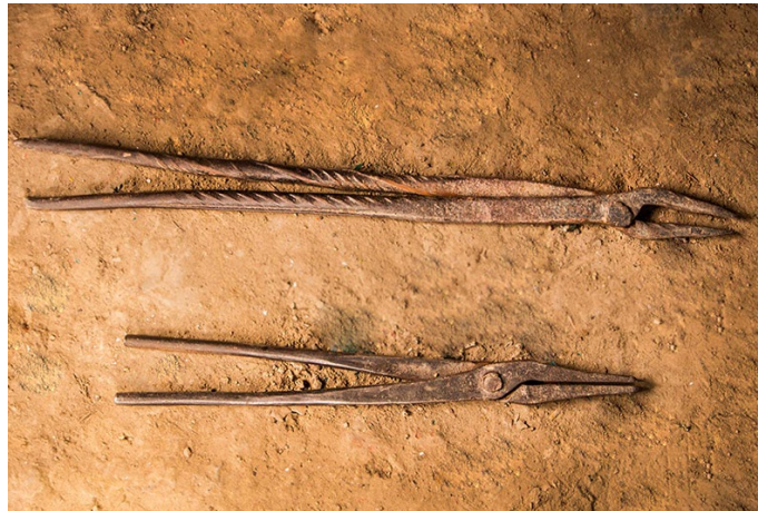
Holders known as chimta are used to pull the molten glass.
