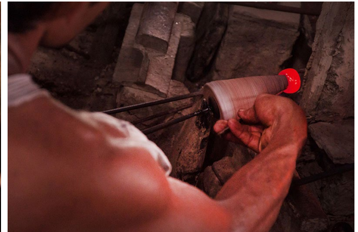
Molten glass taking the shape of a bangle.
