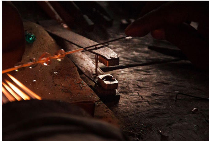
Various designed molds are used to shape the beads.
