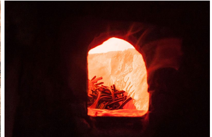
Glass pieces are kept inside the furnace to obtain molten state.
