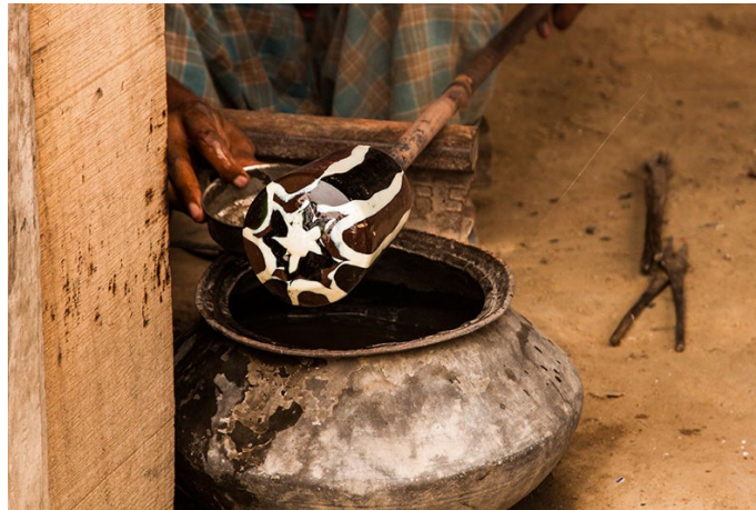
Homogeneous glob is cooled using normal water.
