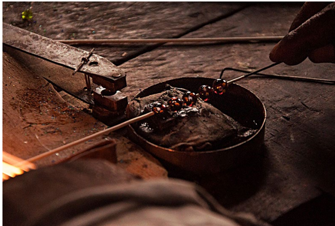
Bead is first dipped in ghee for lubrication.
