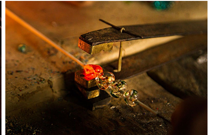
Heart shaped mold pressed on the bead.
