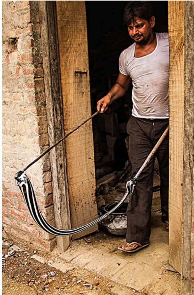
Craftsmen holds two ends of the molten glass.
