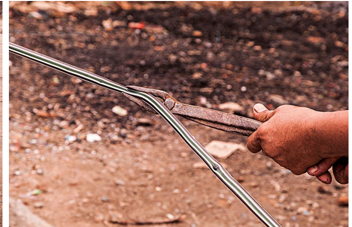
Plier is used to hold the stretched glass.
