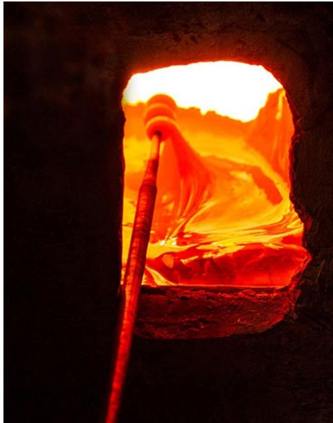
Molten glass is looped on iron stick.
