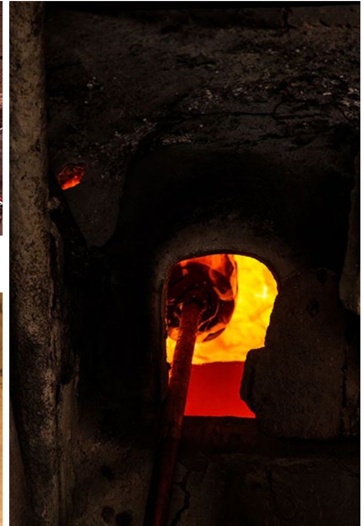
Glob is reheated again in the furnace.
