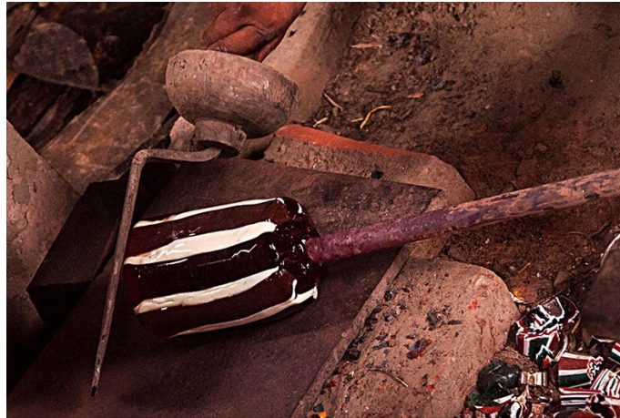
A trowel is used to create a continuous millefiori surface with constant pressure.
