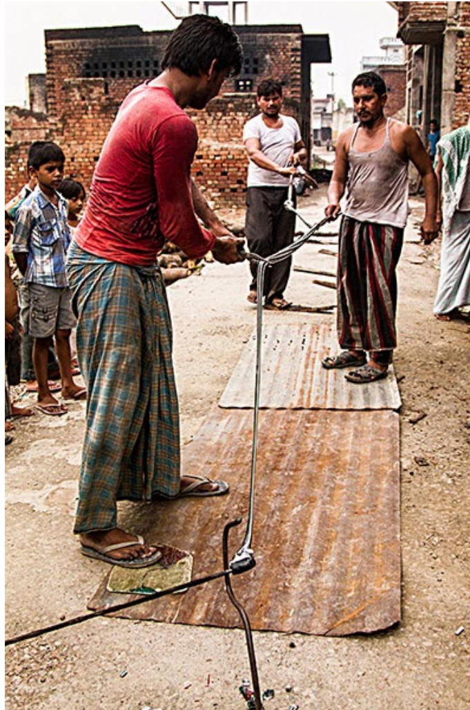
The other end is stretched uniformly by two/three craftsmen in Synchronization.
