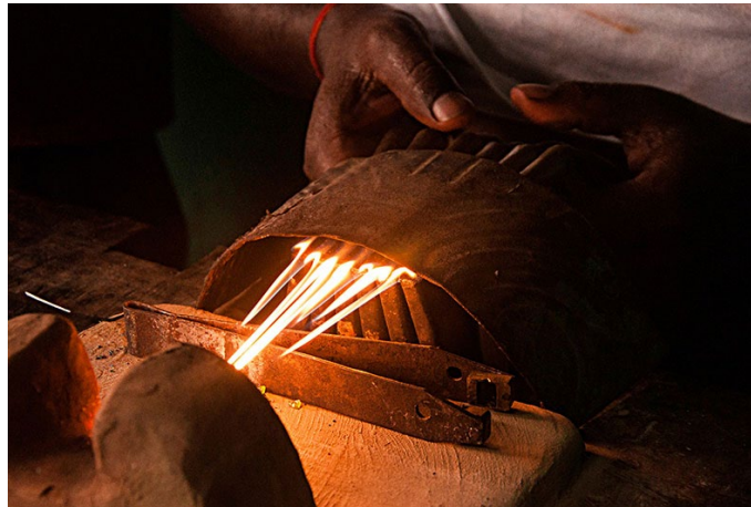
Flame which is directed are also controlled by a pedal below.
