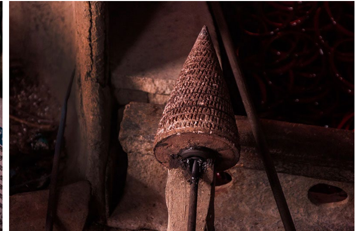
Khalboot is tool used to shape the different sizes of bangle.
