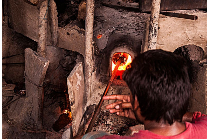
Artisan skillfully collecting the molten glass on the rod.
