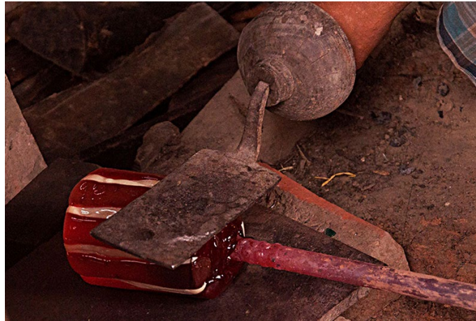
Reheated glass is again pressed with a trowel.
