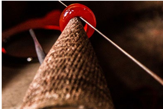
Molten glass is transferred to the khalboot.
