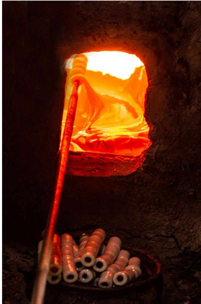
Another coat of molten glass is looped on the silver leaf covered beads.
