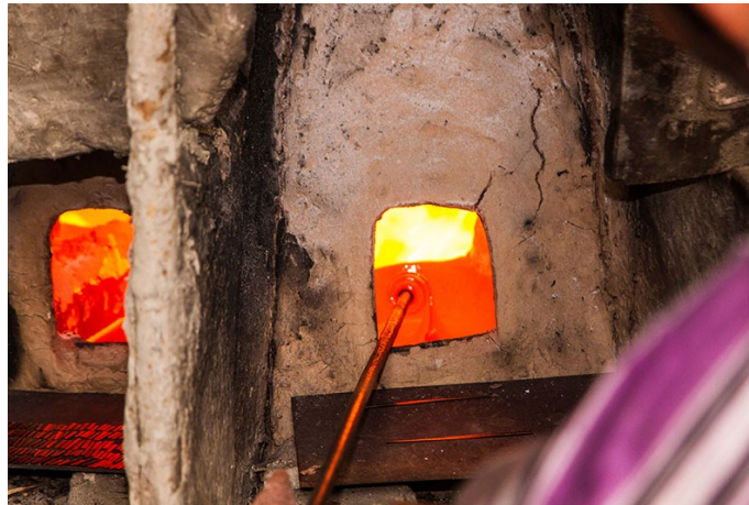
Molten glass is looped on the iron rod.
