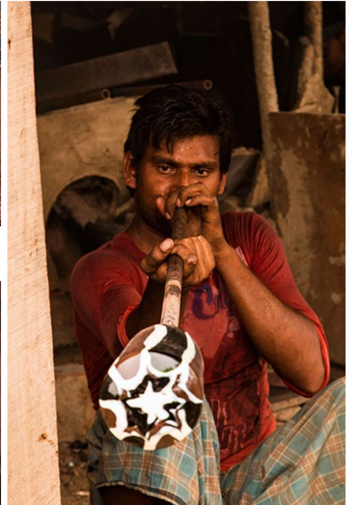
Metal rod is blown to increase the stiffness of the molten glass on the other end.
