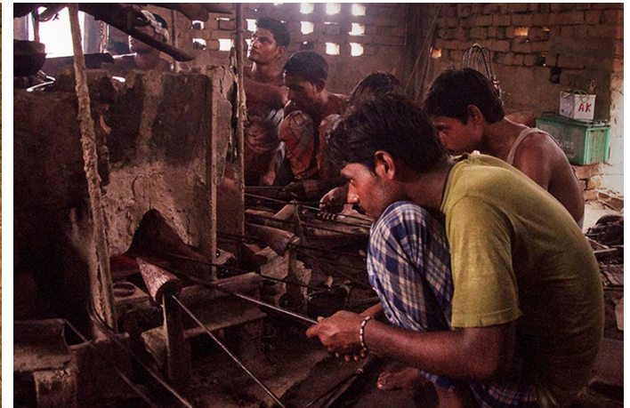
Open furnace is used to melt the molten glass.
