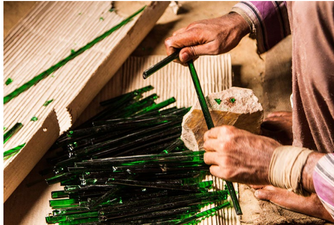
Artisan is manually breaking the glass rods.
