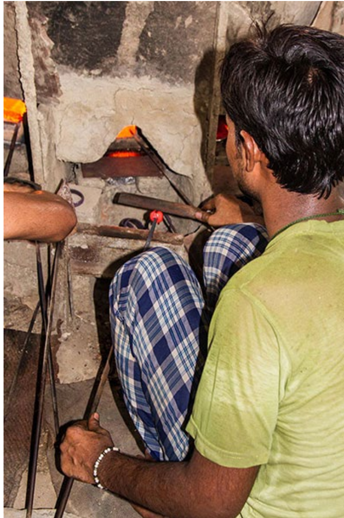
Bangle is pressed giving uniform elasticity.
