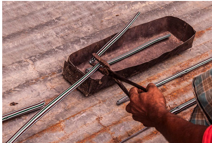
After the glass is cooled down, it is then broken into smaller pieces.
