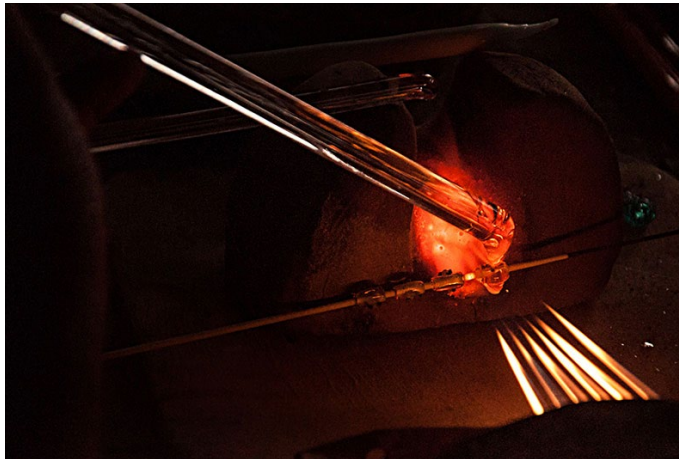
Glass bead taking the form a heart shape through the mold.
