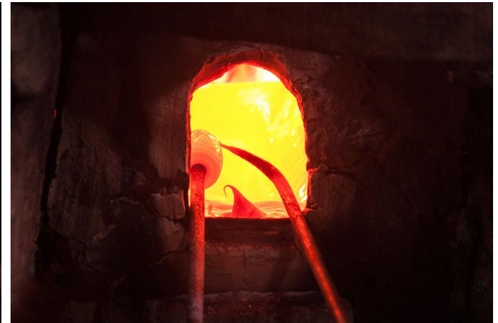
A long iron rod (sariya) is used to loop the molten glass.
