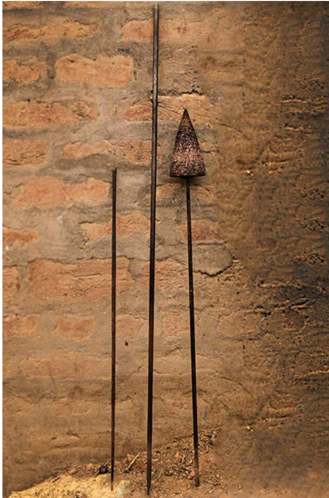
Sariya and khalboot are the main tools used in glass work.
