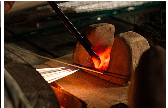
Glass rod is melted to form a coil along the metal wire.
