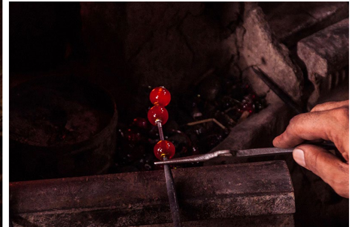
Shaped beads are removed carefully, avoiding breakages.
