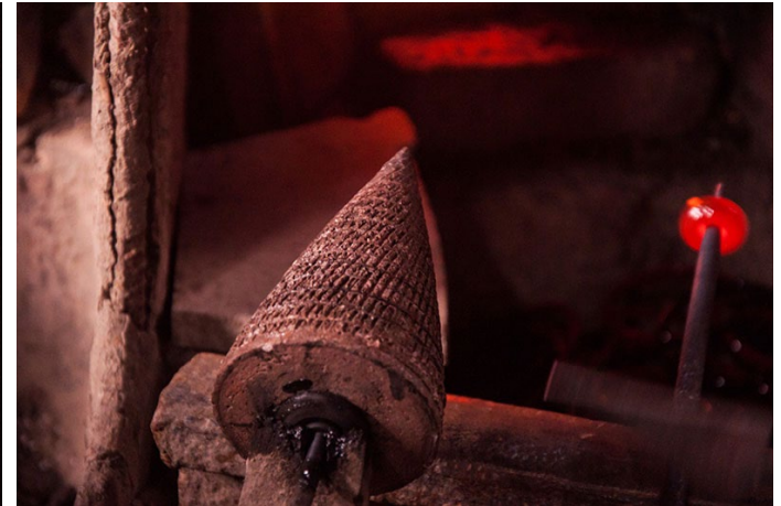
A conical spinning wheel (khalboot) which consists of different grooves.
