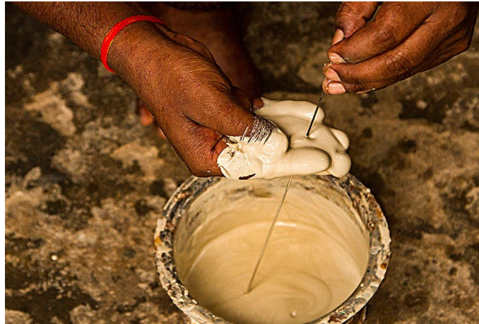
Clay is applied on the metal wire.
