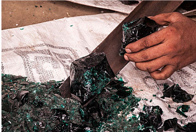
A metal sheet is used to add chunks of glass into the furnace.
