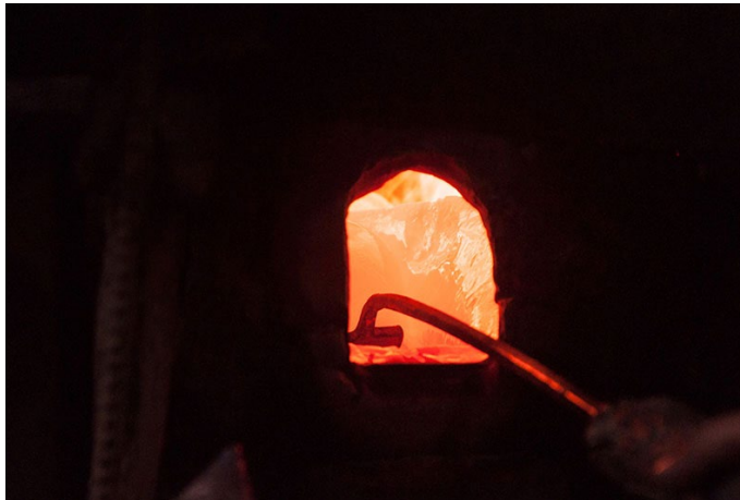
Craftsmen making sure that all the raw materials in the furnace (bhatti) are melted.
