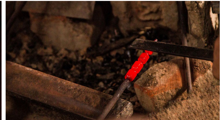
The beads are shaped in cylindrical form.
