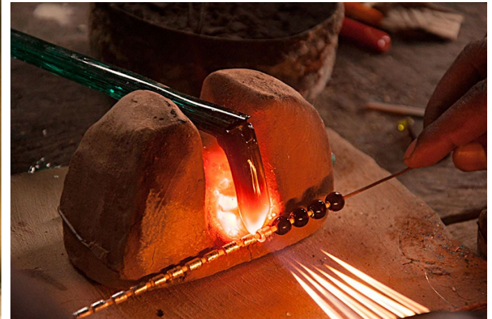
Molten glass is looped and taking a shape of a bead.
