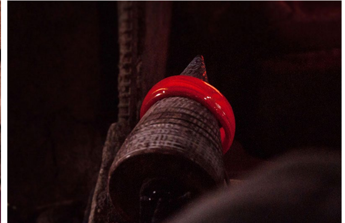
Bangles are pushed on khalboot, depending on the required size.
