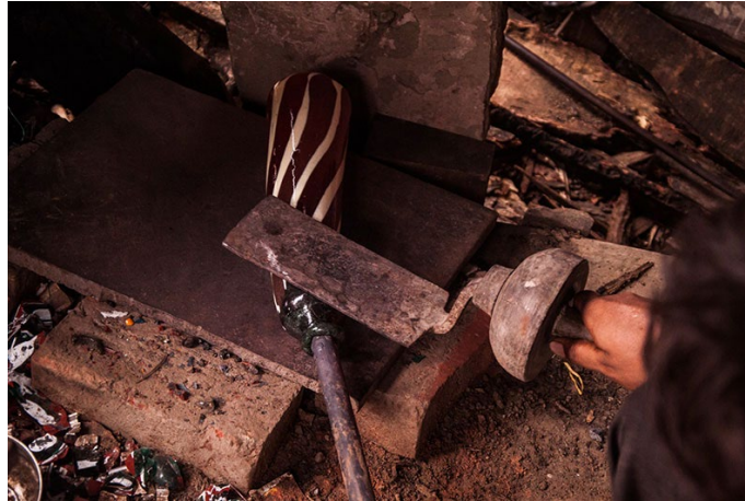
Artisan shapes the molten glob into a cylindrical form.
