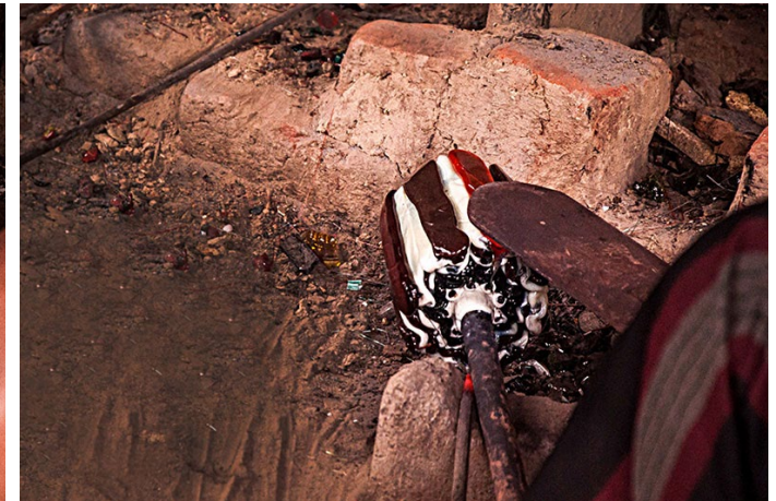
Another layer of paste of different color is applied.
