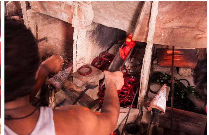
Chunk glass is fed into the furnace.
