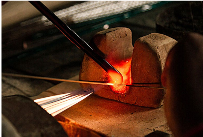
Molten glass being looped.
