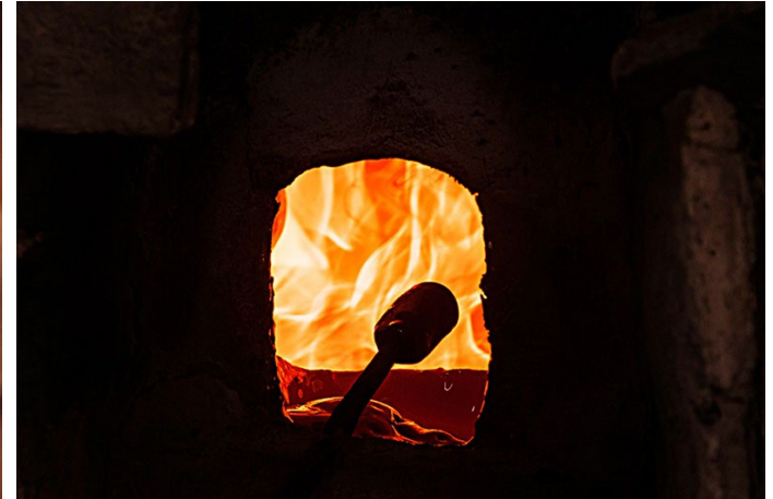
A glob of molten glass is collected on a metal rod.
