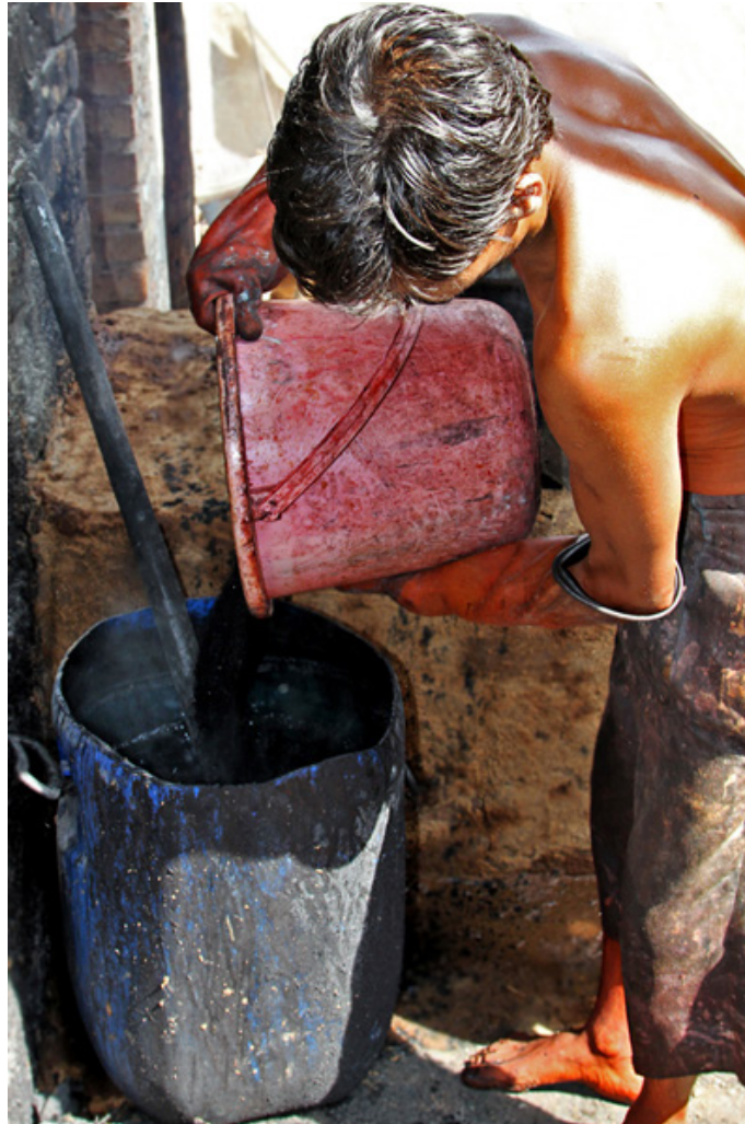
Dye powder is added to the hot water to make a thick solution.
