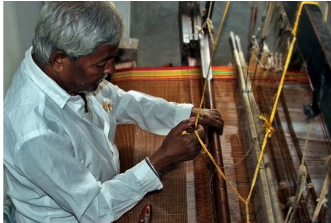
After the thread is positioned, the flying shuttle is again pushed through the yarn.
