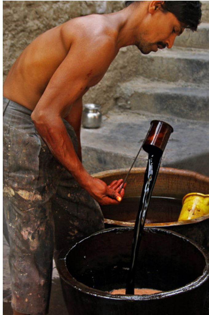
Liquid dye is mixed with water to form a thick solution.
