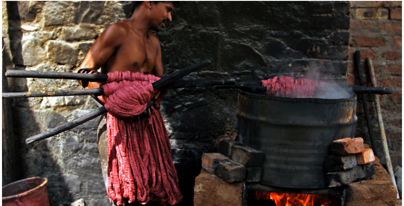
The already dyed yarns are dipped into the large vessel with the help of a bamboo.
