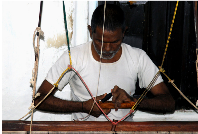
Loaded pirn is inserted into the flying shuttle.
