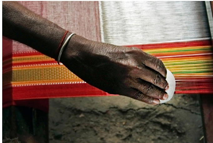
Artisan applying wax to the unweave yarn for smoothing the weaving process.
