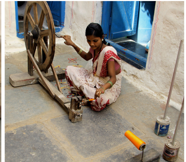
Artisan loading the pirns with silk thread with the help of the Charkha.
