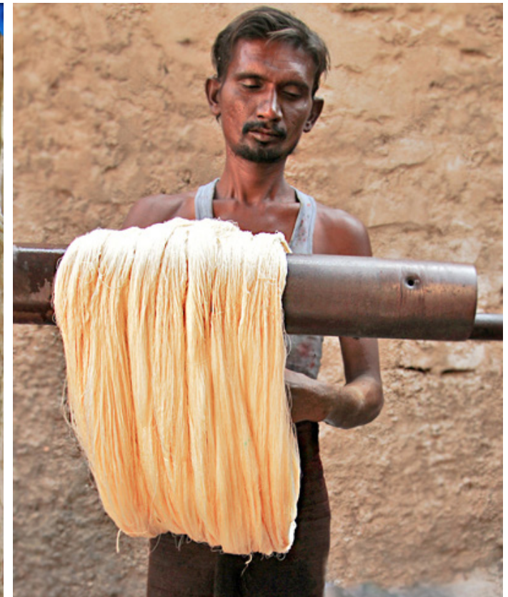
Each bundle is separated and suspended on an iron rod to ensure the threads.
