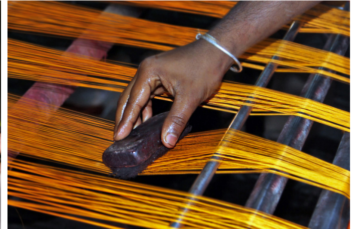
With the help of the brush each thread is separated for the dyeing process.
