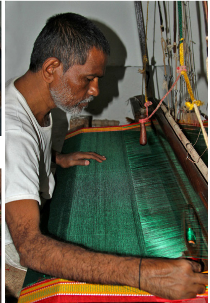
Flying shuttle loaded with pirn is inserted into the divided yarns to weave them.
