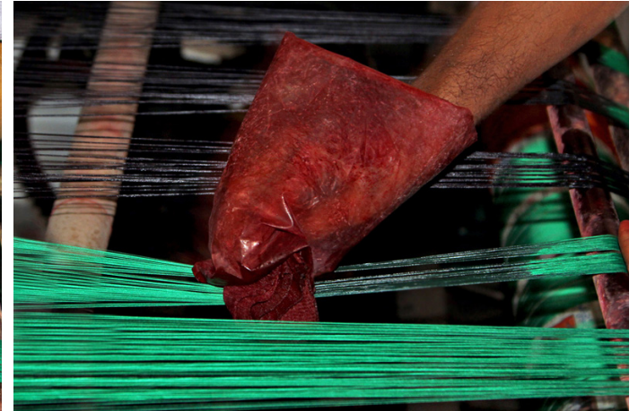
Dye is applied to the yarns with the cloth.
