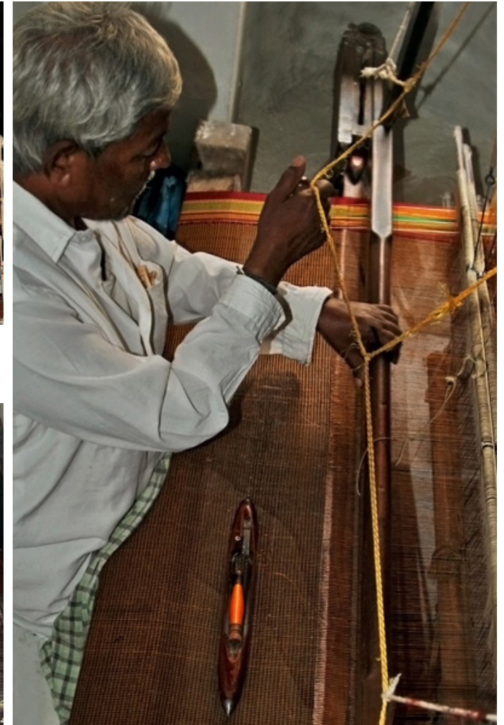
To position the silk thread in place the heddle shaft of the loom is used.
