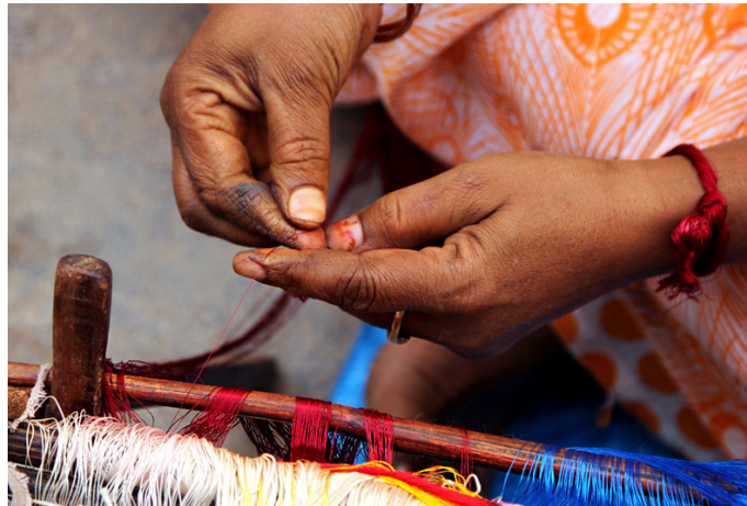
With the help of wood ash and natural gum the threads are linked with one another.
