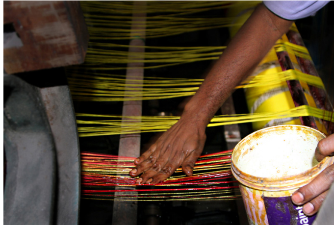
Water is applied to the unweave yarns attached on the loom.
