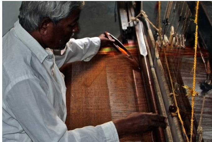
The flying shuttle is then passed through the divided part of the yarns to interweave and create a pattern.
