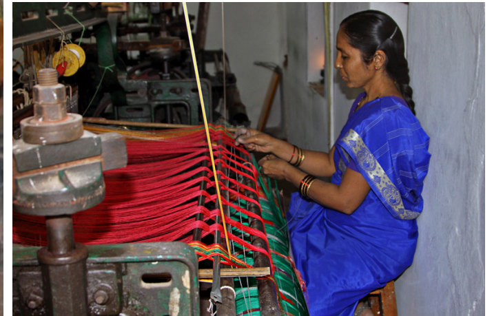
The warped yarns are being set on to the Power loom for the weaving.
