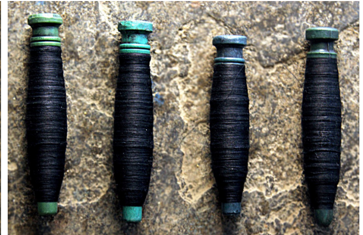
Pirns spun with black silk thread for the weaving process.
