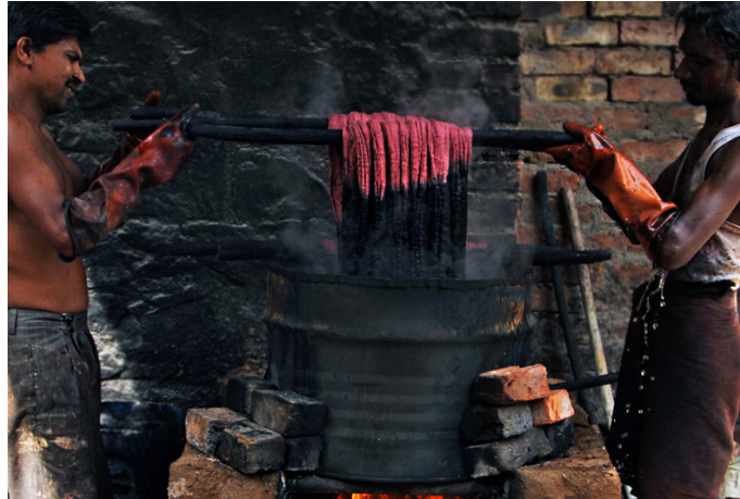
Two workers with the help of a bamboo turns the yarns to dip them fully into the solution.
