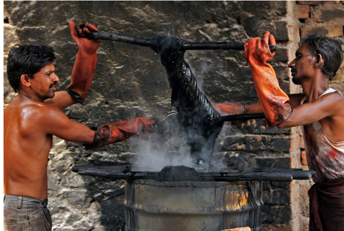
The coloured yarn is then twisted with the help of a rod to squeeze out the excess water.
