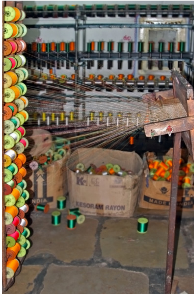
Metallic frames (creels) holds the bobbins through which the threads are passed on to the warping machine.
