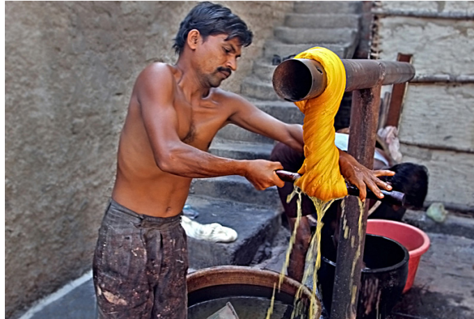
The excess of solution is squeezed out from the dyed yarn using a rod.
