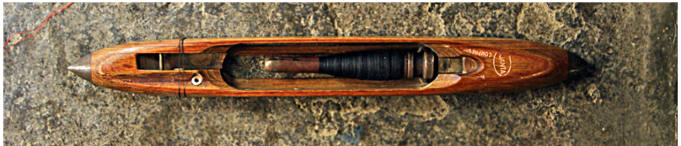
Flying shuttle loaded with pirns.
