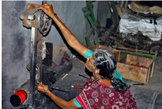
Spindle is fixed to a machine to start the winding process.
