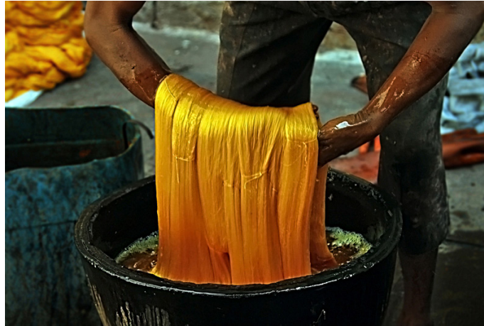
The white yarn changes into yellow and is pulled out of the solution.
