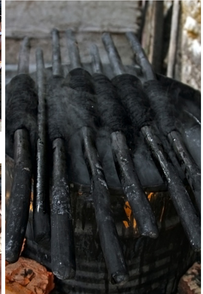
The dyed yarns are kept in the boiling solution to absorb the colours.
