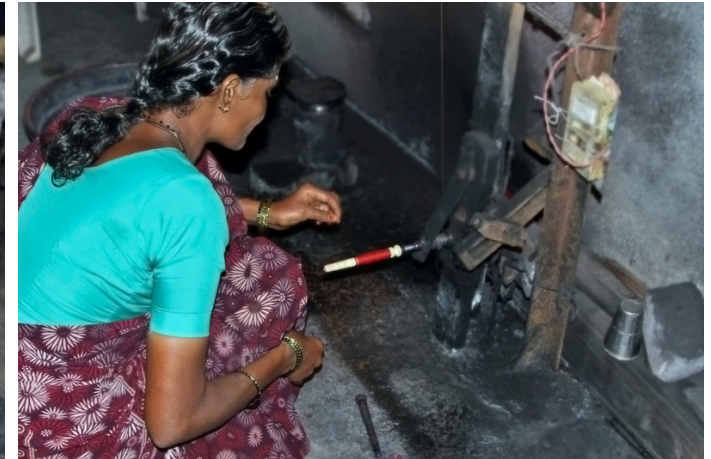
Then the pirns are spun from the spindles.
