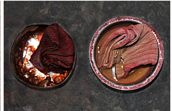
Cloth used to apply dye colours to threads attached to the loom.
