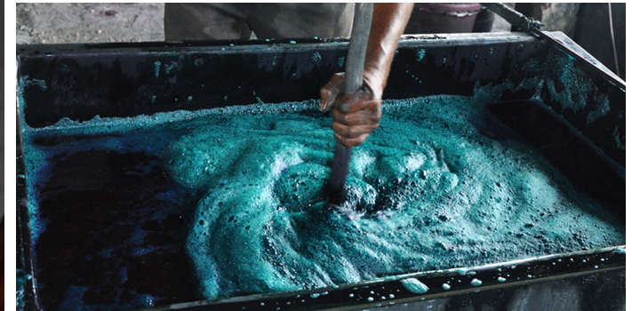
Color solutions are mixed well for even coloration to the yarn.
