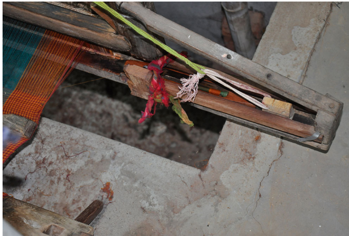
Fly shuttle with wound pirns are loaded to the sley of the loom for the weft insertion.
