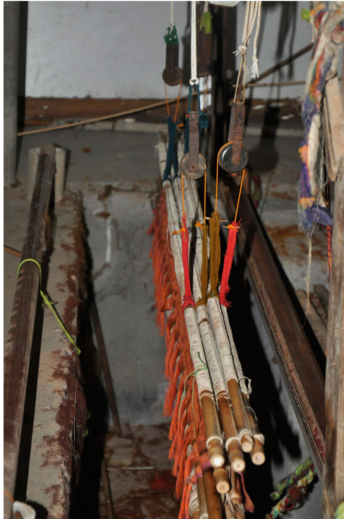
Pulleys and heddles of the loom help in the easier weaving of these saree.
