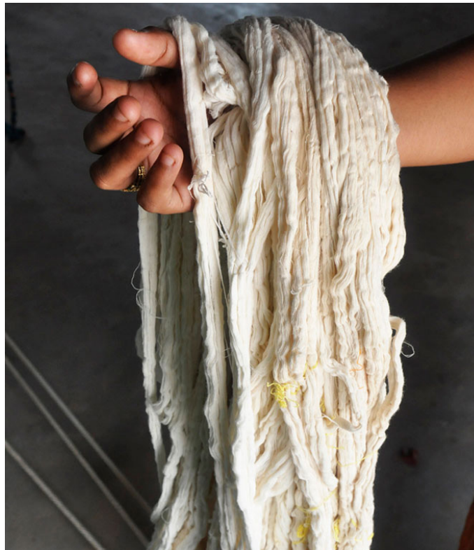
Cotton yarns are starched before coloring for strength purpose.
