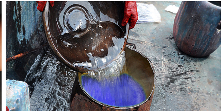
Dye is mixed with hydro sulphate and caustic soda.
