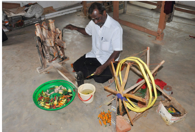
Charaka equipment is used to wind the cotton yarns from hank to the pirn.
