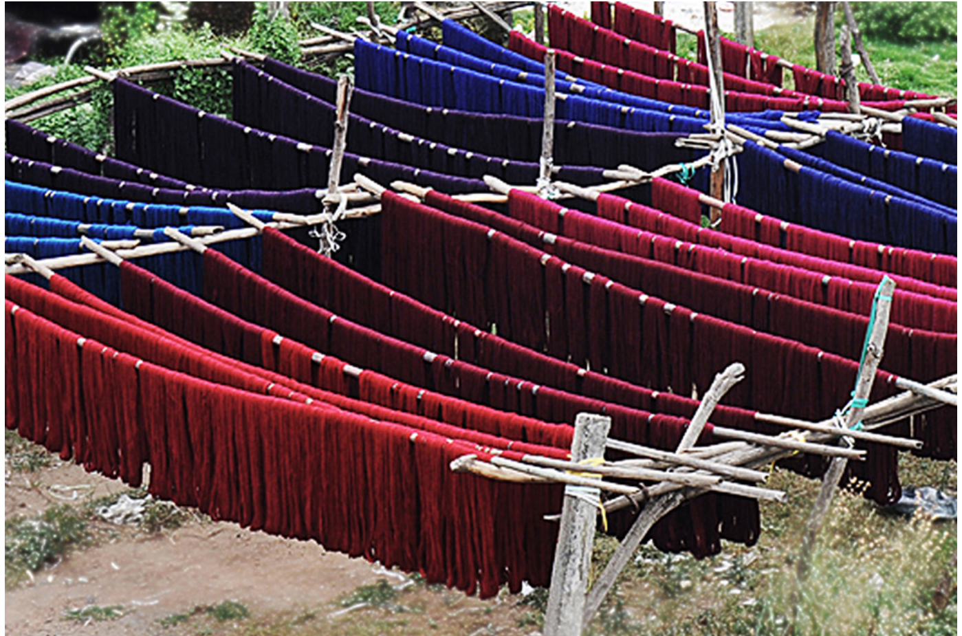
The dyed cotton yarns are dried under sunlight.
