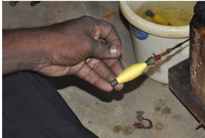
Yarns are wound on a plastic pirn evenly to avoid the breakages while weaving.
