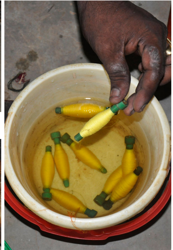
The wound pirns are soaked in water for minimum of 30 minutes before weft insertion.
