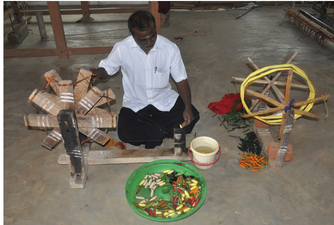
Yarns are wound to the pirns with the help of charkha.
