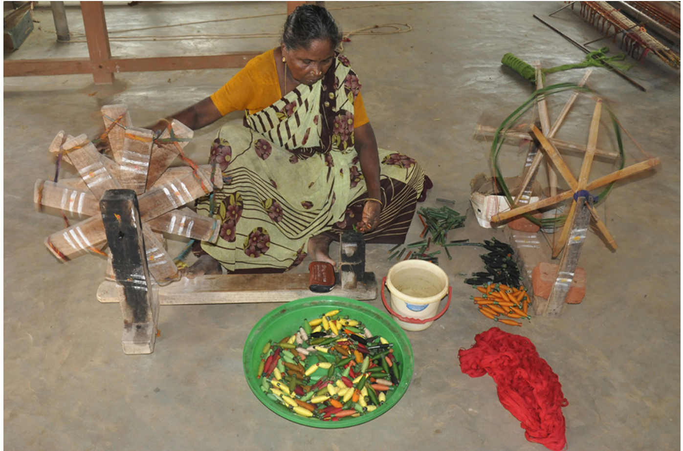
Charkha wheels are used to wind the yarns to pirns.
