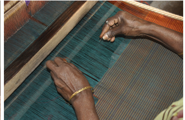
Safety pins are used to pull out the wrong yarns insertion out.
