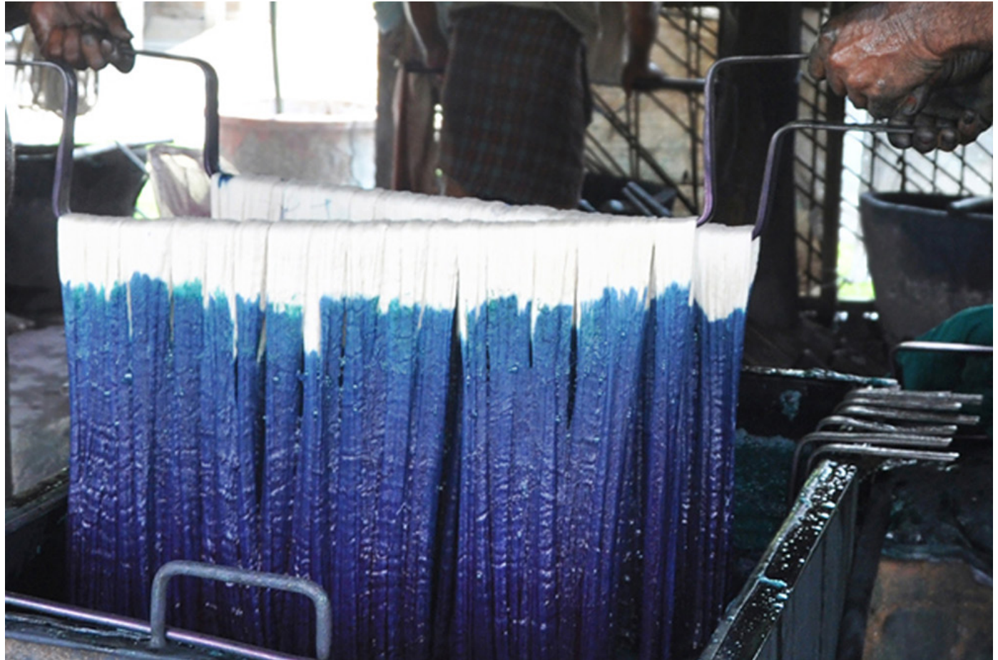
Cotton yarns are soaked in the dye solution heated to high temperature.
