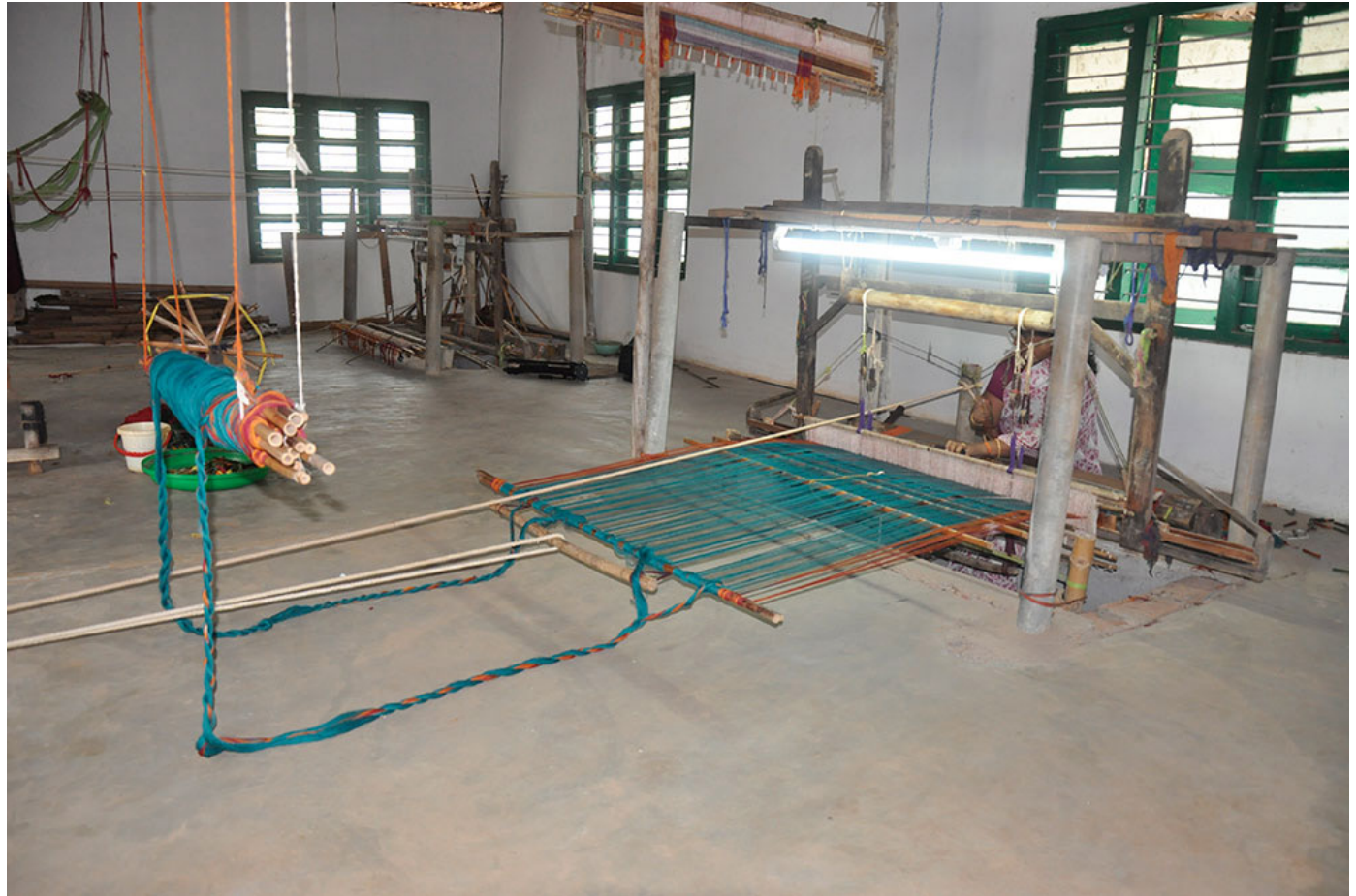
Pit loom is the most popular handloom used for making of the Kandhingi saree.
