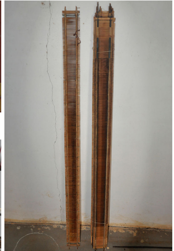
Reed is part of a loom which separates the yarns and keeps them in their positions.
