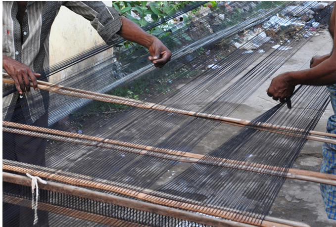
Bamboo sticks is placed in between the cotton yarns to segregate each yarn.
