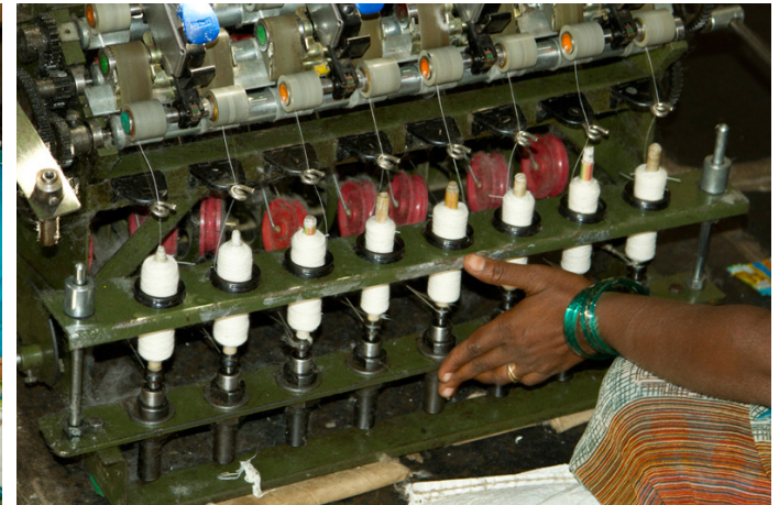
The spinning machine spins 10 spindles together which saves time.
