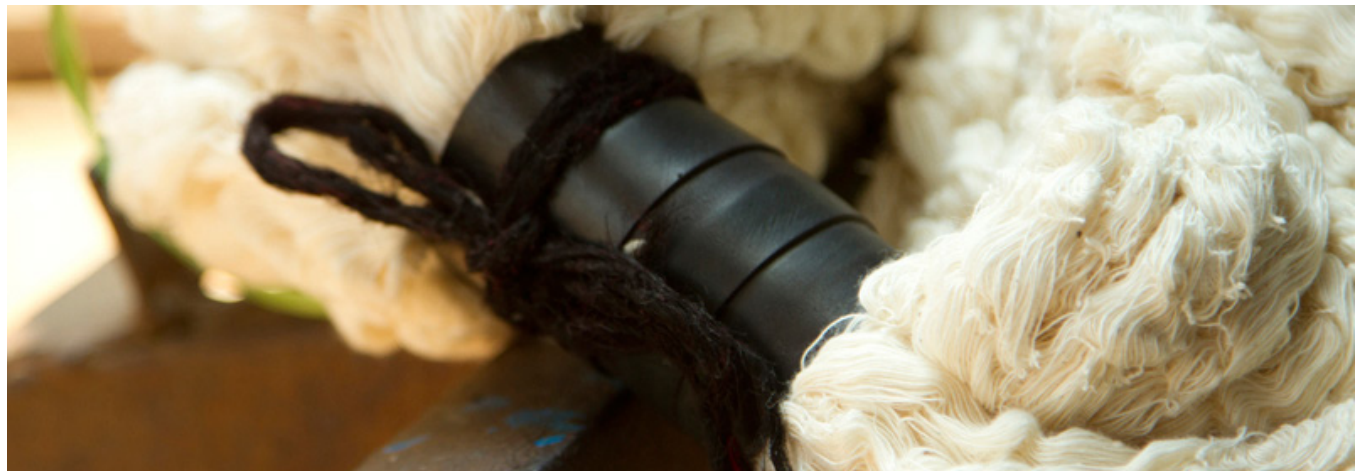
The area of cotton yarns which doesn't have to be dyed is tied with rubber tape.
