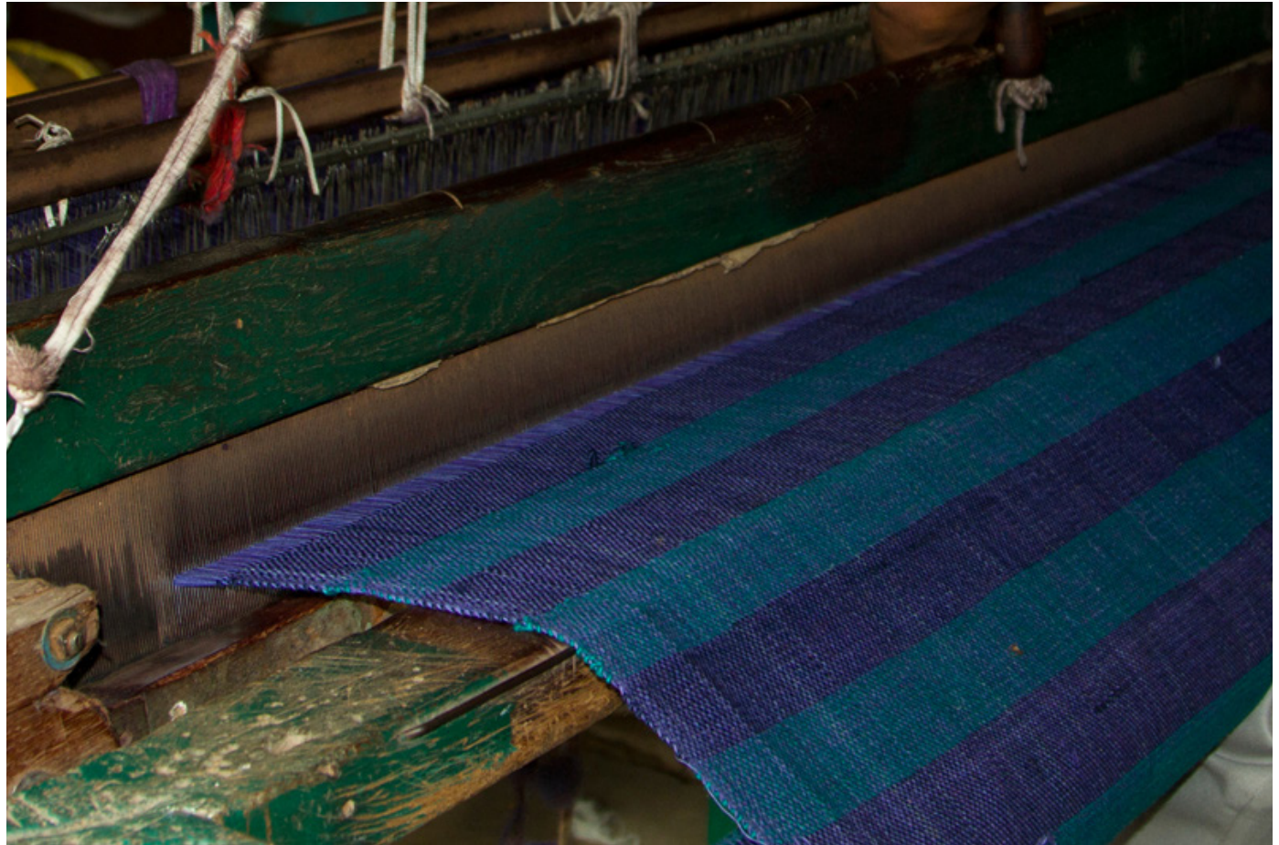
Weaved part of fabric is rolled to a wooden roll attached to the loom.
