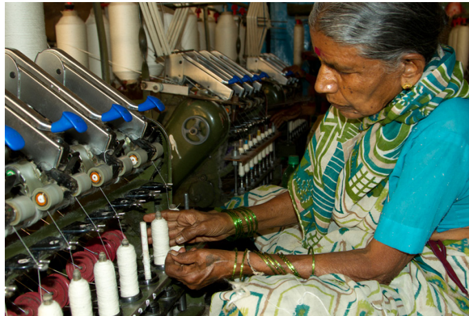
Yarns are spun into bigger spindles from small spun spindles using a spinning machine.
