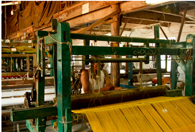
Traditional weaving loom made of wood.
