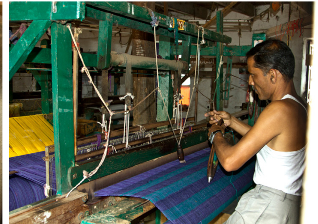
To create patterns different color threads are inserted in fly shuttle and weaved.
