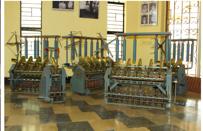
The cotton threads are spun in spindles in the spinning machine.
