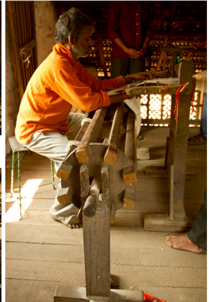
The cotton threads are spun on weaver's beam which is attached to the loom for weaving.
