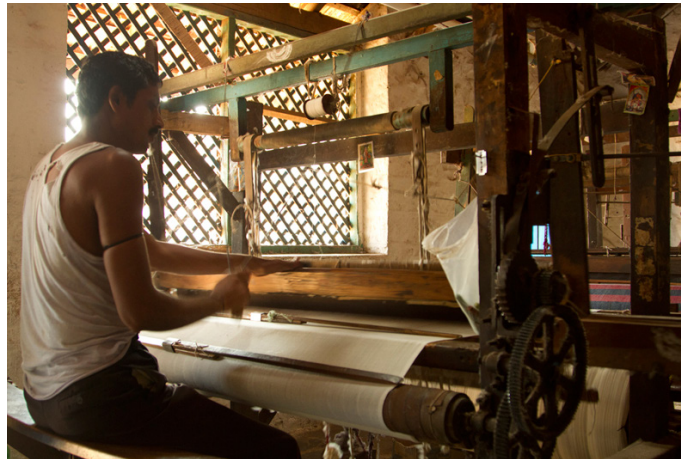
The khadi fabric is weaved on wooden weaving loom.
