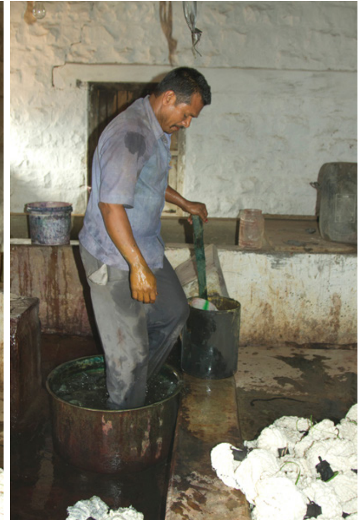
Yarns are stamped to dye the thread for better absorption of color.
