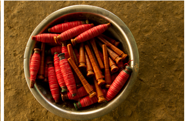
Spindle is used to insert in the flying shuttle for weaving process.
