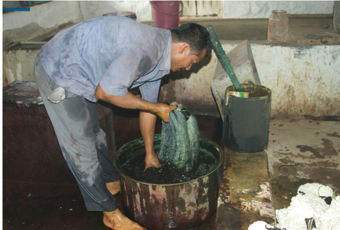
Yarns are dyed 2 to 3 times to get the darker shade.
