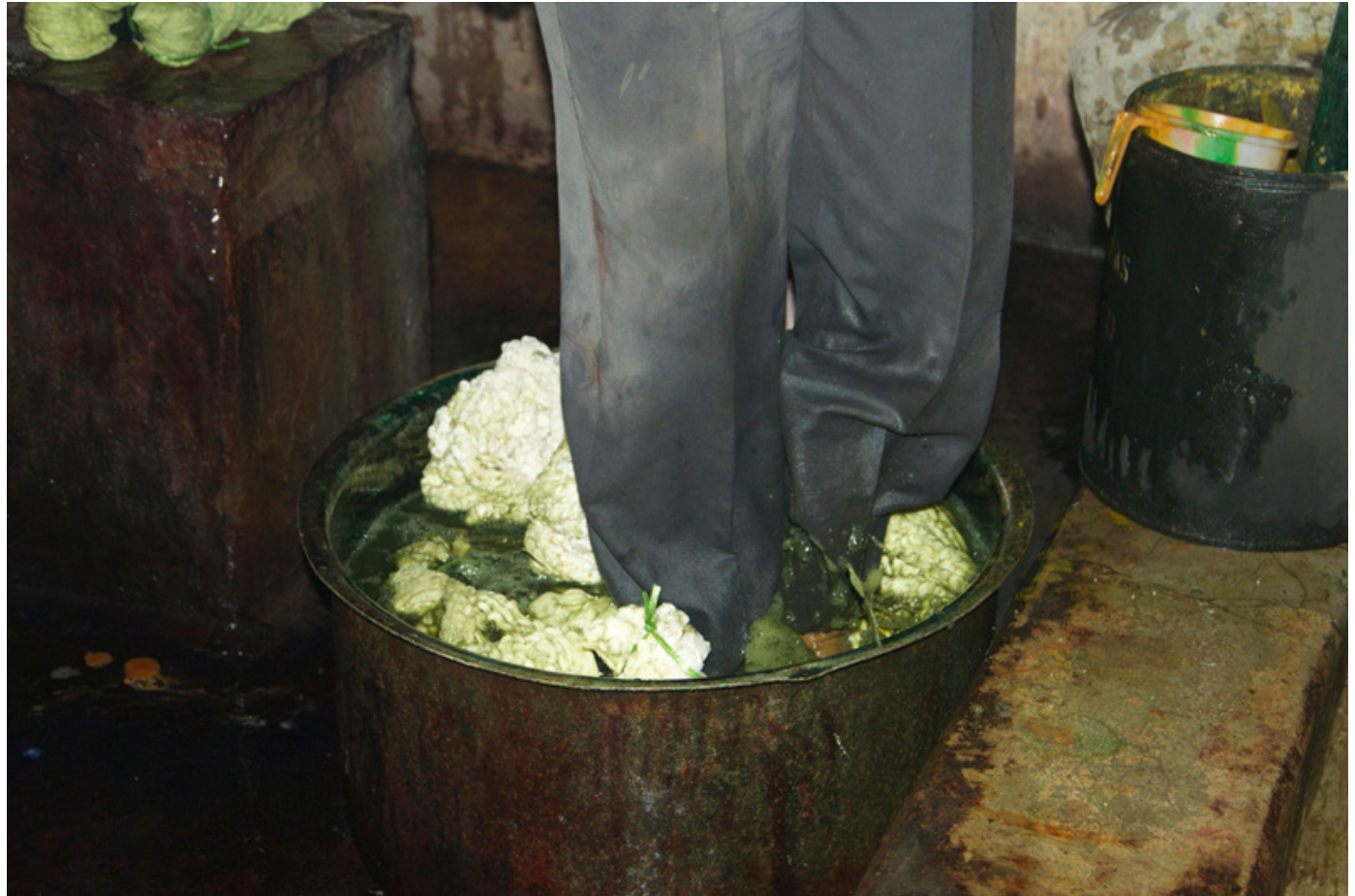
The cotton yarns are immersed in the dye solution.
