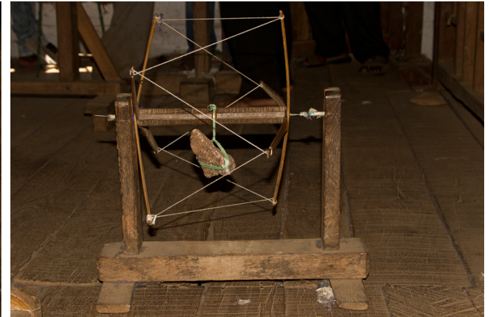
Charkha used to convert the yarns into spindles.
