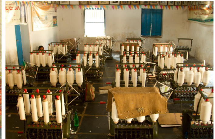
Cotton threads are spun into spindles on cardboard roles.
