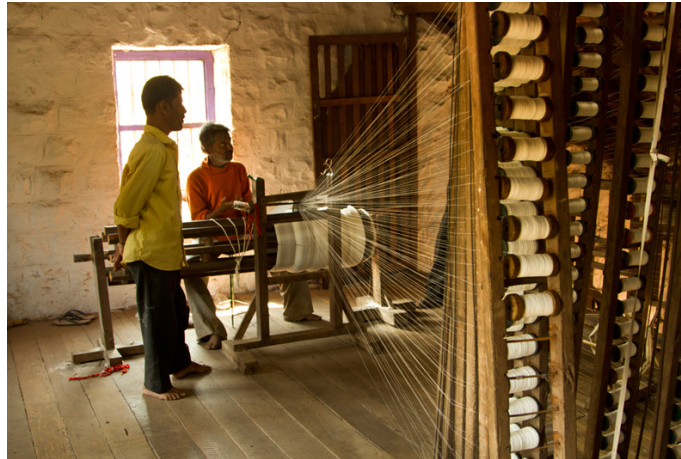
From the spindles, the yarns are spun into warp.
