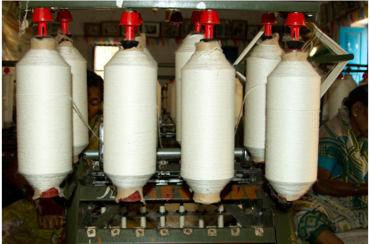
The yarns are spun on cardboard rolls, which are locally known as Hanji cones.
