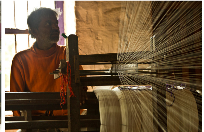
The cotton threads are spun onto warp beam.
