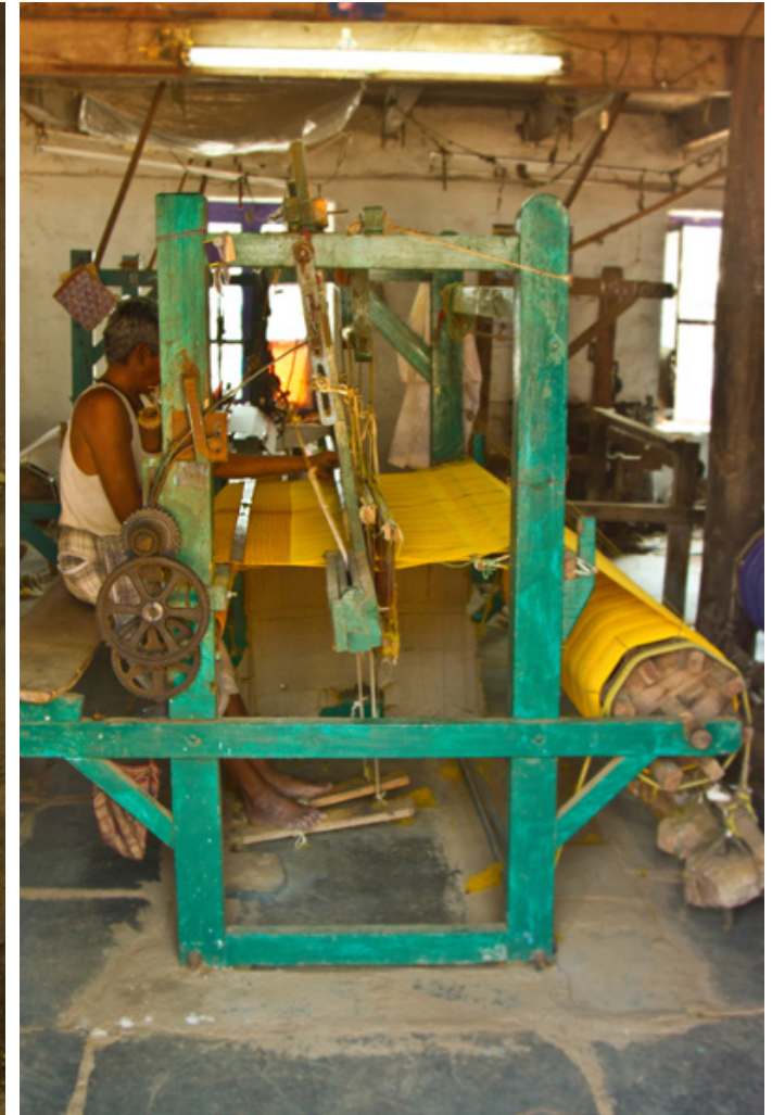
Pedal weaving loom with gear mechanism used for weaving.
