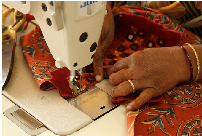
Cutout fabric pieces are stitched together and embroidered piece is stitched on the fabric.
