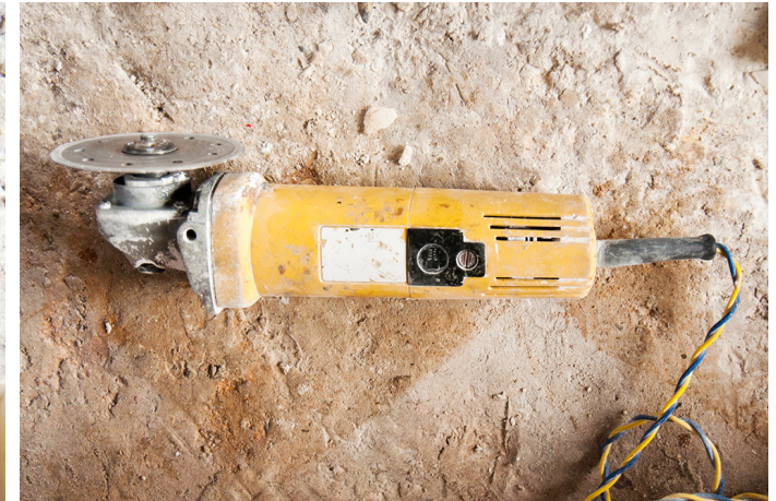
Motorized cutting tool used for cutting marble stone.
