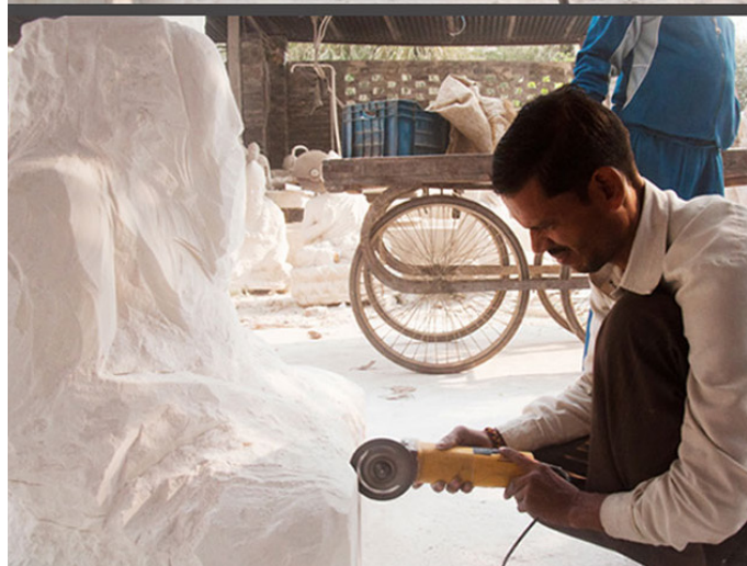
Preliminary rough details of the idol are made using motorized cutting tool.
