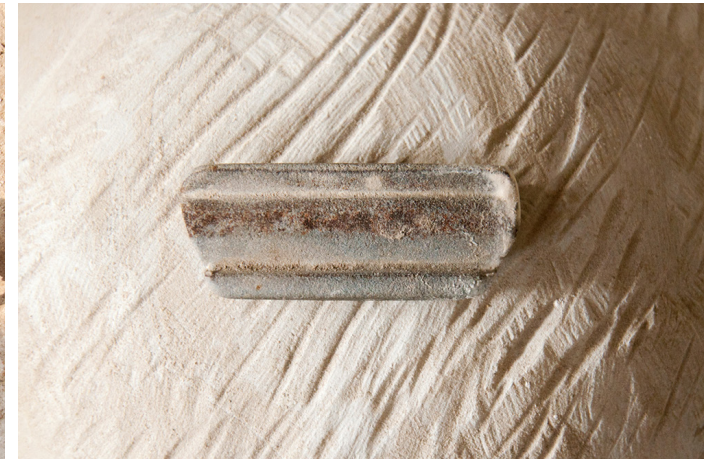
A tool that is used for checking the bevel and carvings of marble stone for its alignment and accuracy.
