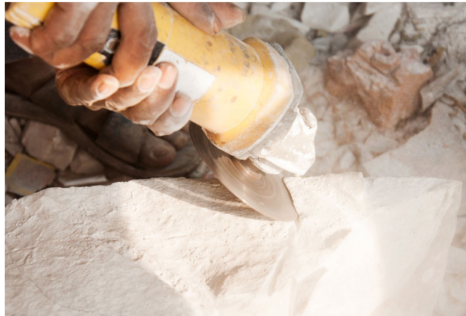
As per the markings the initial layer of marble stone is cut.
