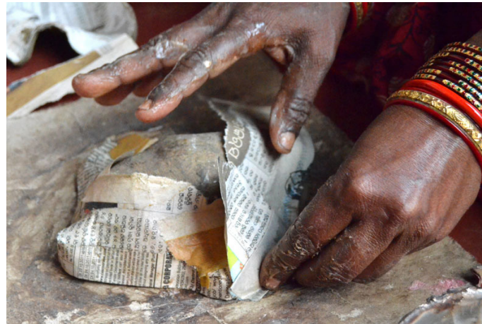
Paper pulp being layered with gum to make it take the shape of the die.
