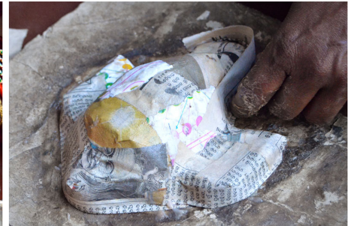
Paper pulp being layered with gum to make it take the shape of the die.
