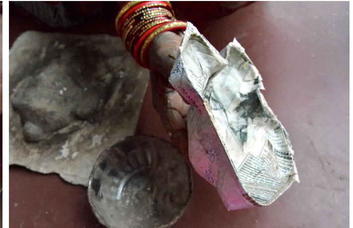
First layer of paper is removed from the die.
