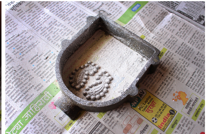
Evenly spread ammonium chloride on casting frame.
