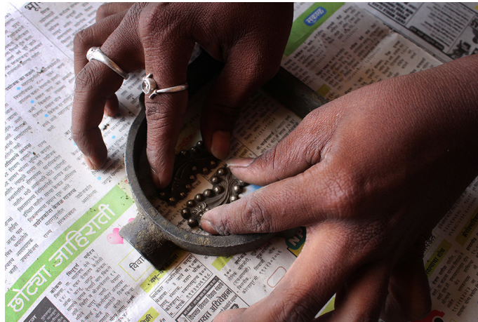
The accuracy of artisan placing the stencil inside the casting frame.
