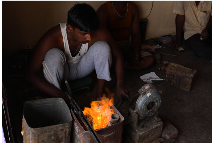
Craft man blowing the fire for melting silver.
