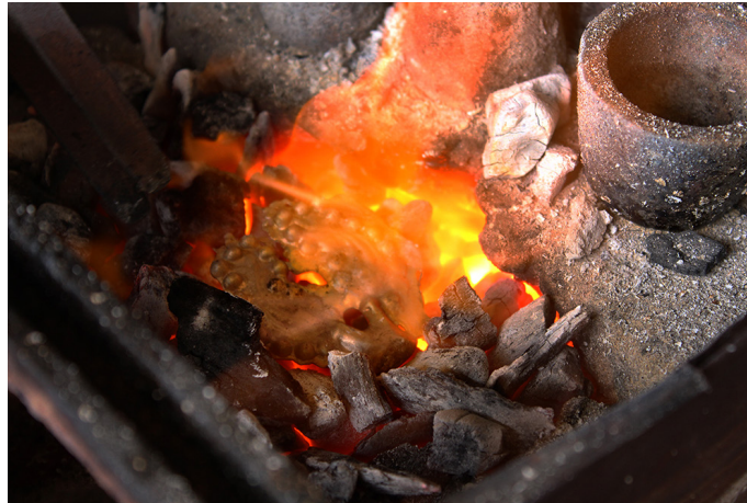
Heating the casted artifact once again to make it tender.
