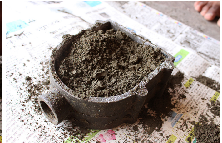
The rest of the part also filled with molding sand.
