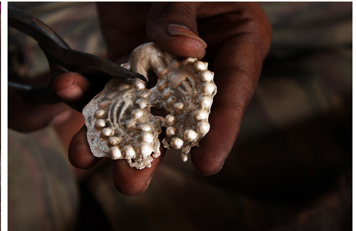
Cutting the joints of artifact for separating them.
