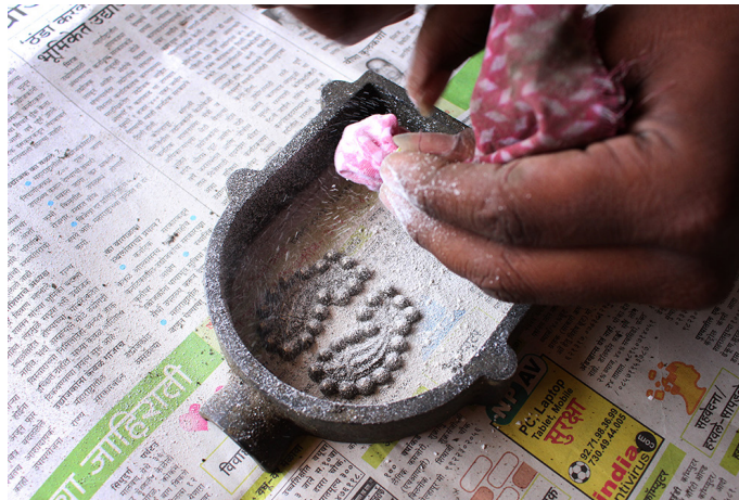
Artisan evenly sprinkling ammonium chloride.
