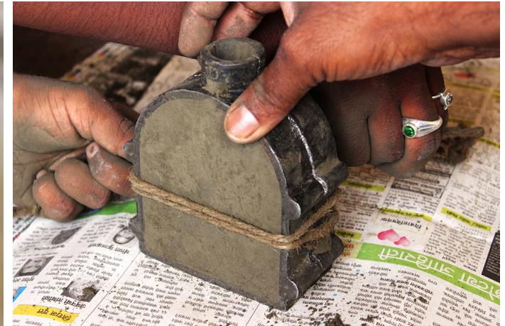
Knotting the frames tightly together to avoid air circulation.
