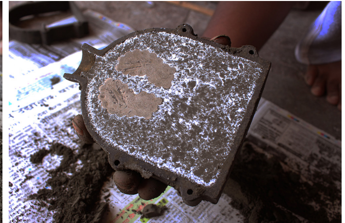
Interior view of casting frame after filling the sand.
