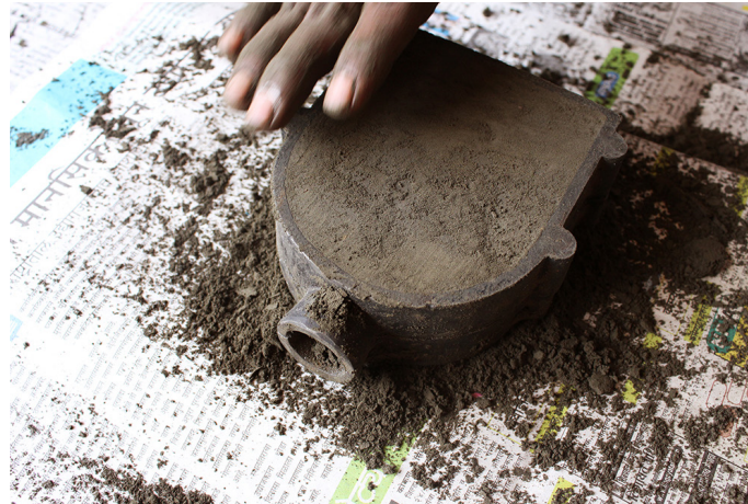
Cleaning the sides and removing the sand.
