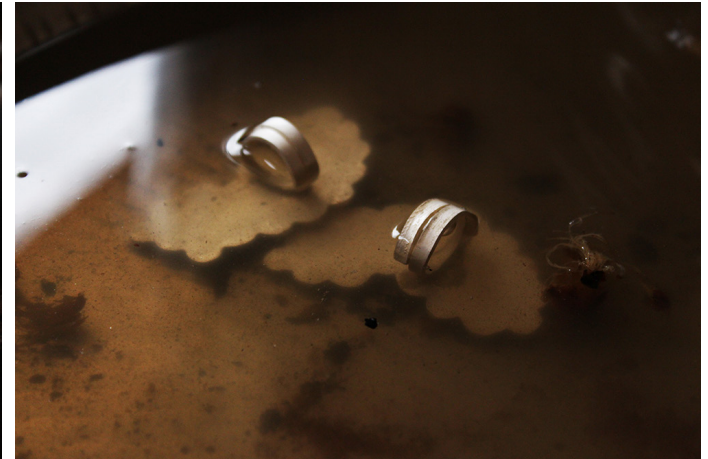
Soldered toe rings are kept in water for cooling down.
