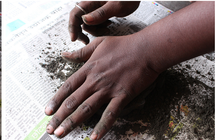
Pressing the sand thoroughly to achieve a perfect casting mold.
