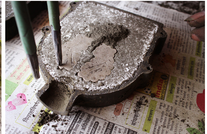
The edges of stencils are gently pressed to remove it from the mold.
