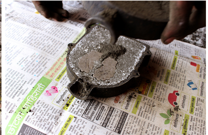
Separating the frames into two parts.
