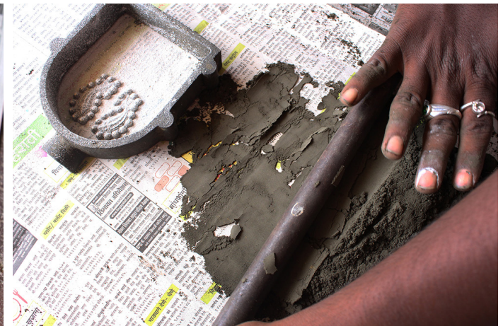
Artisan making the molding sand even more fine and lenient.
