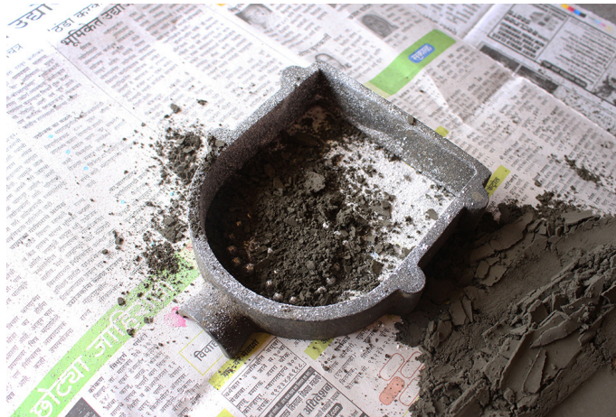
Filling the frame with molding sand.
