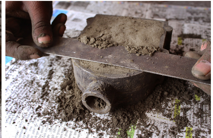
Artisan removing the excess amount of sand from the frame.
