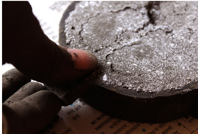
Removing the sand for creating path for molten silver.
