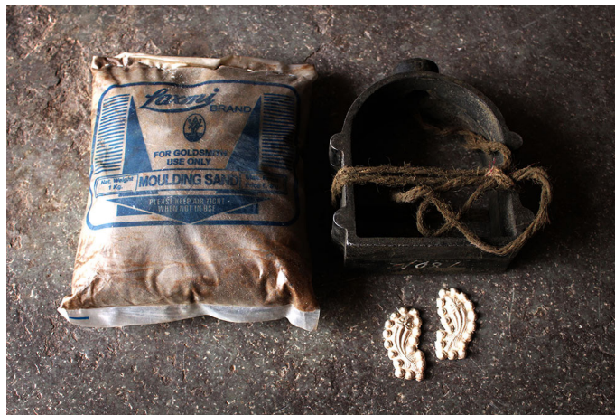
Left to right: Molding Sand, Casting Frame and Stencil Design.
