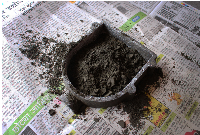
Making process of casting mold.
