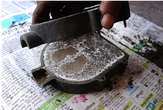
Placing the remaining part of frame for completing the mold.
