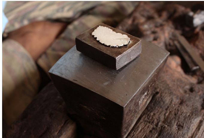
Casted artifact places on the cavities of pressing die.
