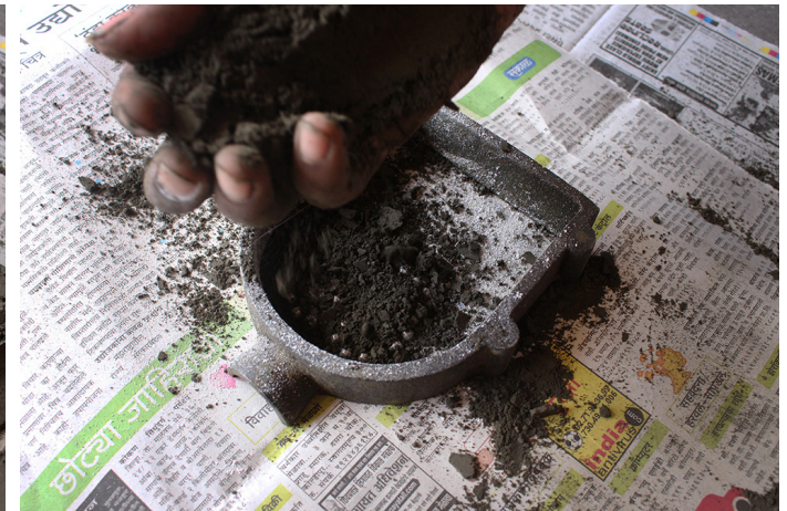
Filling the frame with molding sand.
