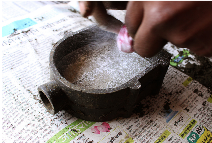
Artisan evenly sprinkling ammonium chloride.
