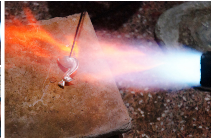
Joining the two parts of the peacock by heating.
