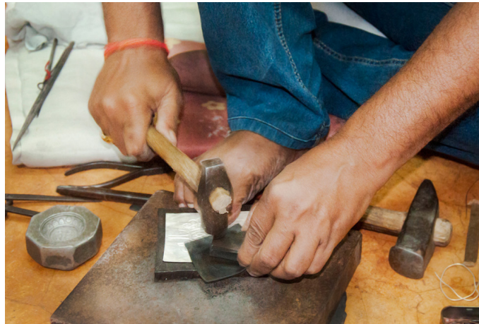
Embossing the metal sheet by hammering.
