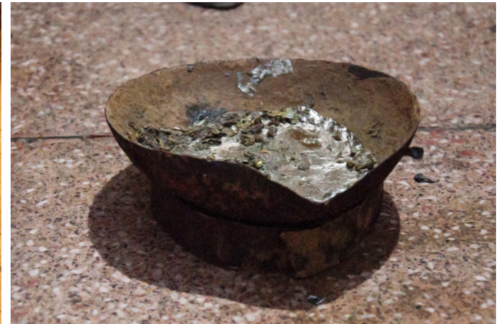
Crucible is used to melt silver waste.
