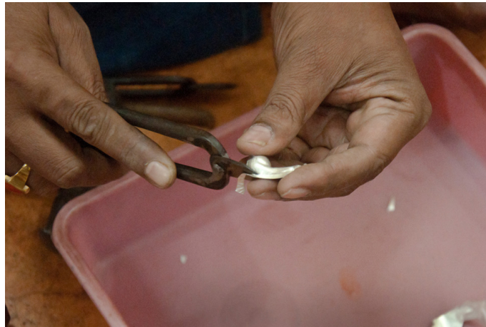
Removing unwanted metal with the help of metal sheet cutter.
