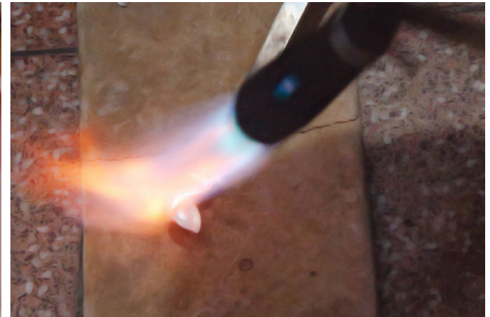
Hand gas burner is used to heat the embossed craft piece.
