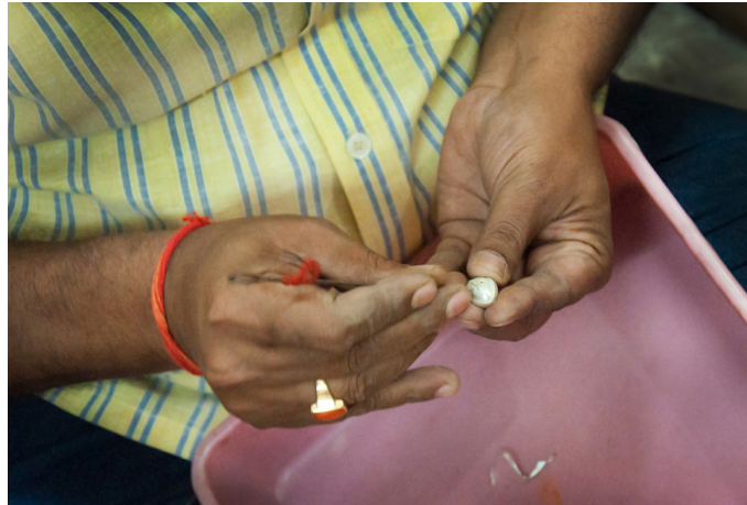
Artisan piercing the metal sheet to make a hole.
