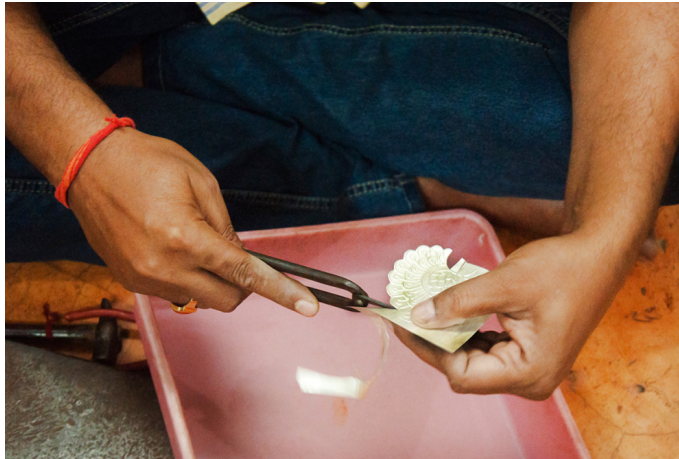
The unwanted metal is removed by using metal sheet cutter.
