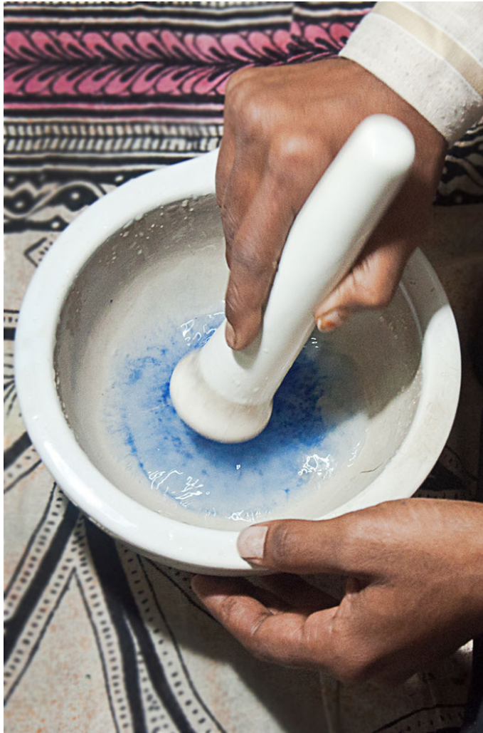
Grinding the colour glass with water to make fine powder.
