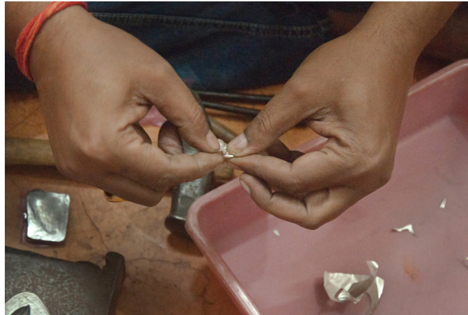
The two embossed parts are attached by binding wire.
