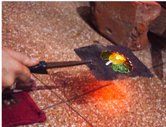
The craft is heated to retain the colour for long time.
