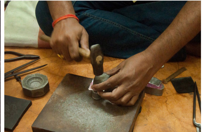
Preheated embossed sheet is hammered.
