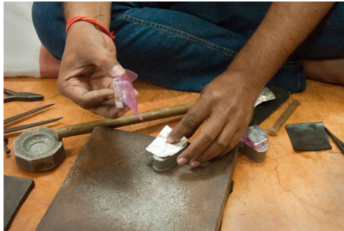
Silver sheet is placed on the mold.
