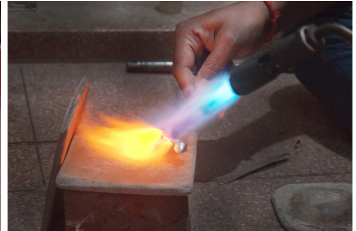
The embossed part is reheated.
