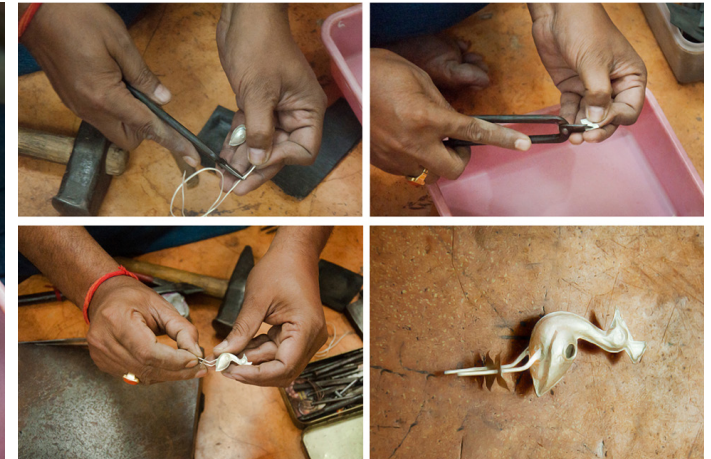
Using silver wire and silver sheet does the leg part of the peacock.
