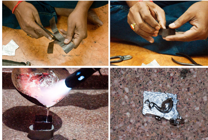
Metal casting by melting silver waste in crucible.
