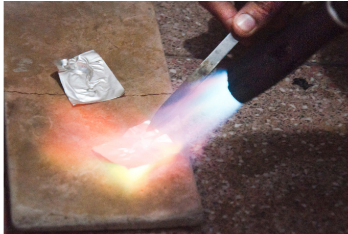
Heating the embossed metal sheet to make it soft and easy to bend.
