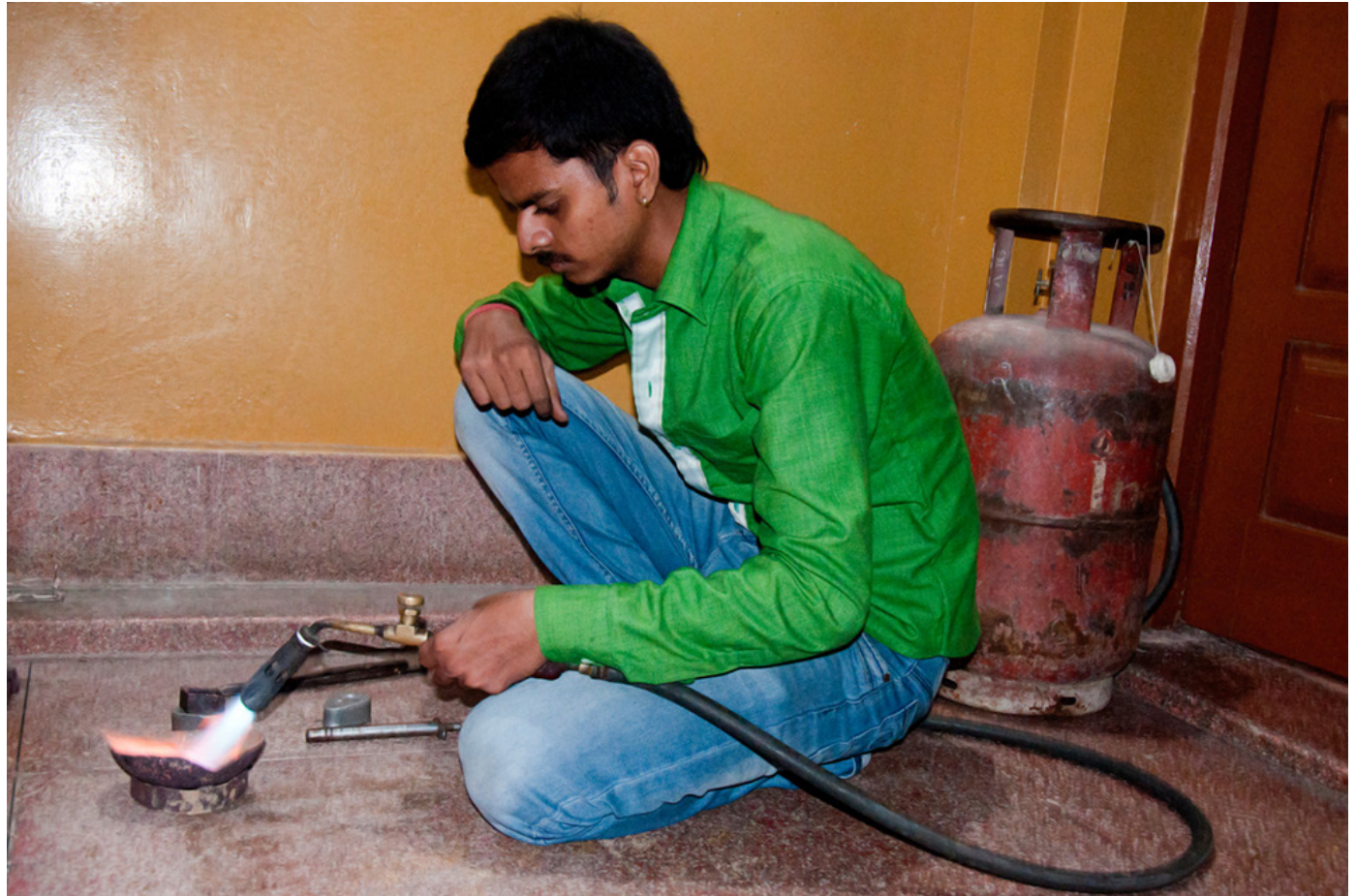
Hand gas burner is used to heat the silver sheet.
