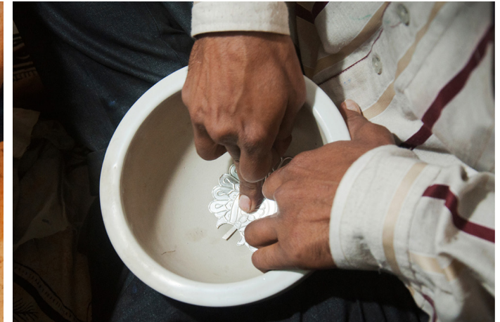
Bending the embossed silver sheet.
