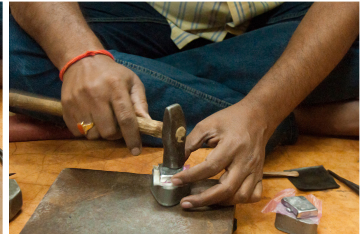
Hammering the sheet by placing the impression tool to get a required shape.
