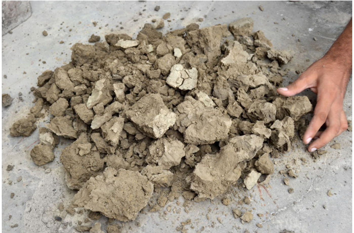
Pieces of solid clay being broken down.
