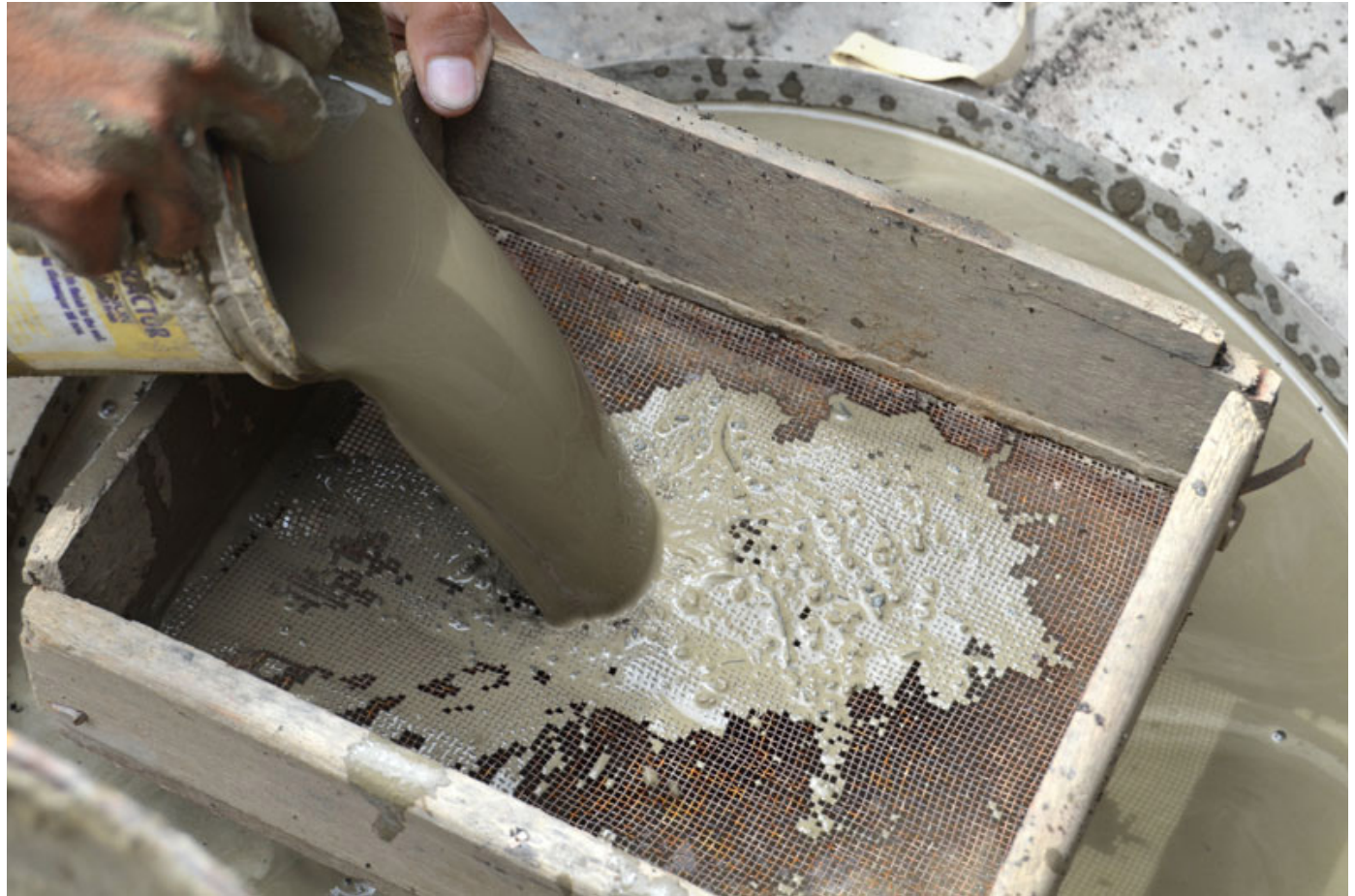
Watery clay sieved through a fine mesh to remove tiny stone pieces.
