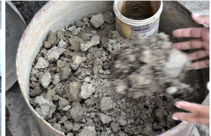
Clay pieces being mixed with water.
