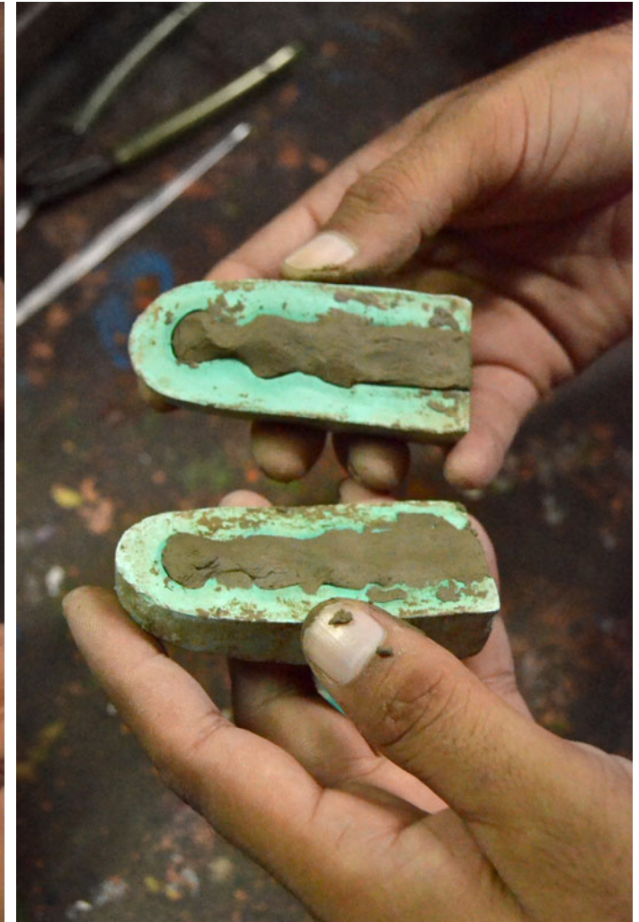
Small piece of clay to be rolled and placed between two halves of the mould.
