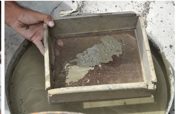
Watery clay sieved through a fine mesh to remove tiny stone pieces.
