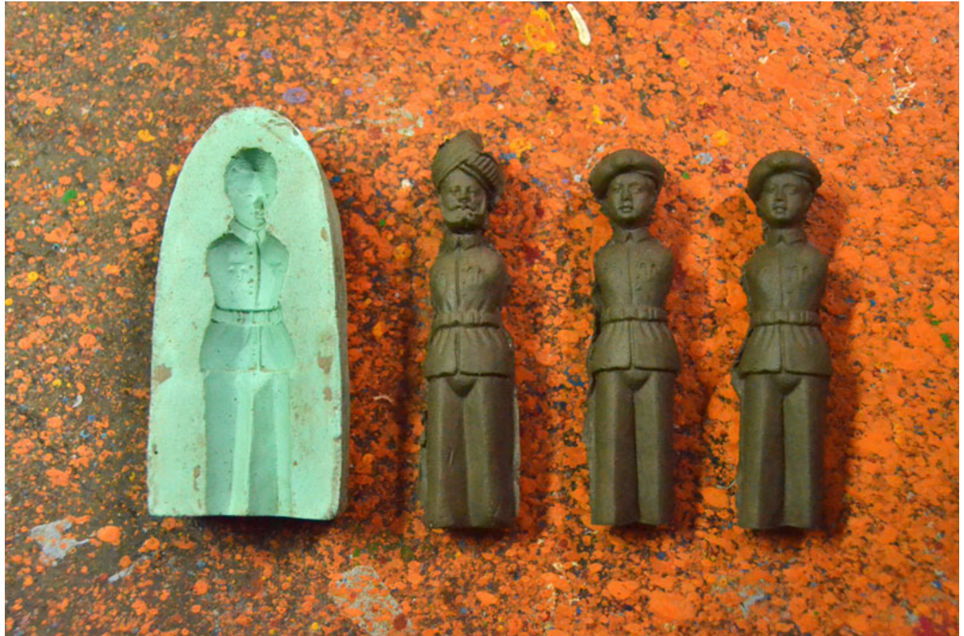
Mould and the figures cast from it.
