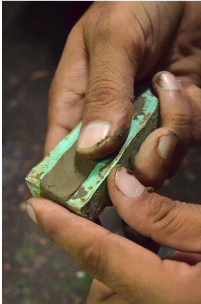
Small piece of clay to be rolled and placed between two halves of the mould.
