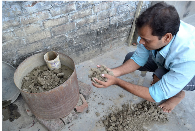
Clay pieces being mixed with water.
