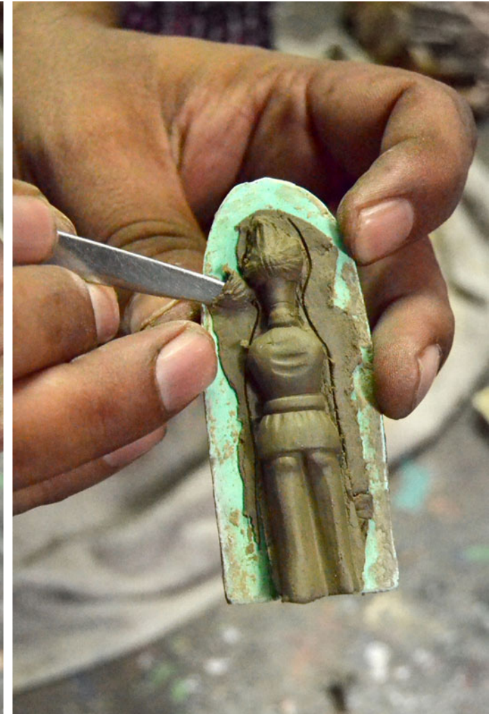
Figure being removed from the mould.
