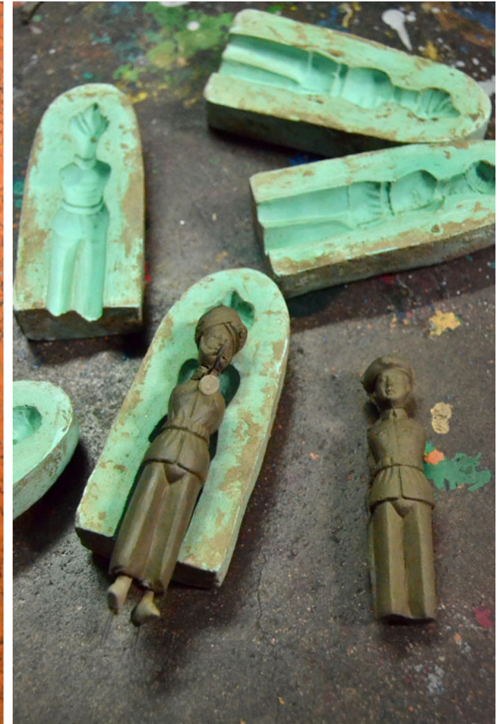
Moulds and the figures cast from them.
