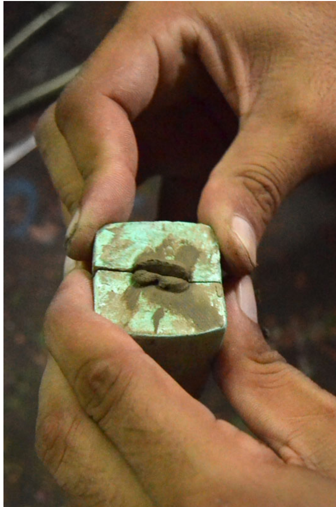
Clay being firmly pressed to form the figure.
