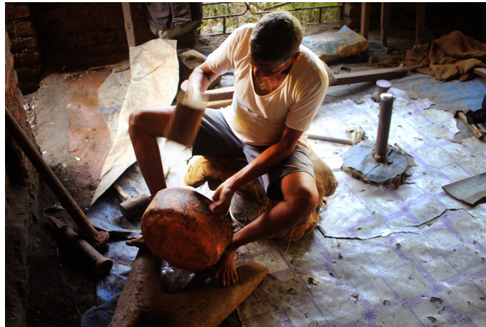
Beating the copper on Sandhan( an iron rod with smooth surface) to give even texture.
