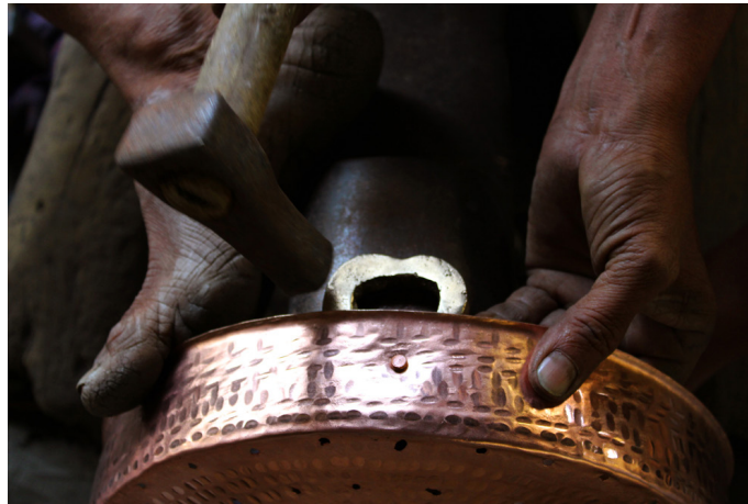
Applying tin on hot copper.
