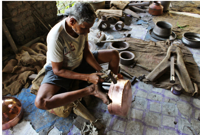
Interior of steamer plated are beaten with Chauras dabak(squire iron hammer).
