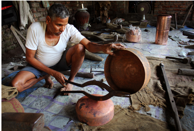
Trimming the copper to an accurate size of steamer plate.
