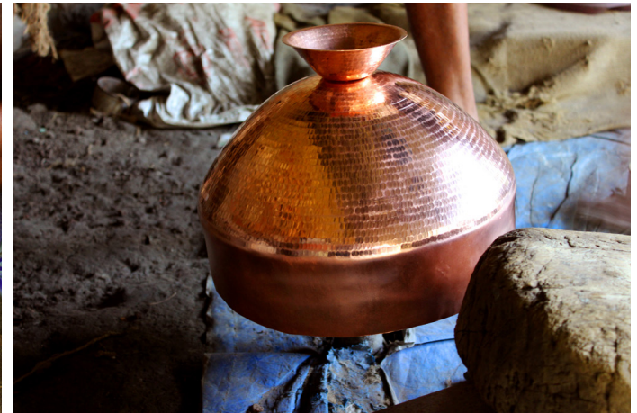
Texture of the copperware is given by beating them continuously by using metal hammer and bar anvil.
