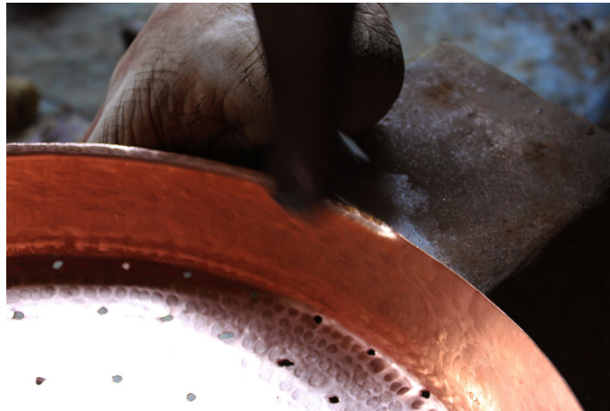
Attaching the handle to steamer plate.
