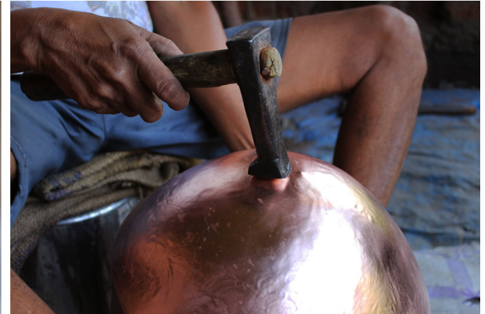
Beating process of copper to give texture and firmness.
