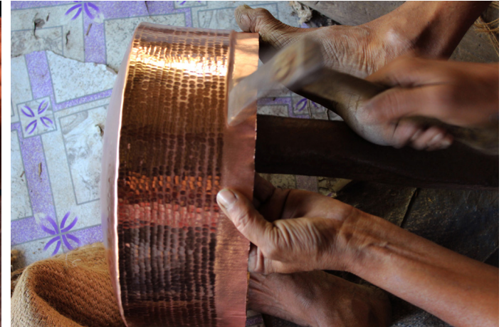
Finishing the edges of steamer plate.
