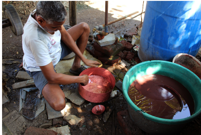
Giving acid wash to copper vessels.
