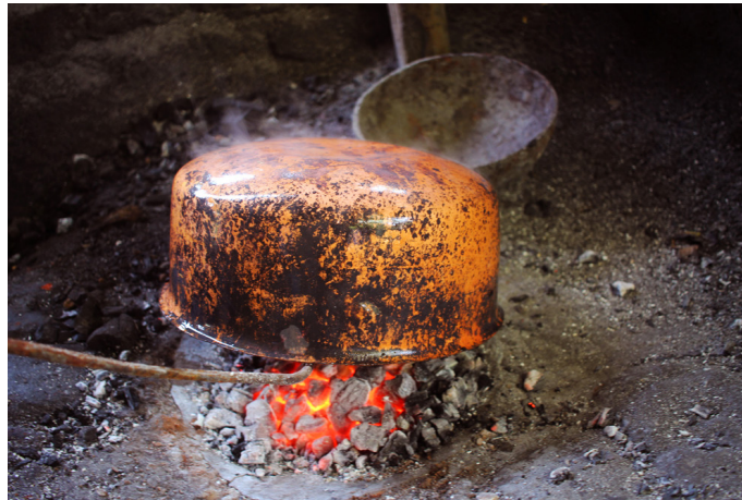
Repeated process of firing copper which makes metal even more tender.
