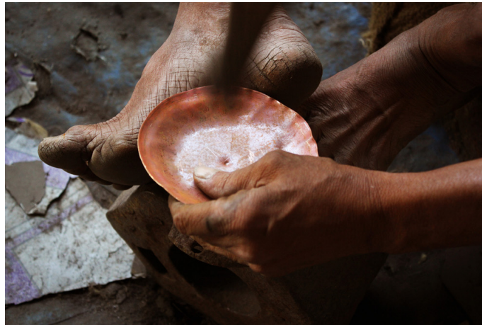
Beating process of copper plate to acquire the shape of phool.
