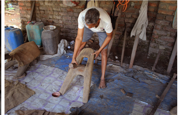
Artisan assembling the khod(wooden frame) and kharvai(bar anvil).
