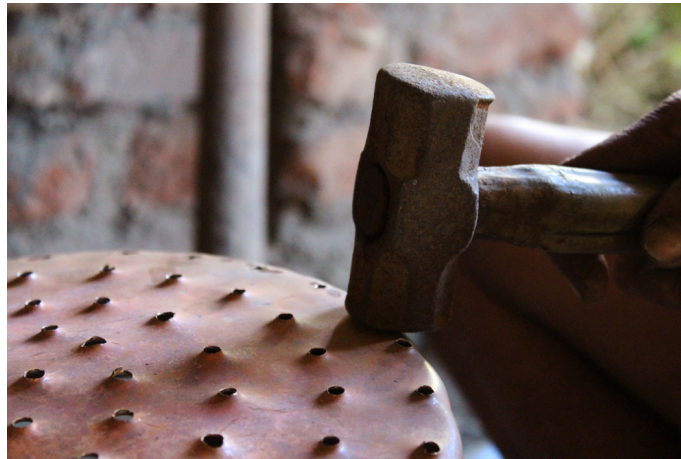
Close up view of flattening the rough surface with the help of dabak(iron hammer).
