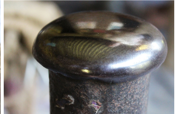
'Sandhan' a multipurpose tool which delivers smoothness to the copper surface.
