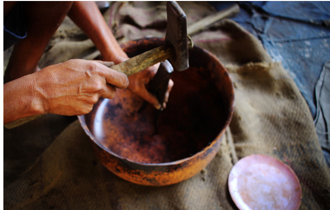
Artisan marking the centre point with the help of traditional tools.
