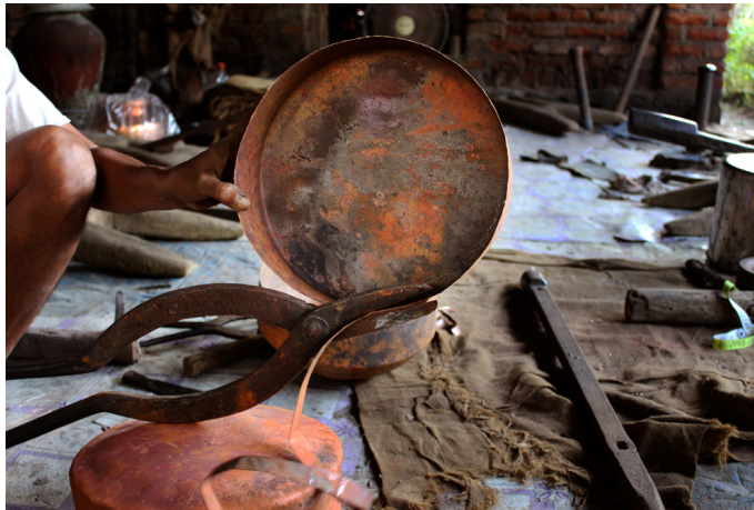
Artisan using the traditional cutting tool 'Katri' to trim and size copper.
