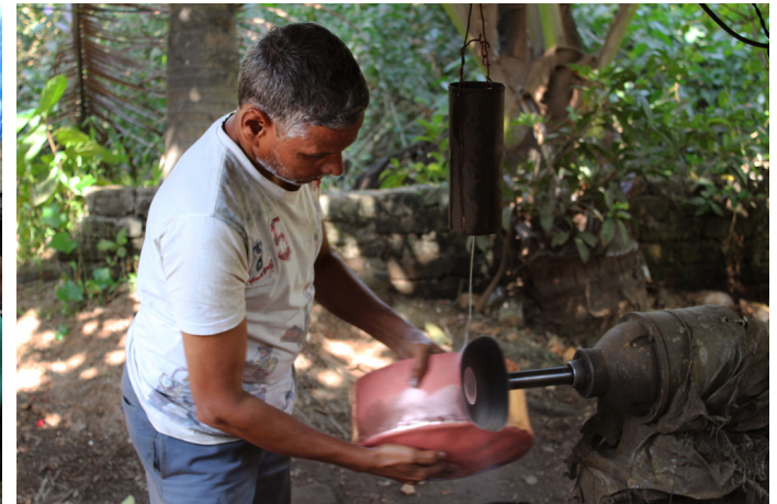
Buffing the copper with the help of electronic buffing machine.
