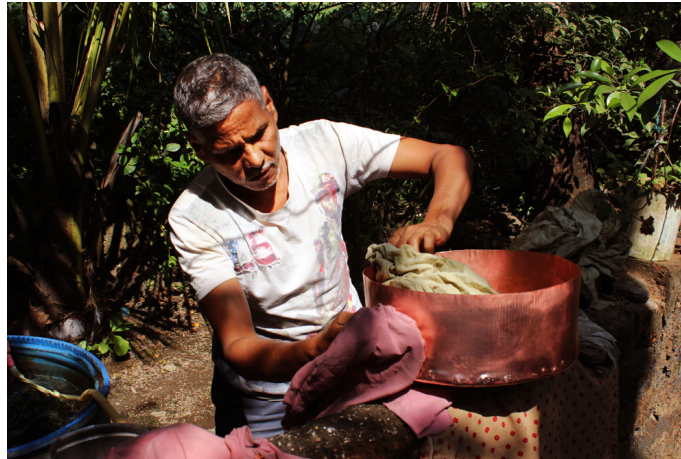
Wiping thoroughly and ensuring no water left on copper to avoid stain marks.
