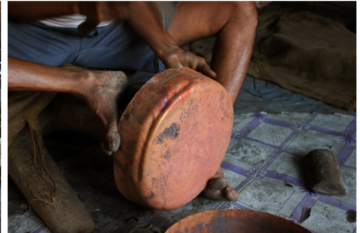
Beating process of steamer plate on Kharvai(bar anvil).
