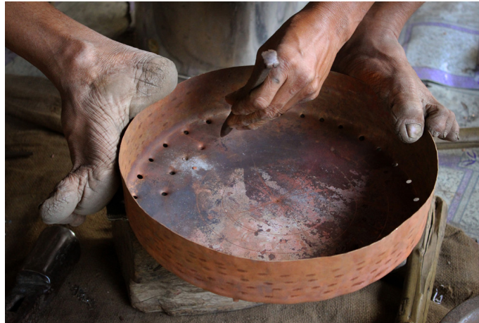
Punching holes on steamer plate by using Togar (the big iron nail).
