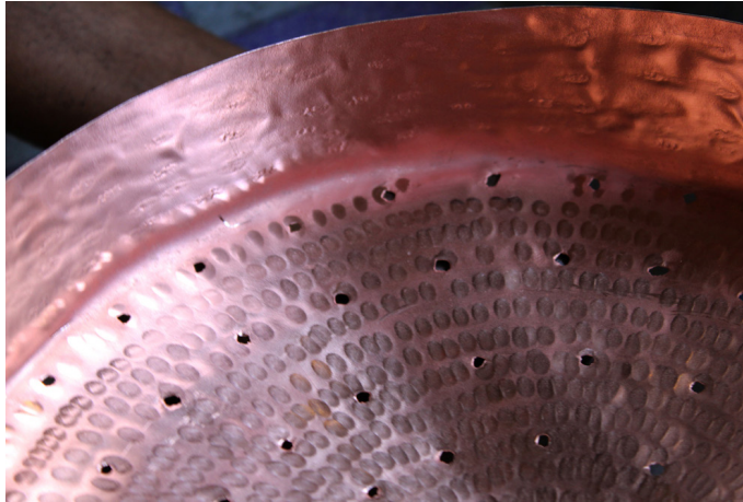
Finishing the edges of steamer plate.
