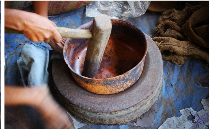
Making of lid: Mogri(wooden hammer) and Adi( circular shaped iron tyre) the tools which is used to obtain the dome shape.
