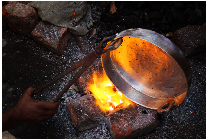
Artisan creating circular patterns by using chavarshi dabak.
