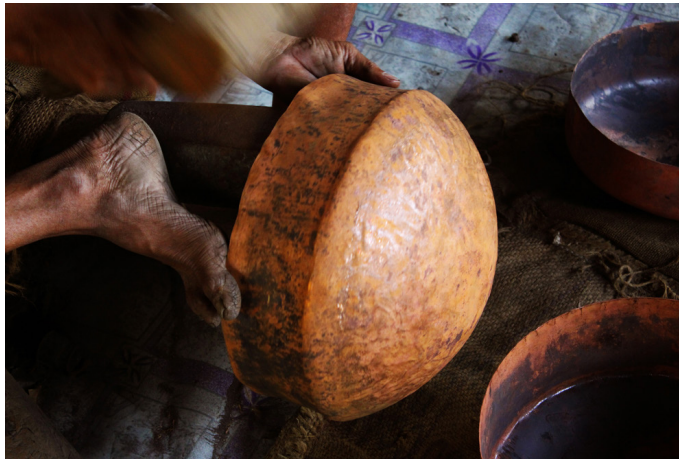
Final touch up of the lid to attain accurate fitting.
