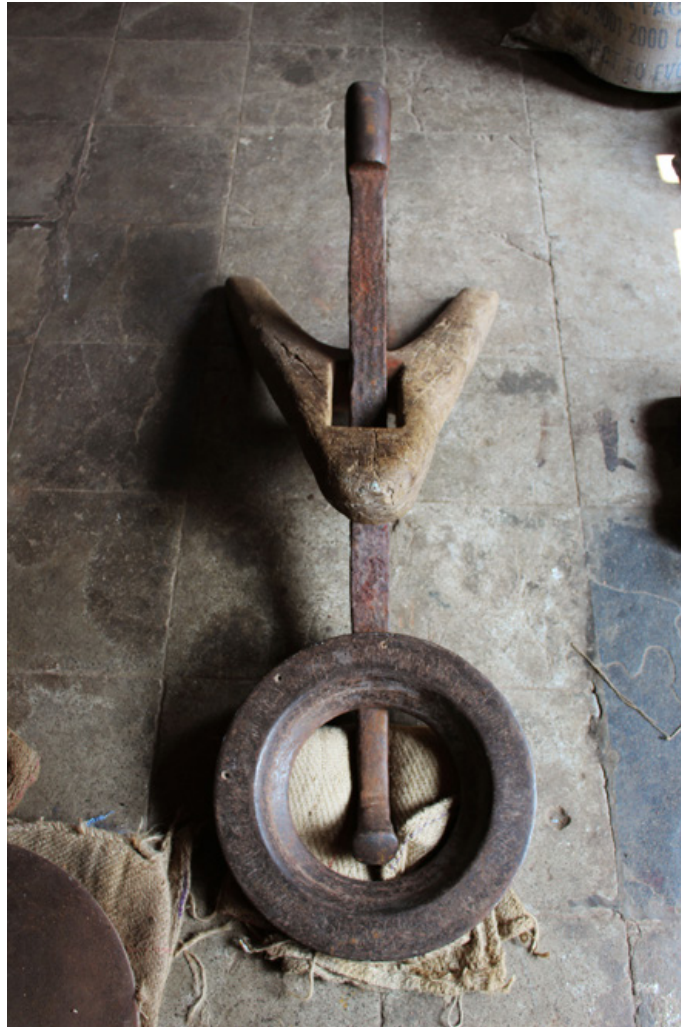
Composition of tools 'Kharvai(bar anvil), khod (wooden frame), and adi(circular iron tyre).
