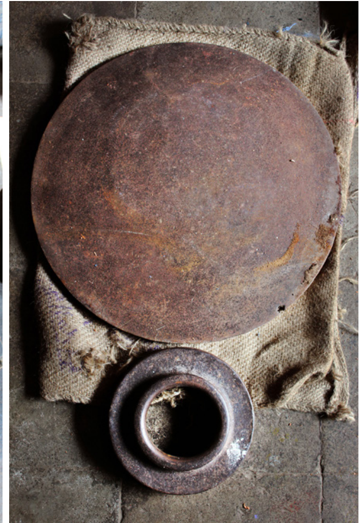
Iron frame which is used for making copper plates and mandli(smaller version of adi).
