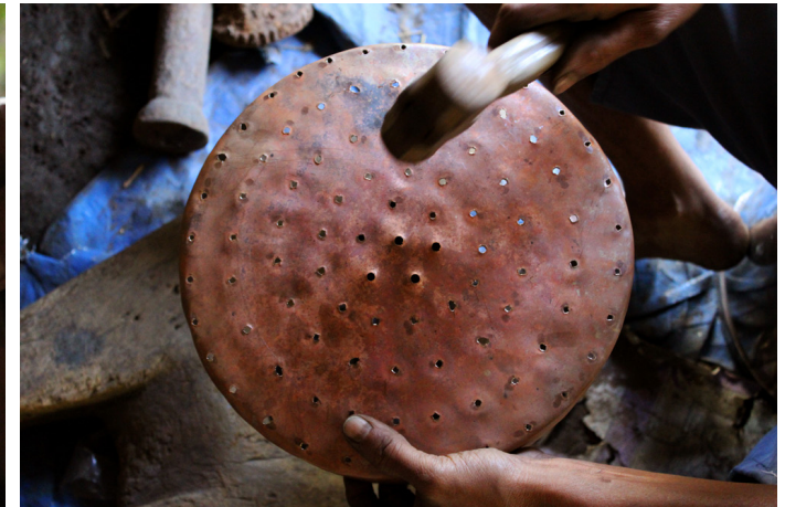
Flattening the rough surface with the help of dabak(iron hammer).
