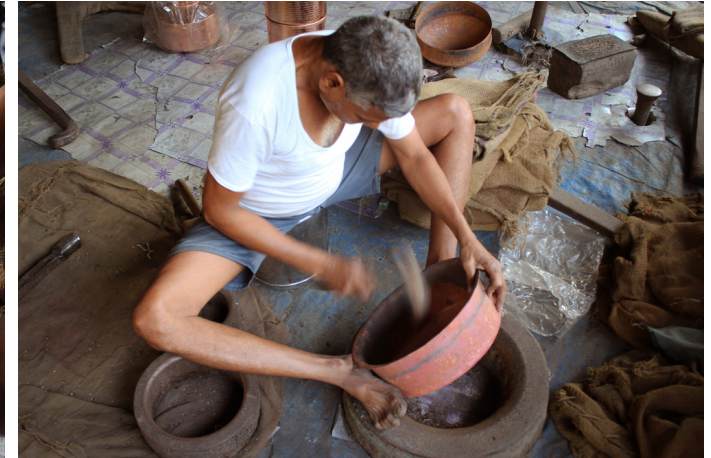
Repeated beating process on Adi( circular shaped iron tyre).
