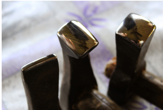
Chavarshi, Nakhi, Chauras dabaks are the iron hammers which are used for beating and giving texture to copper vessels.
