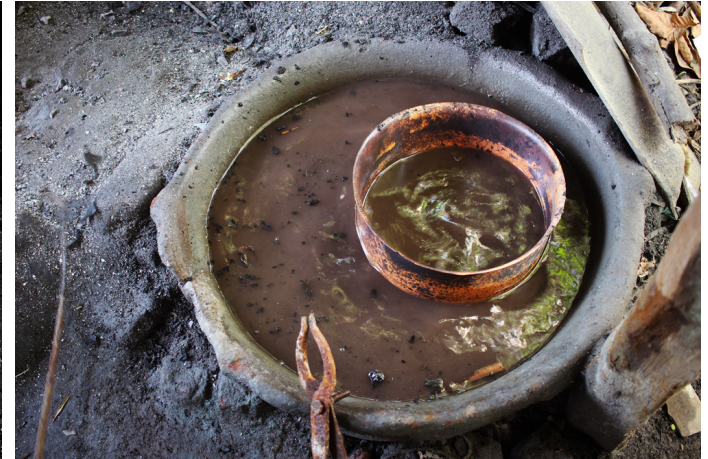
Cooling the fired copper in water.
