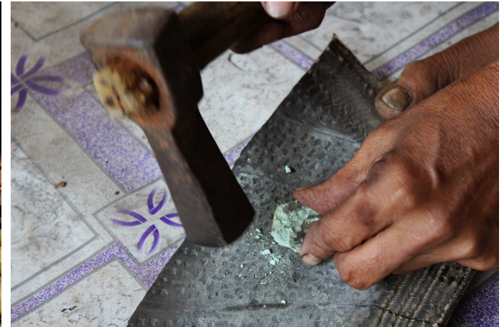
Polishing the dabak (iron hammer) to give fine and smooth surface.
