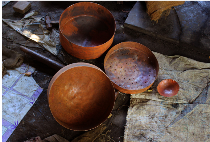
The four elements of Modakpatra after obtaining their shapes.
