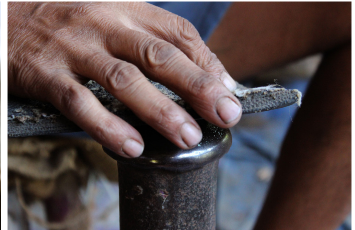
Close up view of Sandhan(an iron bar which has a very shiny and smooth surface).
