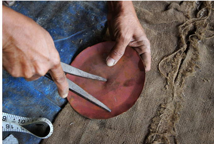
Marking the radius of phool(lid handle).
