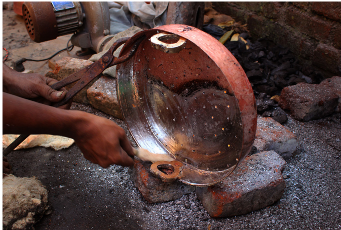
Punching the dome shaped lid with traditional tools for fixing handle.
