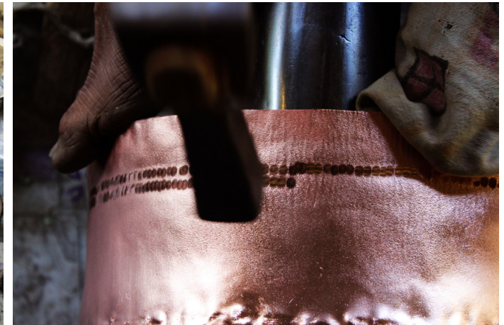
Beating the base vessel with Chavarshi dabak to give bend.
