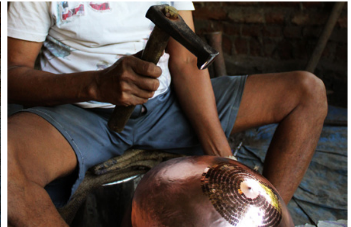
Base vessel is beaten on Kharvai to give glow and texture.
