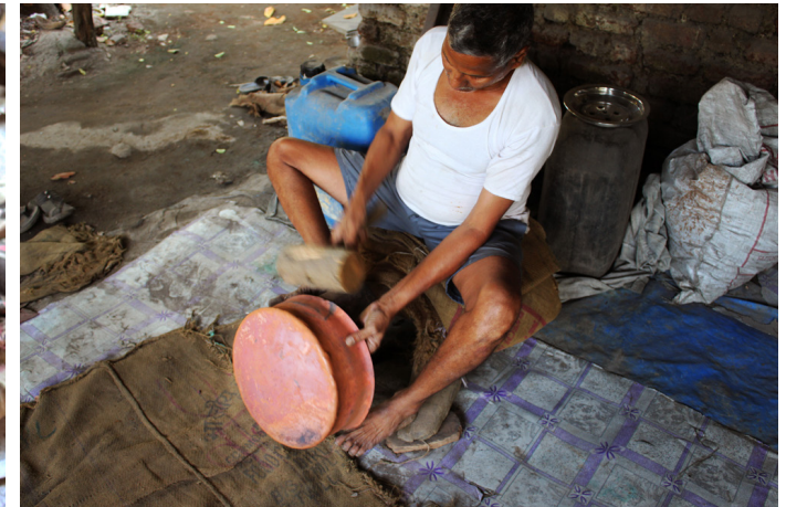
Making of base vessel: copper is getting beaten on Kharvai(bar anvil).
