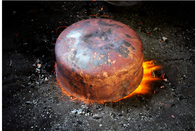
The firing process of copper to make it soft.
