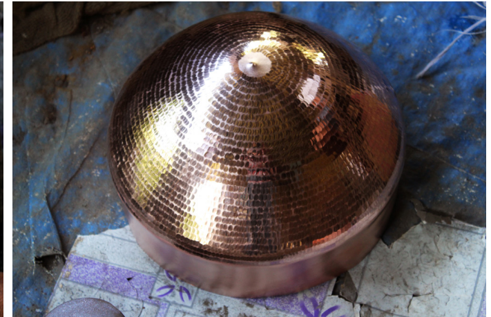
Downside of Steamer plates are beaten by chavarshi dabak (iron hammer) to give a leaf shaped pattern.
