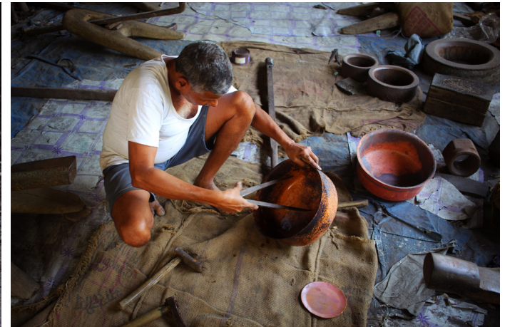
Artisan marking the measurements with the help of traditional geometric compass.
