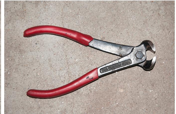
A plier that is used in holding the rubber sole while giving it a shape.
