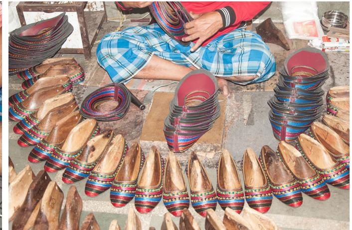
Artisan placing the ready shoes in the mold, as a part of the process.
