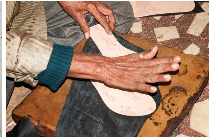
The sole is then pasted to a thin sheet of leather, which gives a soft padding to the legs.
