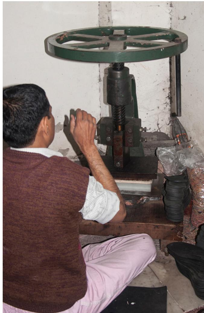
A rubber mat is pressed in the die cut machine, which makes the soul of the Mojari.
