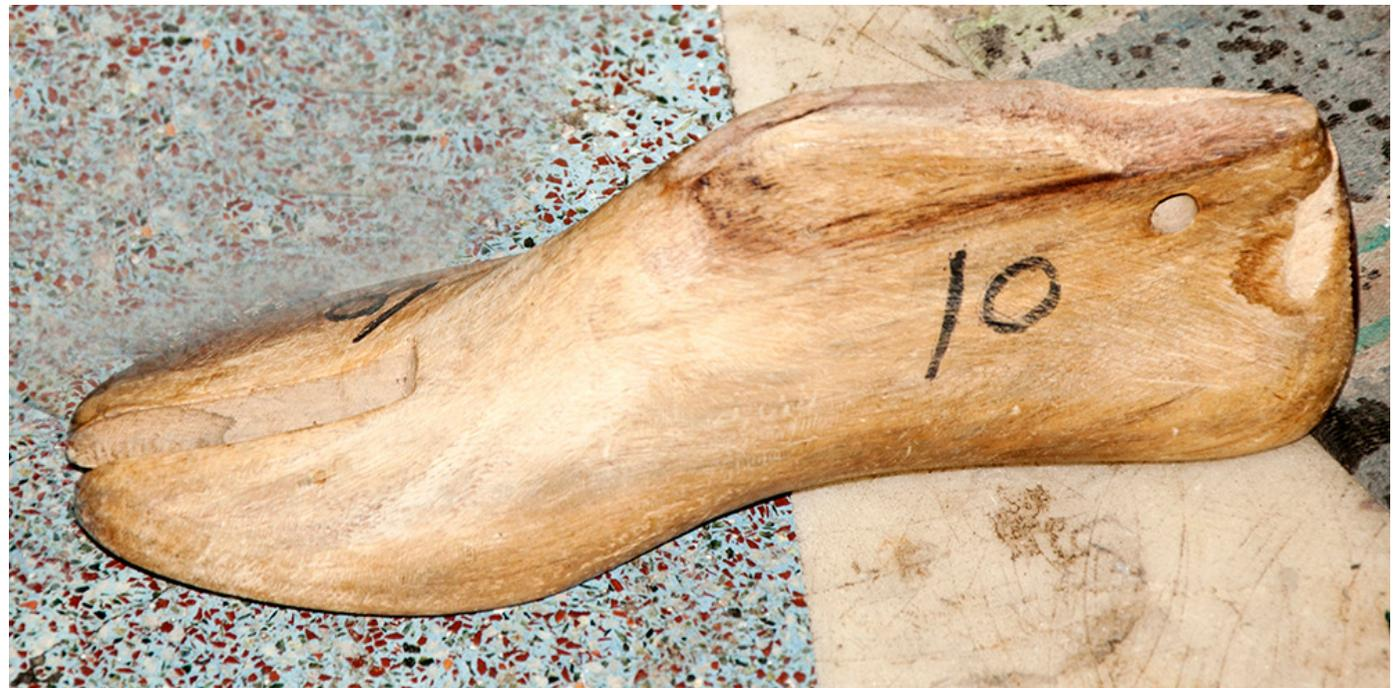
A wooden mold of shoe interior, which is inserted when the shoe is inserted, such that it can take shape of a shoe.
