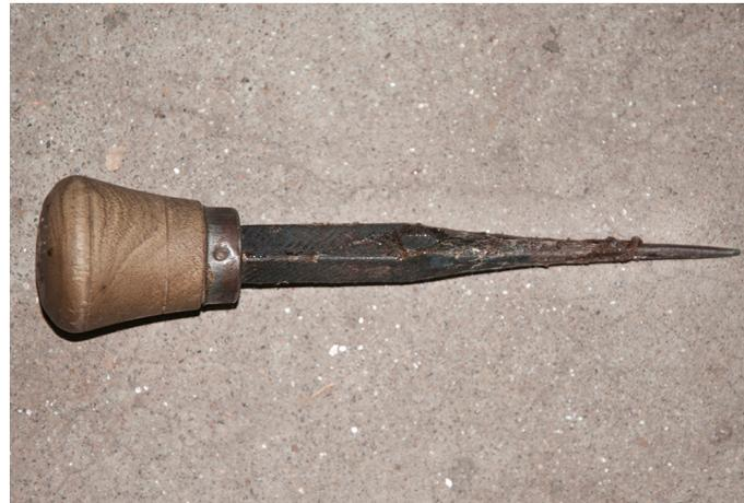
A hole-punching chisel called Katarni, used in punching hole in leather to sew through heavy threads.
