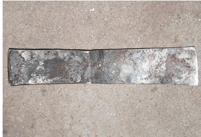
A flat iron chisel used in cutting through leather and thick clothes.
