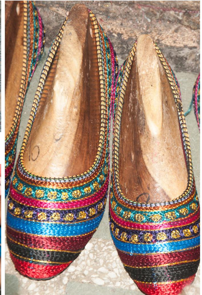
Wooden molds are inserted in the finished shoe piece, so that it retains the shape post drying.
