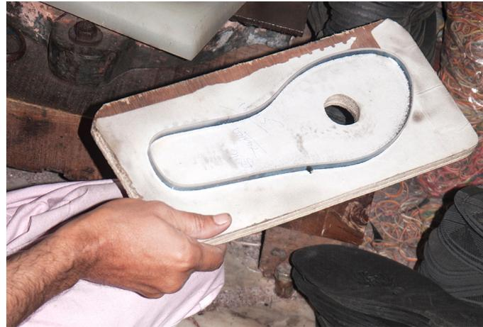
Presses die in the shape of shoe sole, which will cut the soles out of rubber mat, in a press cutting machine.
