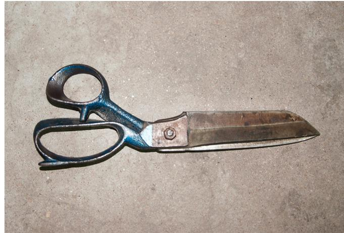
Scissor used for cutting cloth, thread and leather pieces, used in making Mojari.
