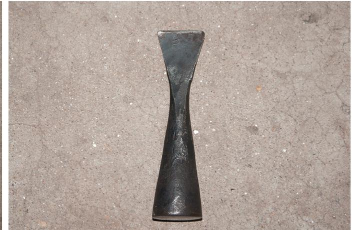
A heavy chisel called Rapi, which is used in tearing heavy leather pieces into required pieces.
