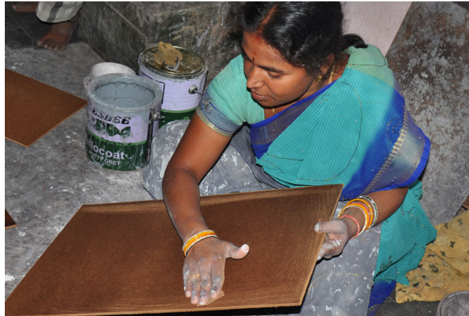
Wooden board is being smoothened by rubbing it with sand paper.
