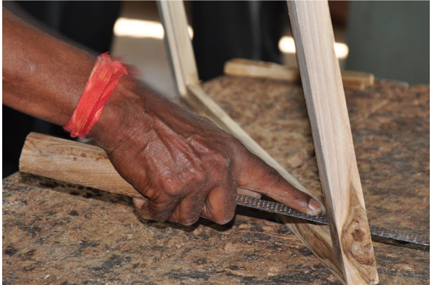
Riffler used to smoothen the curved surface.
