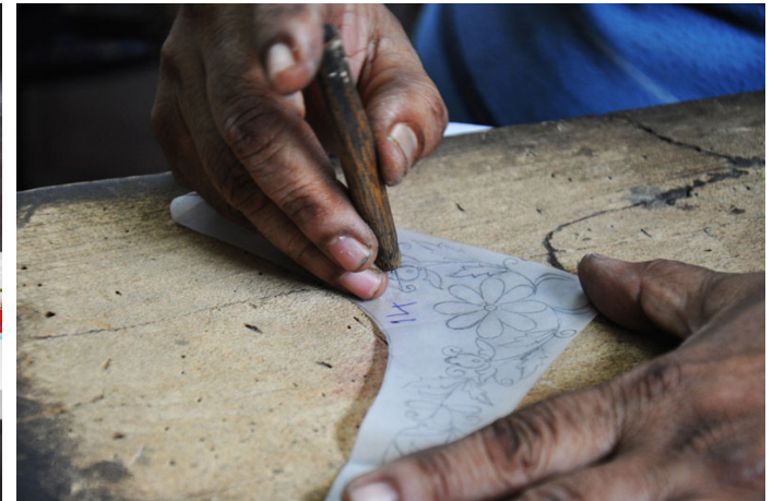
A sharp pointed tool is used to make small holes on traced design.
