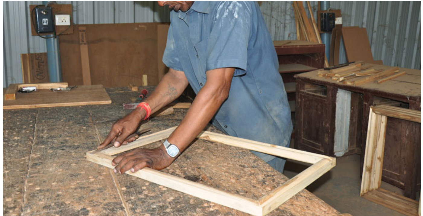
Rectangular wooden frame made of teak wood.
