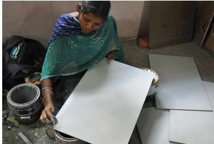
Artisan coating luppa paint on the wood board.
