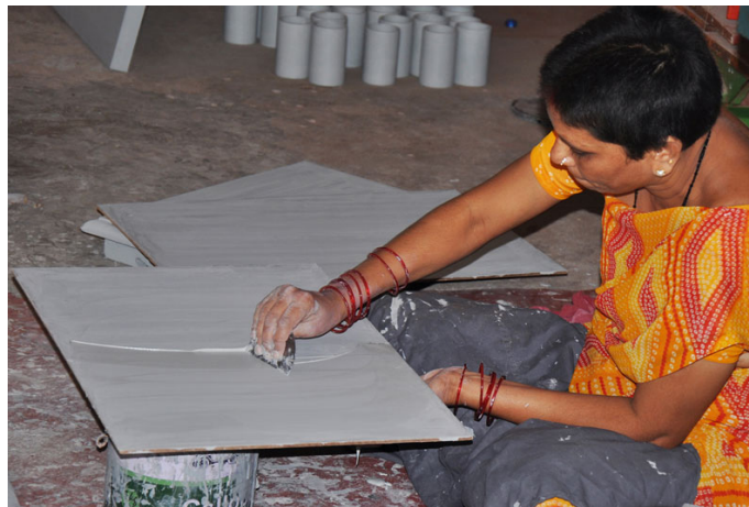
Nearly nine to ten coats are coated on the plank.
