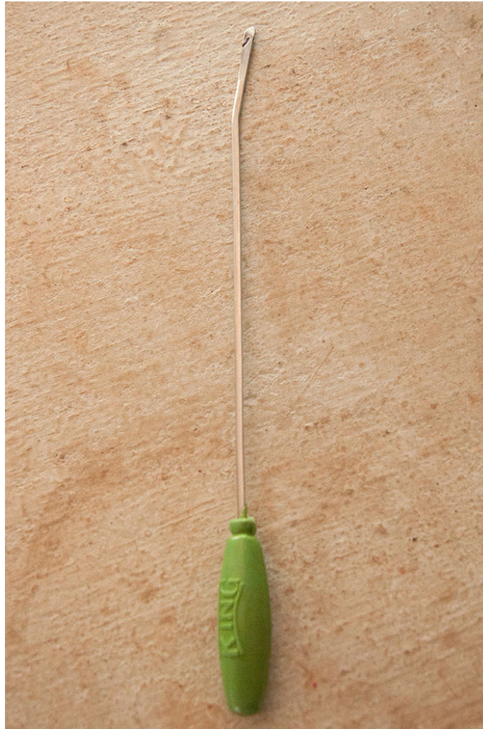
Metal hook is used while weaving to arrange the design patterns in order.
