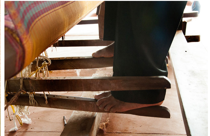
Pedals, which helps in lifting one set of warp threads at a time to have the shed opening for the fly shuttle insertion.
