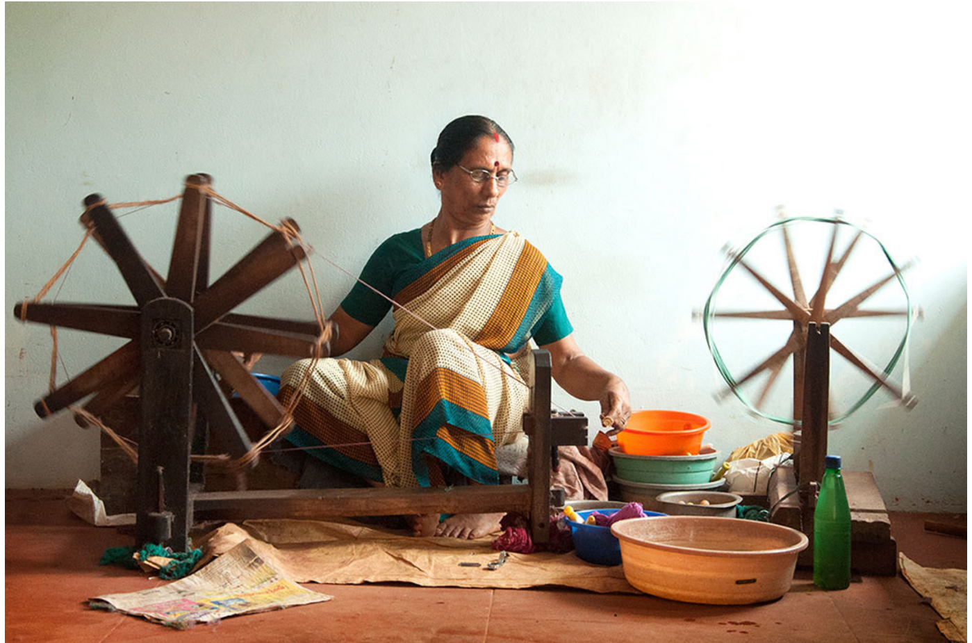
Yarns are wound by the Charaka equipment to the pirns.
