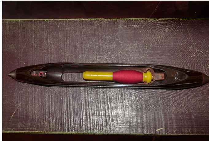
Fly-Shuttle: This tool helps to carry the cotton threads, through the warp sheds.
