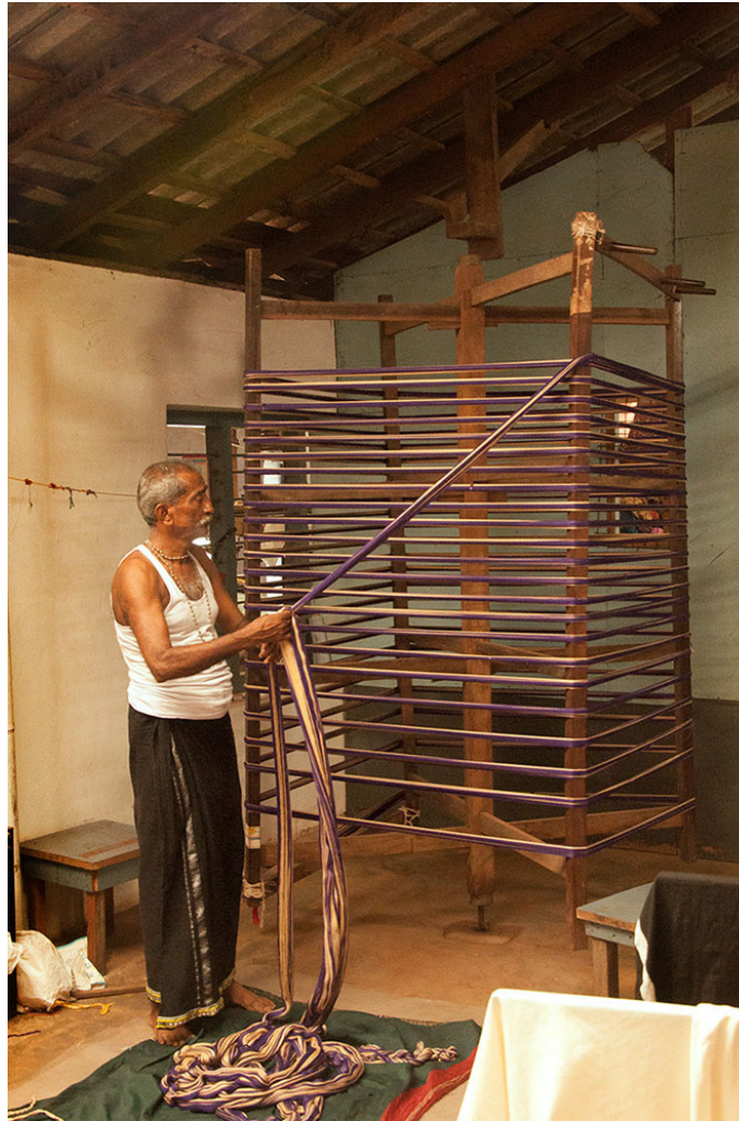
The cotton threads are taking out from the warping equipment.
