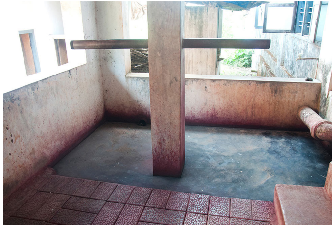
Metal rods are generally used to squeeze the yarns after dyeing.
