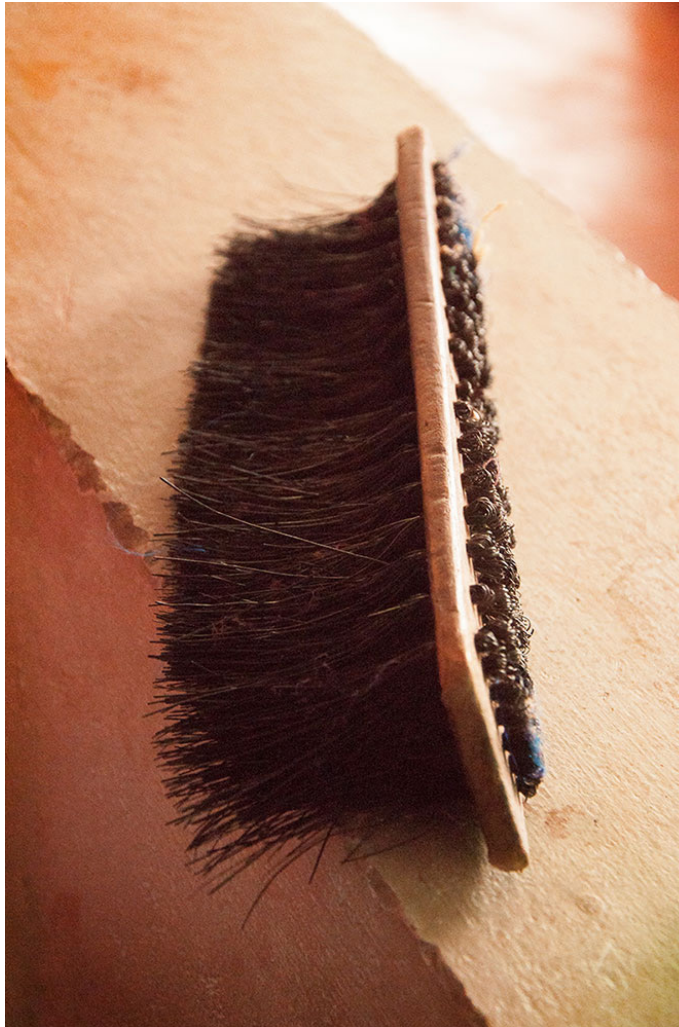
Palm fibres Brush is used to apply the starch on yarns on the loom.
