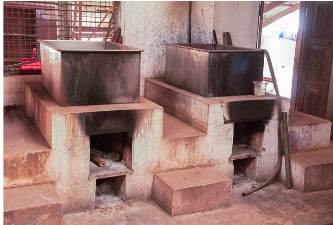
Metal tanks (Two numbers) are specially made for the dyeing purpose using wood fire method.
