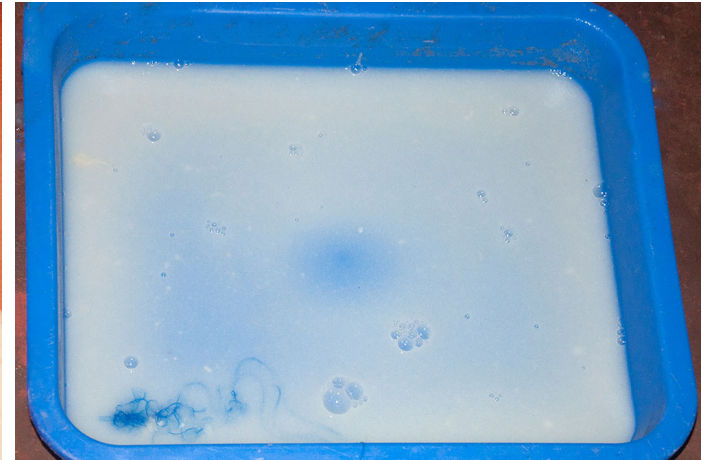
Starch is applied on threads to gain strength.
