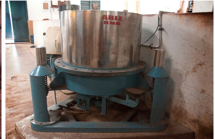
Electric spinning machine used to remove excess of water in yarns.
