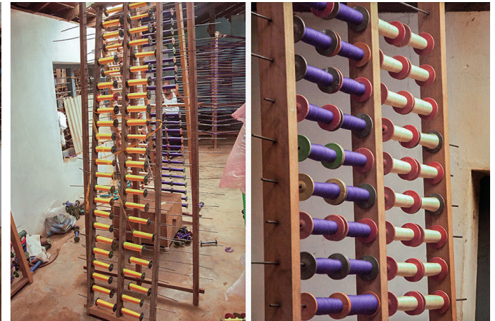
Creels: The coloured bobbins are placed on creels as per the pattern for warping.
