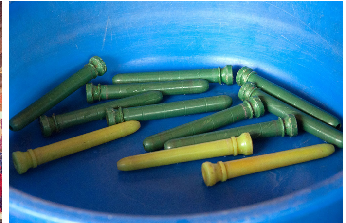
Plastic pirns are used to wind the yarns for weaving.
