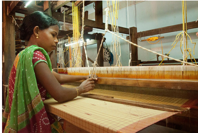
Weaver pulling rope to move shuttle between the threads of the warp.
