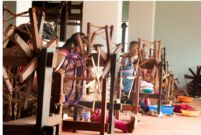
The cotton threads from the rolls are spun into the spindle by using Charaka.
