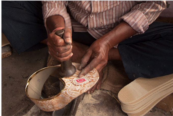
Golden topline is attached by stamping as border.
