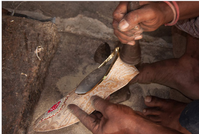
Shoes are stitched by piercing a sharp chisel.
