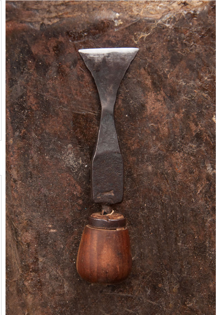
Flat chisel is used to cut the extras of shoes.
