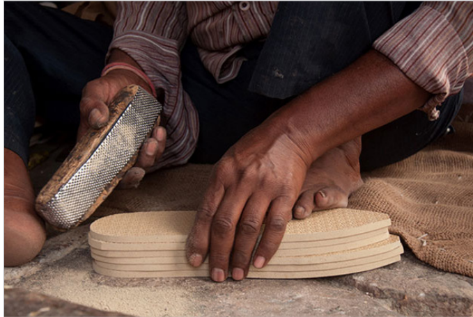
Artisan is shaping the Sole part of sherwani shoes.
