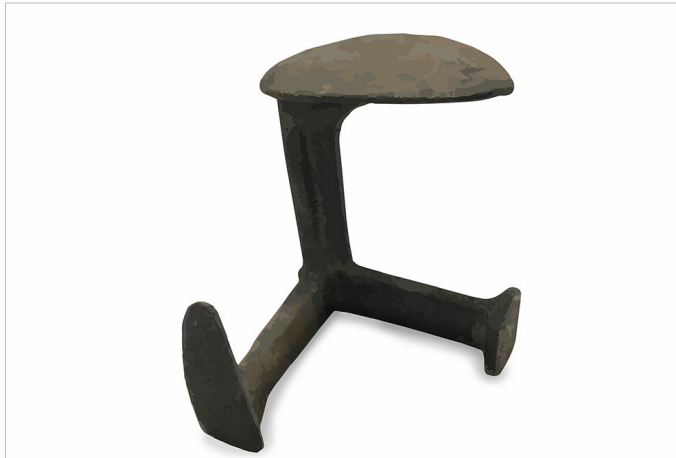
Cobbler stand tool is used to give shape to the shoes.
