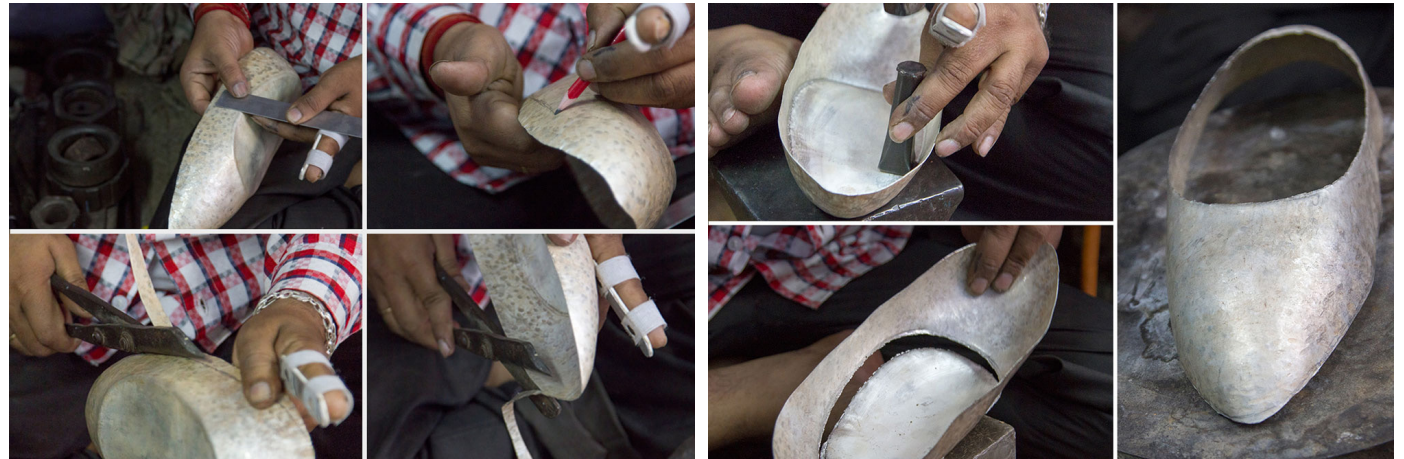
Shoe is measured to the sample shoe size and the unwanted area is removed using metal sheet cutter.
