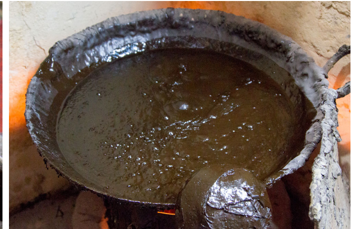
Lacquer: used in embossing work which makes embossing easier without cracking.
