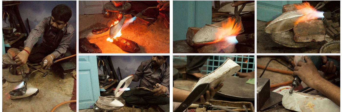
Embossing work is being made on the silver shoes using customized chisels.
