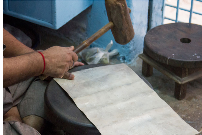
Leveling the silver sheet by hitting with wooden hammer.
