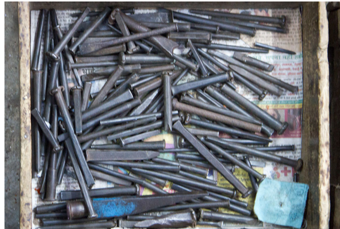
Customized chisels: used in embossing work.
