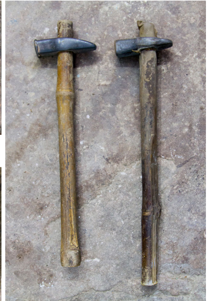
Hammers: used for hitting silver sheet to get a required shape.
