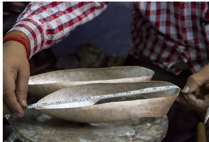
The base size is being measured using the measuring tape.
