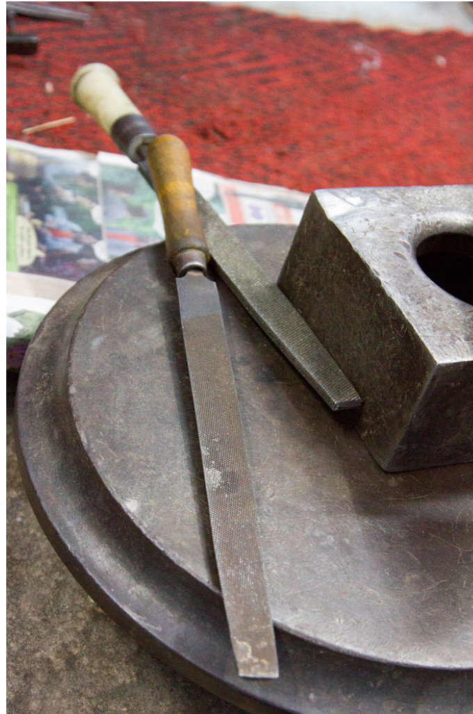
Filers : Used to smoothen the edges.
