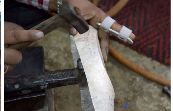
Basic shape is being given by hammering over the silver sheet.
