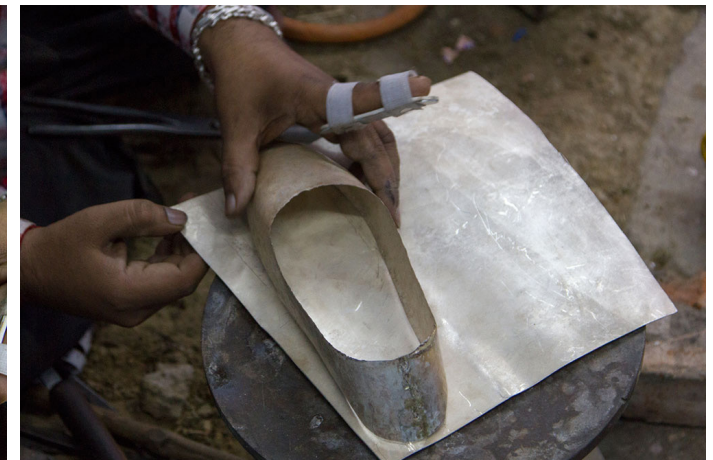
Measurement for the shoe base is being measured by placing basic shoe structure over the silver sheet.
