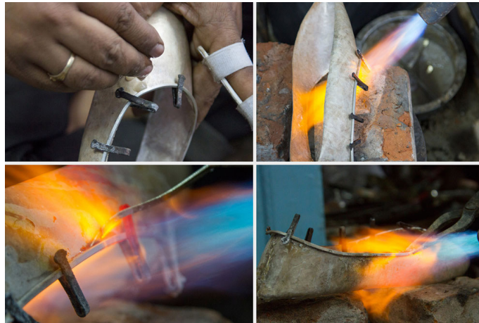
Silver wire is heated and being fixed over the shoe topline.
