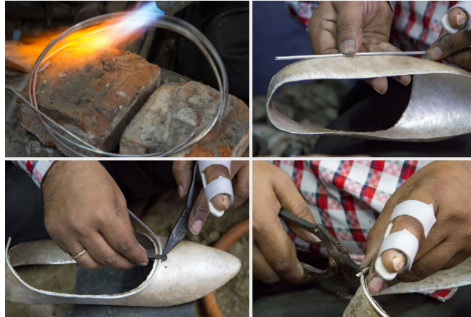
Silver shoe base is obtained by cutting the silver sheet.
