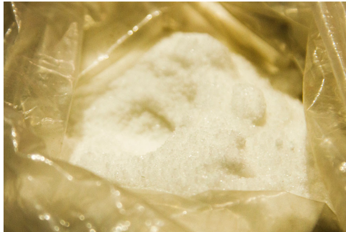
Brazing flux powder used while joining the different parts of the Kamandalu.
