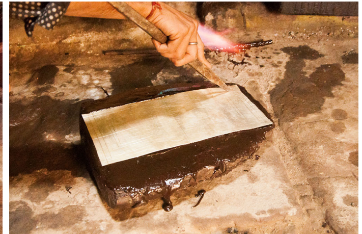
Silver sheet is pressed in the corners of the silver sheet to make it stuck to lack.
