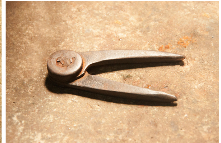
Compass used for measuring the distance while sketching on the silver sheet.
