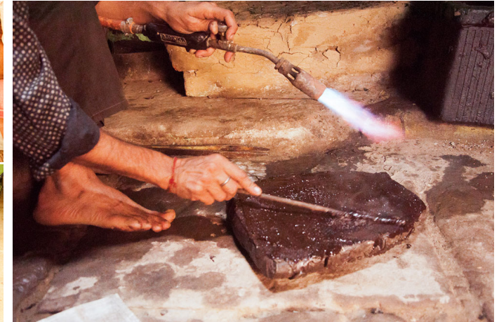
Lack is spread even on a stone evenly by melting the lack through fire gun.
