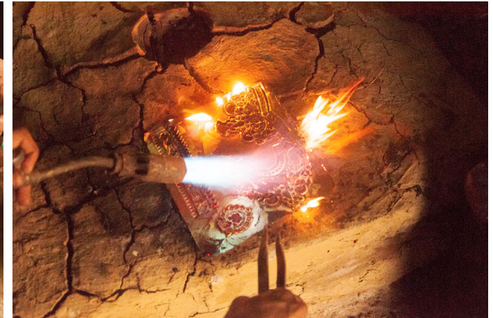
Then the lack is melted again to separate the designed silver sheet from lack.
