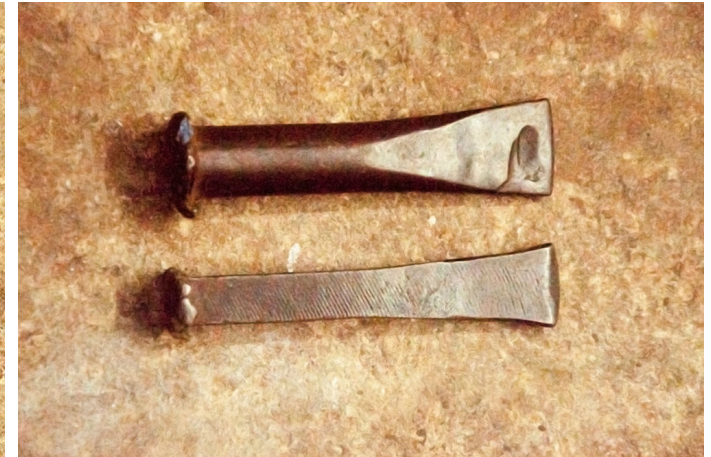
Chisels are used to etch designs on the silver metal.
