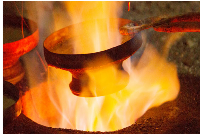
Then the parts of the kamandalu that joined with the bonding agents are fired in the furnace.
