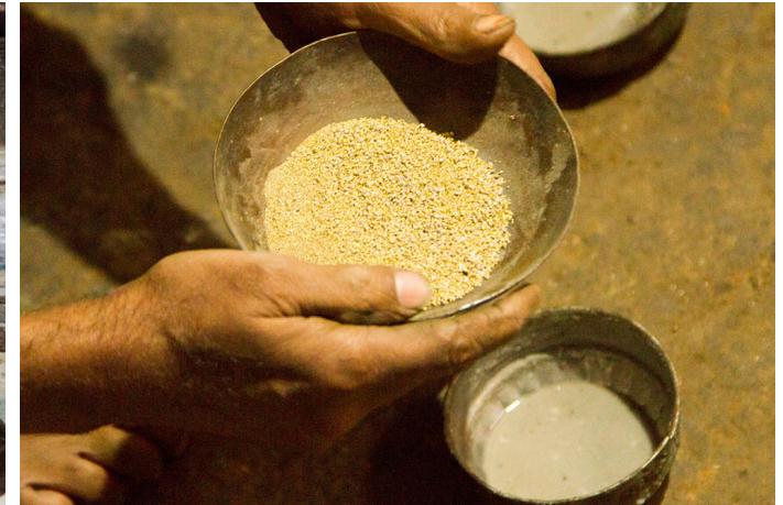
Brass powder that is used for filling the gaps between the two parts.
