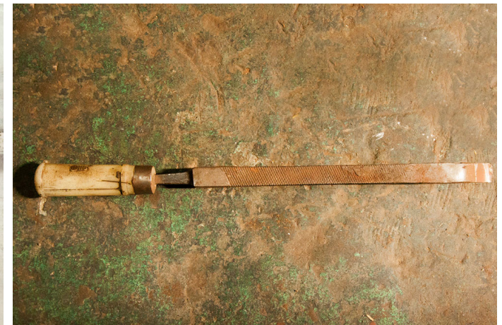
File used for polishing the utensils.
