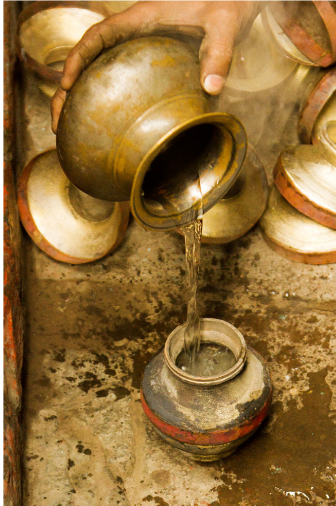
Water is poured on the fired kamandalu to calm down the temperature.
