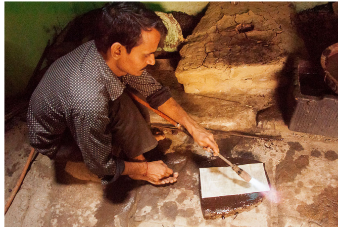
On lack the silver sheet is stuck for the grip purpose.
