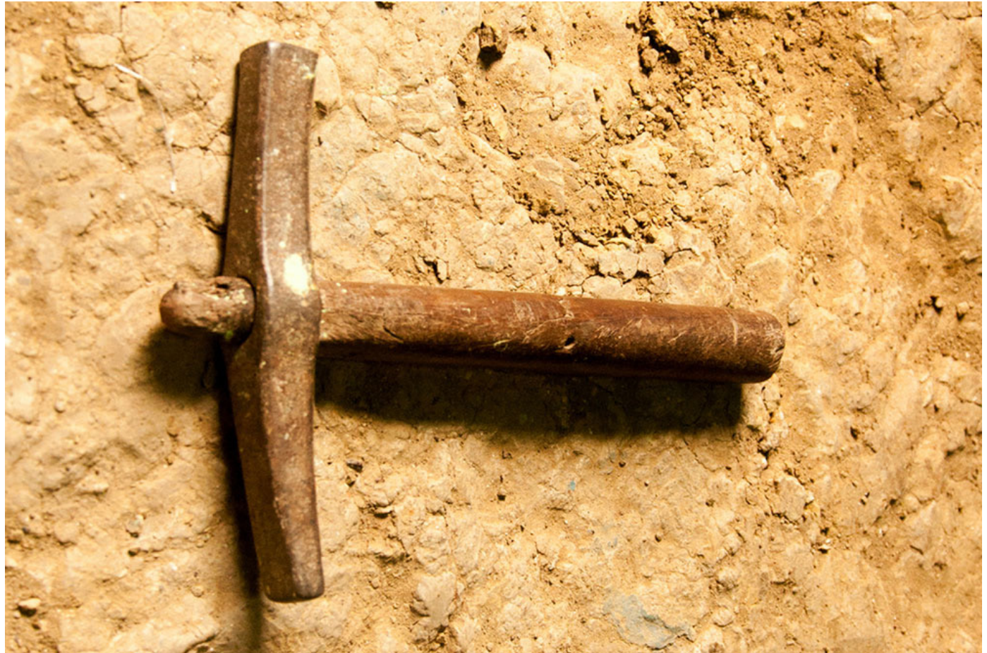
Hammer is used while engraving the silver plates.
