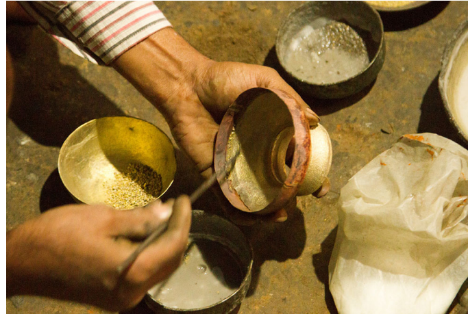
By using a brush this mixer is applied inside portion of the joints.
