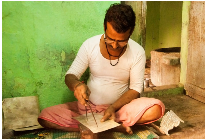
Silver sheet is measured before the design is drawn on it.
