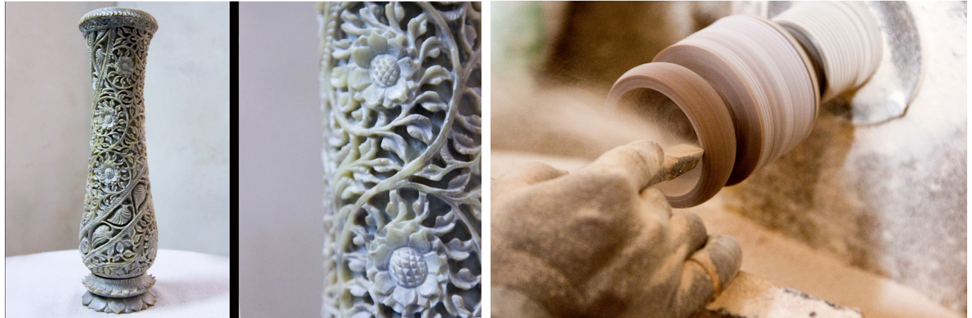
Stone is carved with help of Chisels tools by using turnery machine.
