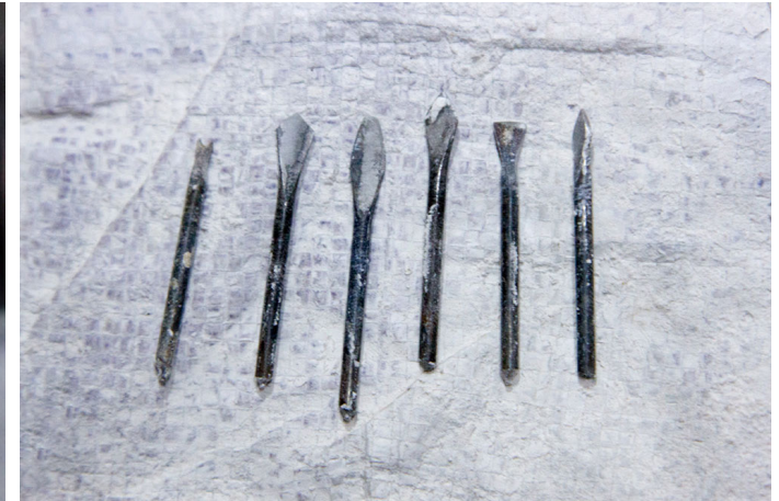
Several types of chisels tools used for carving process.
