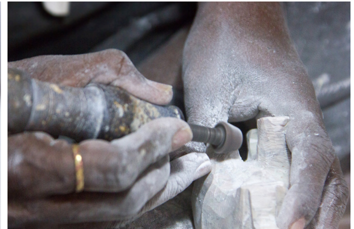
Leg parts is getting carved by using power carving sharp tools.
