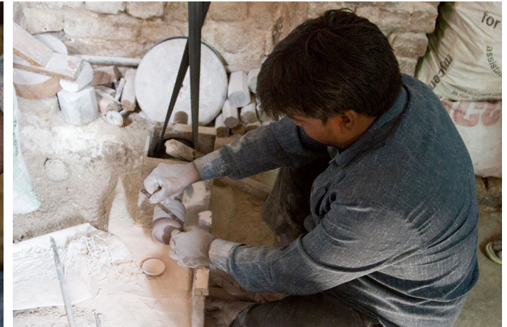
Hacksaw blade is used to cut the finished product from stalk.
