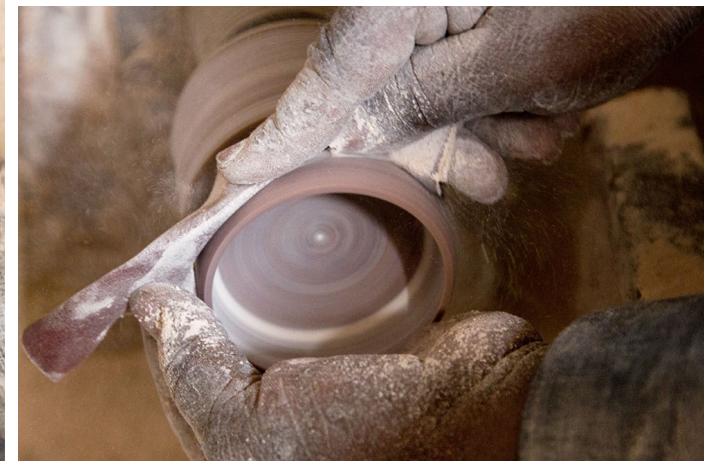
Emery sheet is used to remove rough surface on the bowl.
