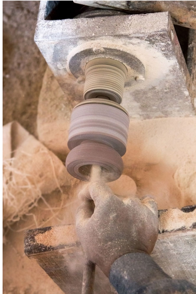
Artisan creating a hollow form of the bowl by using turnery machine.
