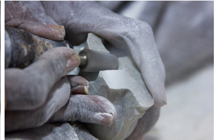
The block of stone is roughly shaped by using power carving sharp tools.
