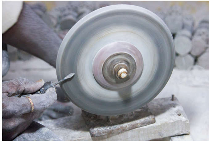
Artisan sharpening the chisels tools, using grinding wheel.
