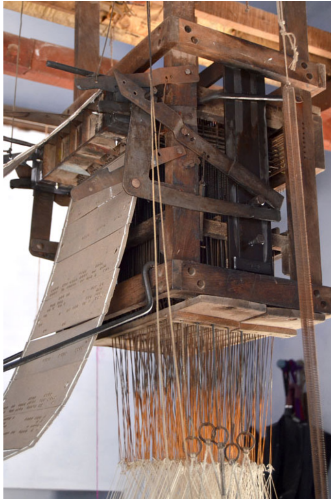
The heald (part of the loom) moving the warp threads up and down.
