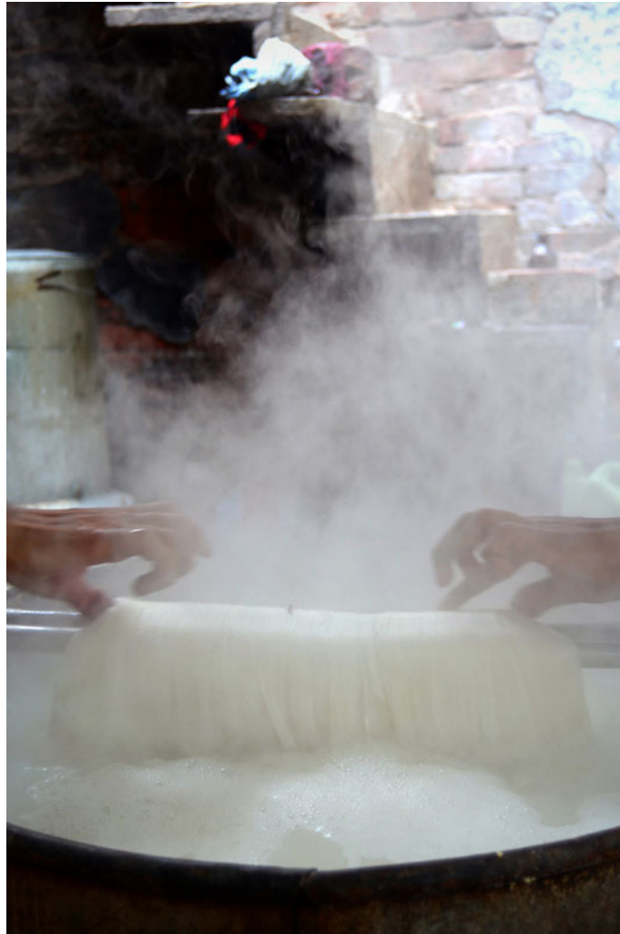
Yarn being boiled in soap water to increase pliability and give a smooth and shinier texture.
