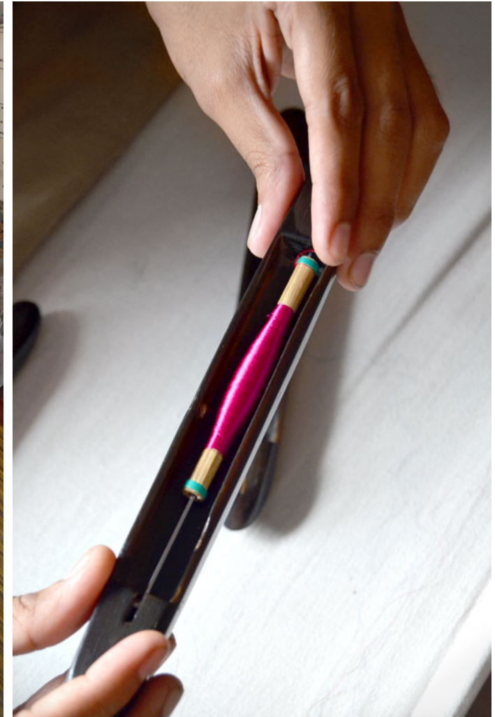
The weft-yarn used in a shuttle called 'dharki' is thrown from one to other side while weaving.
