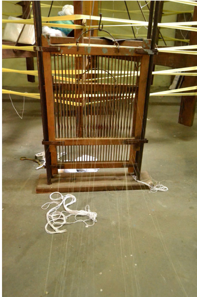
Reeling machine being fed by yarn, winding them and forming the skein for warp.
