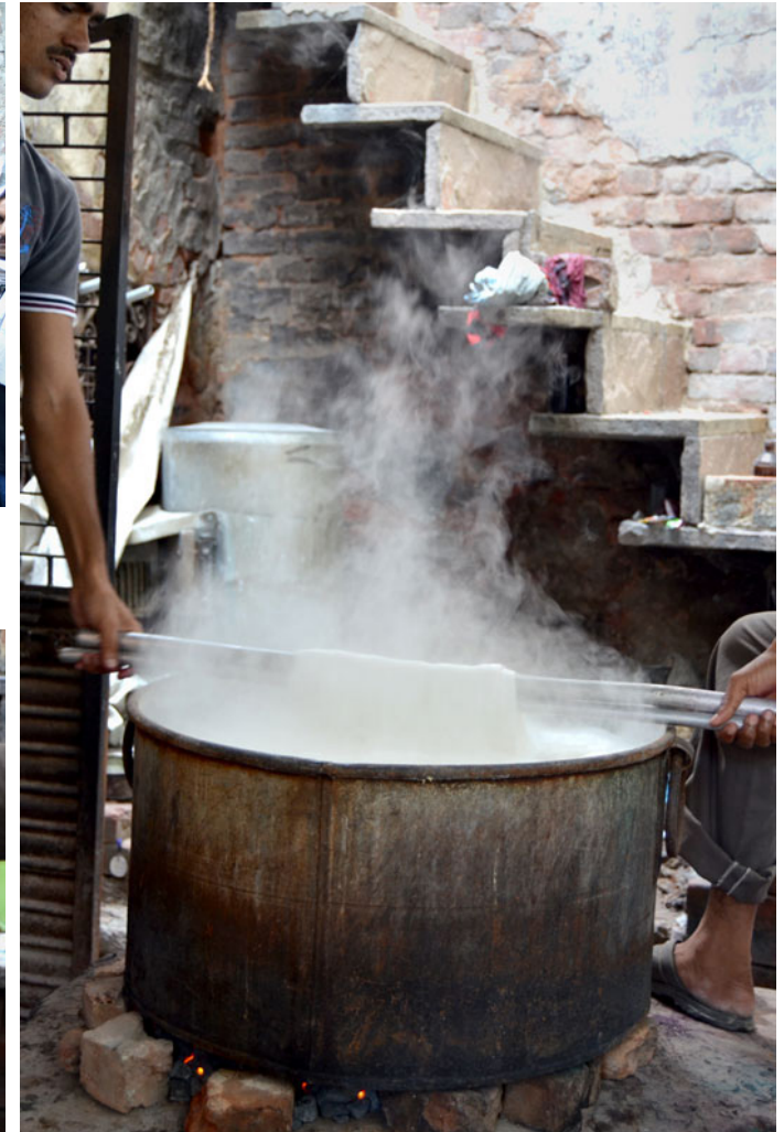
Yarn being boiled in soap water to increase pliability and give a smooth and shinier texture.
