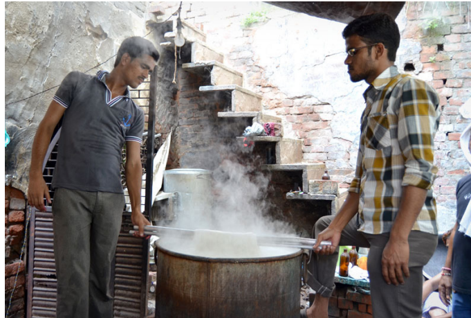
Yarn being boiled in soap water to increase pliability and give a smooth and shinier texture.
