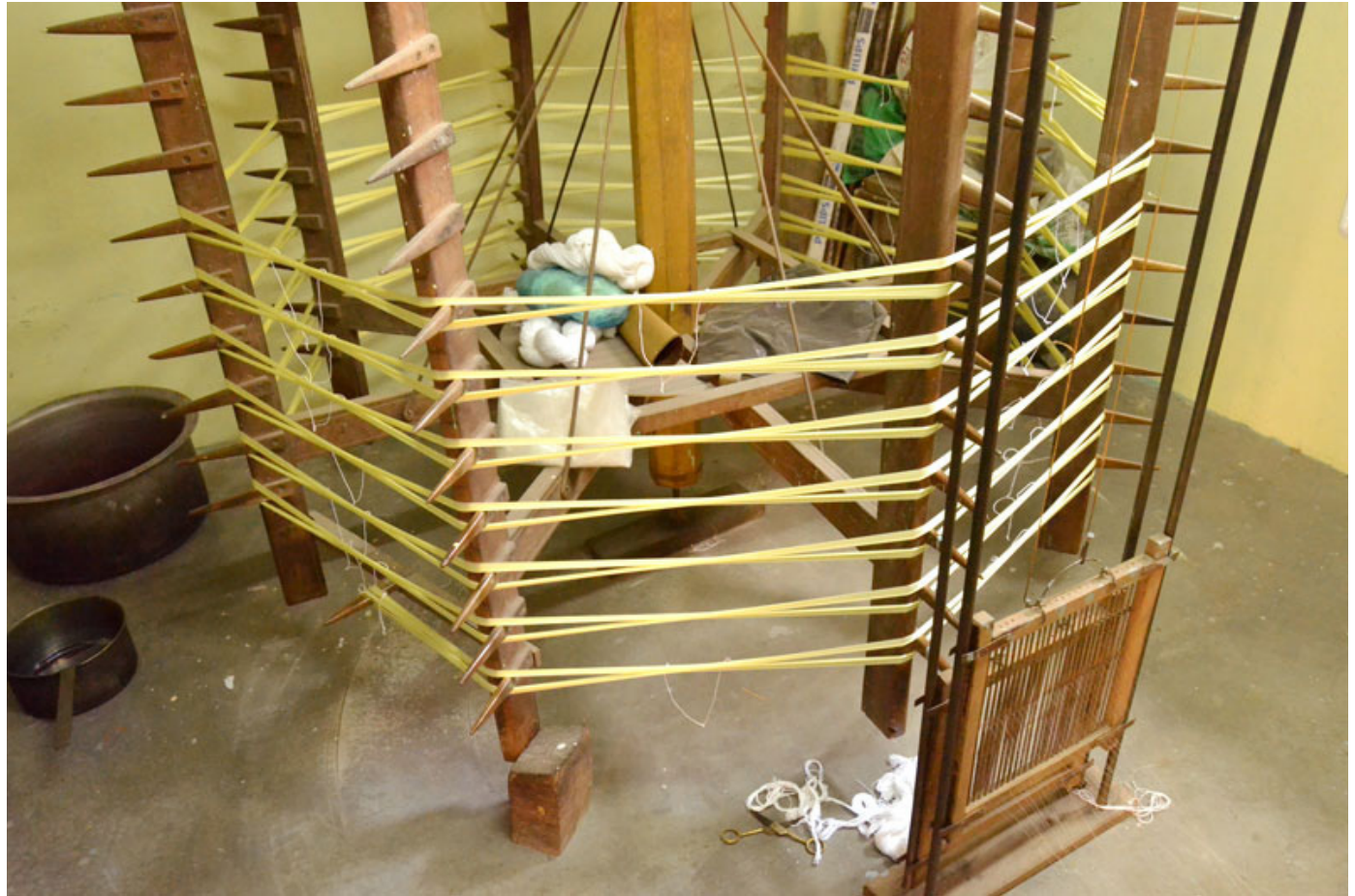
Reeling machine being fed by yarn, winding them and forming the skein for warp.
