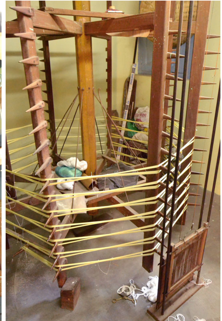
Reeling machine being fed by yarn, winding them and forming the skein for warp.
