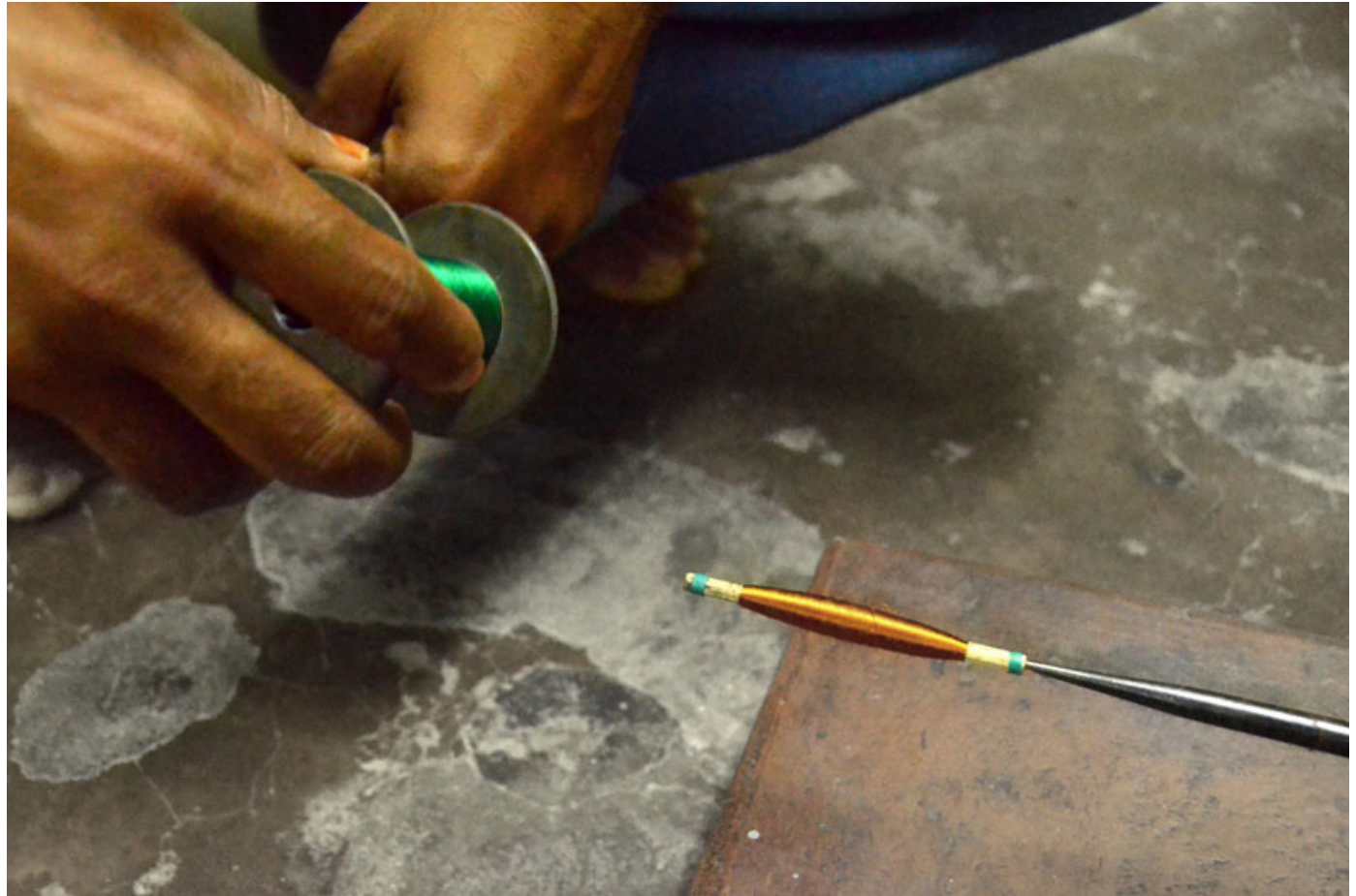
Spinning wheel being used for winding the weft yarn on nari (bobbins).
