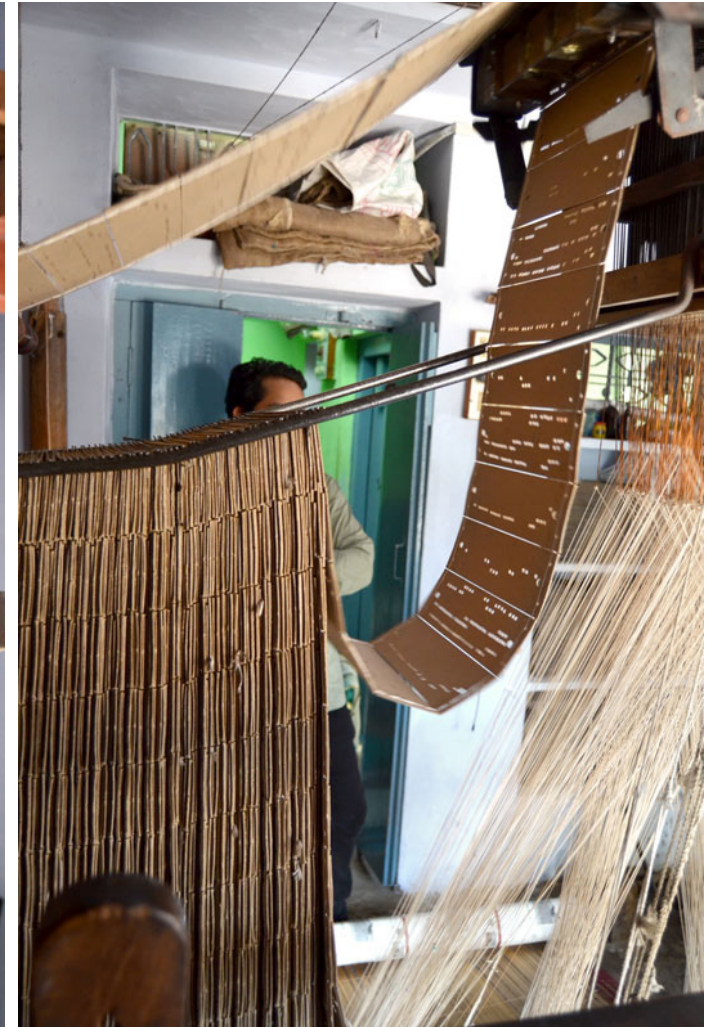
The heald (part of the loom) moving the warp threads up and down.
