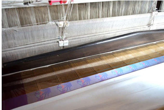
The cloth roll, which is at the front of the loom, rolling the fabric that is being constructed.
