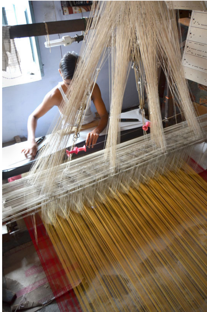
The reed (like a comb) controlling the separation of the warp threads while weaving.
