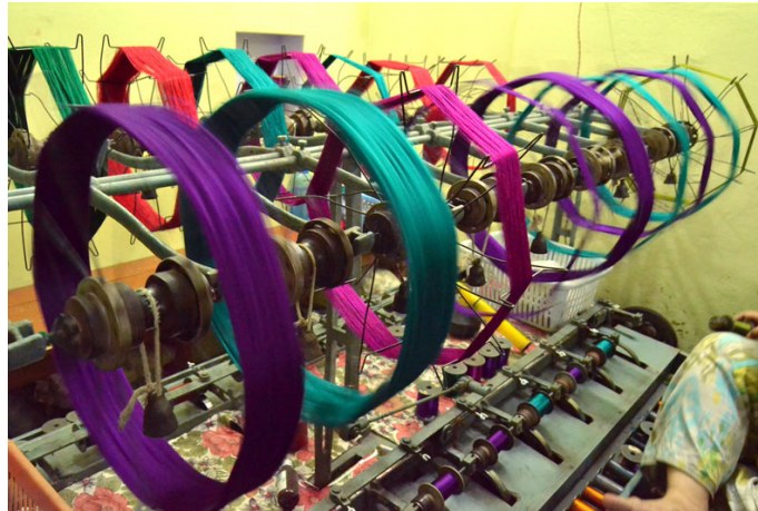
Yarn for the weft being reeled on a small cylindrical object.
