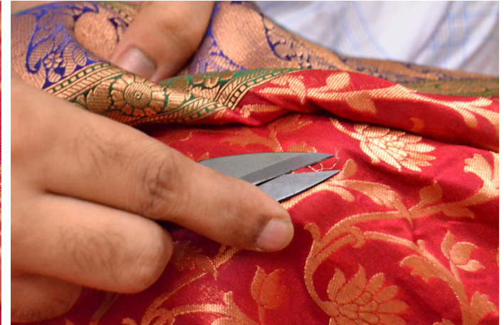
Karigar cutting tiny threads left over from weaving on the reverse side of the fabric to make it more transparent.
