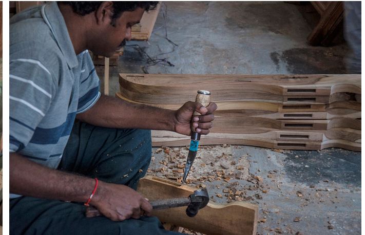
Making a small rectangular hole.
