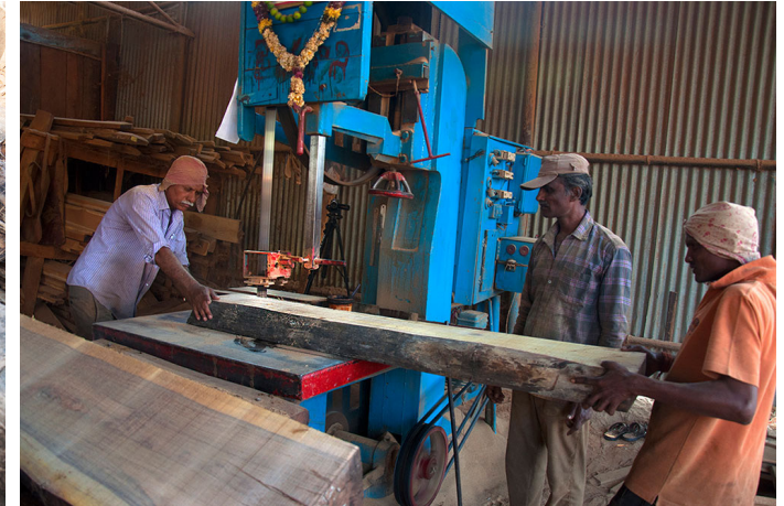
The wood is sliced removing outer layer by passing it through a machine.
