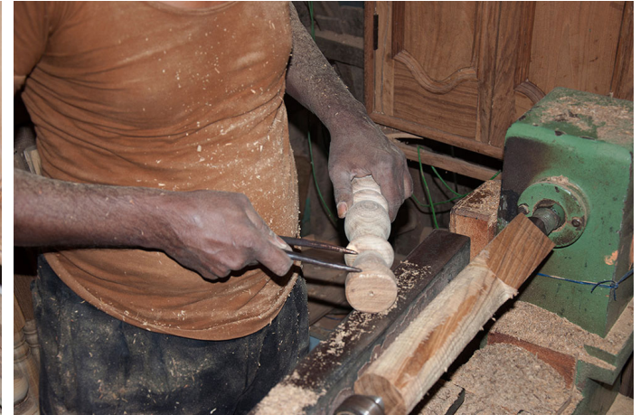
Artist measuring with the help of measuring gauge.
