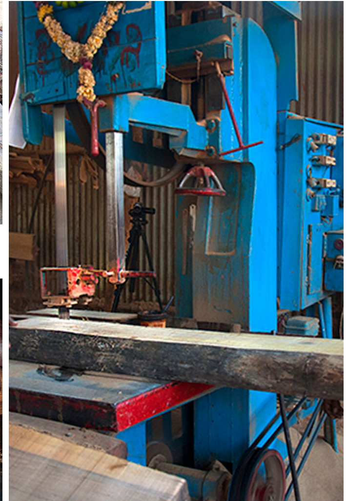
Wood is put through a machine to slice out outer layer.
