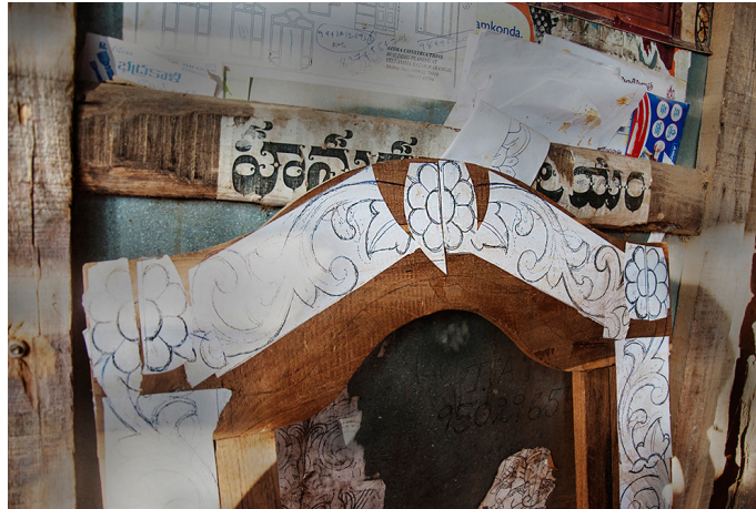
A sketch sheet of floral design placed on wood to be carved.
