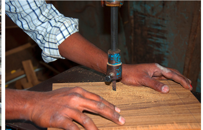
Cutting a plank of wood with help of saw machine.
