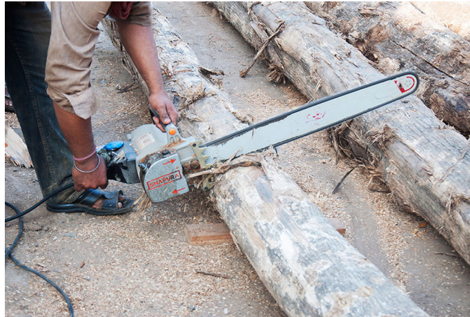
Chainsaw machine helps to cut to required length of wood logs.
