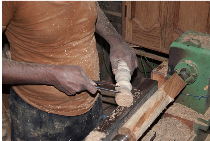
Measuring with help of gauge.
