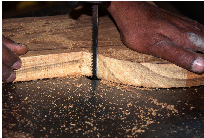
Wood planks are cut in a designed form with help of machine saw.
