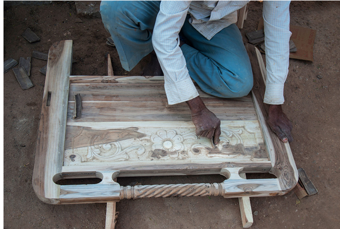
Giving a fine finish by rubbing sand paper over the wood.
