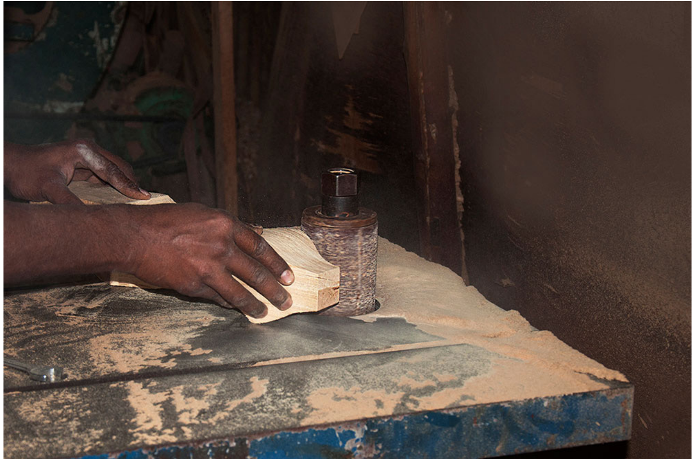
Sanding wood with help of mechanical sander.
