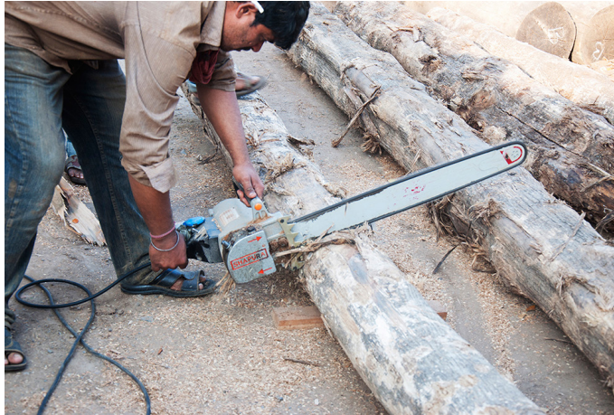
The wood log is cut with help of chainsaw machine.
