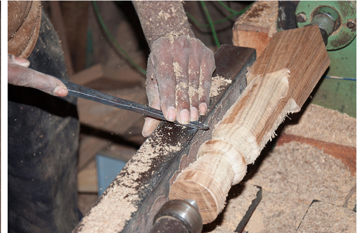
The making of a leg with help of wood turning machine and filing gouge.
