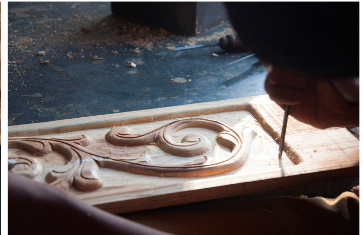
Carving wood evenly to form a flat surface and make design visible.
