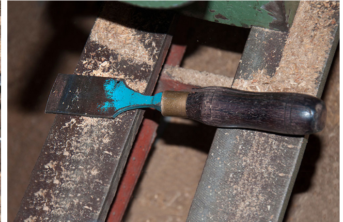
Butt chisel used to carve wood.
