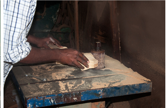
Smoothing wood with mechanical sander to give a better shape.
