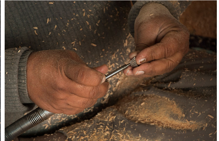
Artisan then changes the drill bit to a smaller bit to carve even more details.
