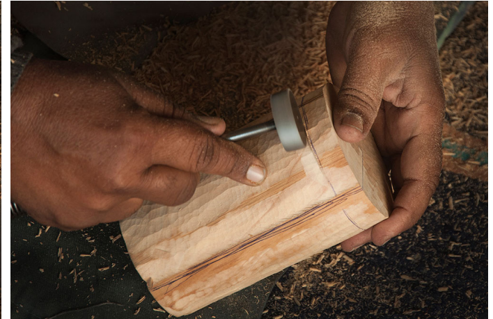
Artisan then drills away the excess wood with the help of markings.
