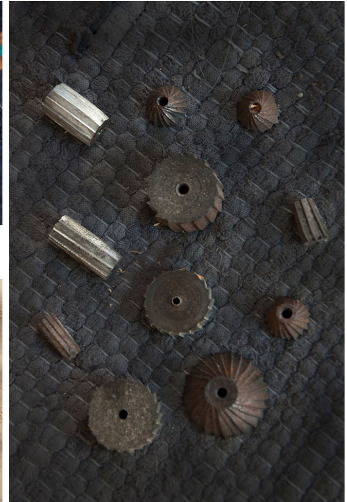
Various sizes and typed of drill bits used in carving the wooden block to a required shape.
