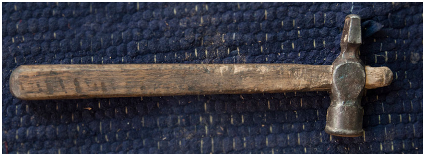
Hammer used in hitting the chisel, for carving.
