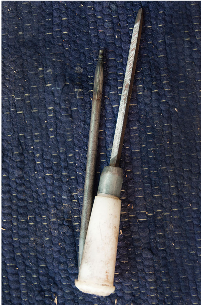
A large chisel with plastic handle, used in carving, along with the hammer.
