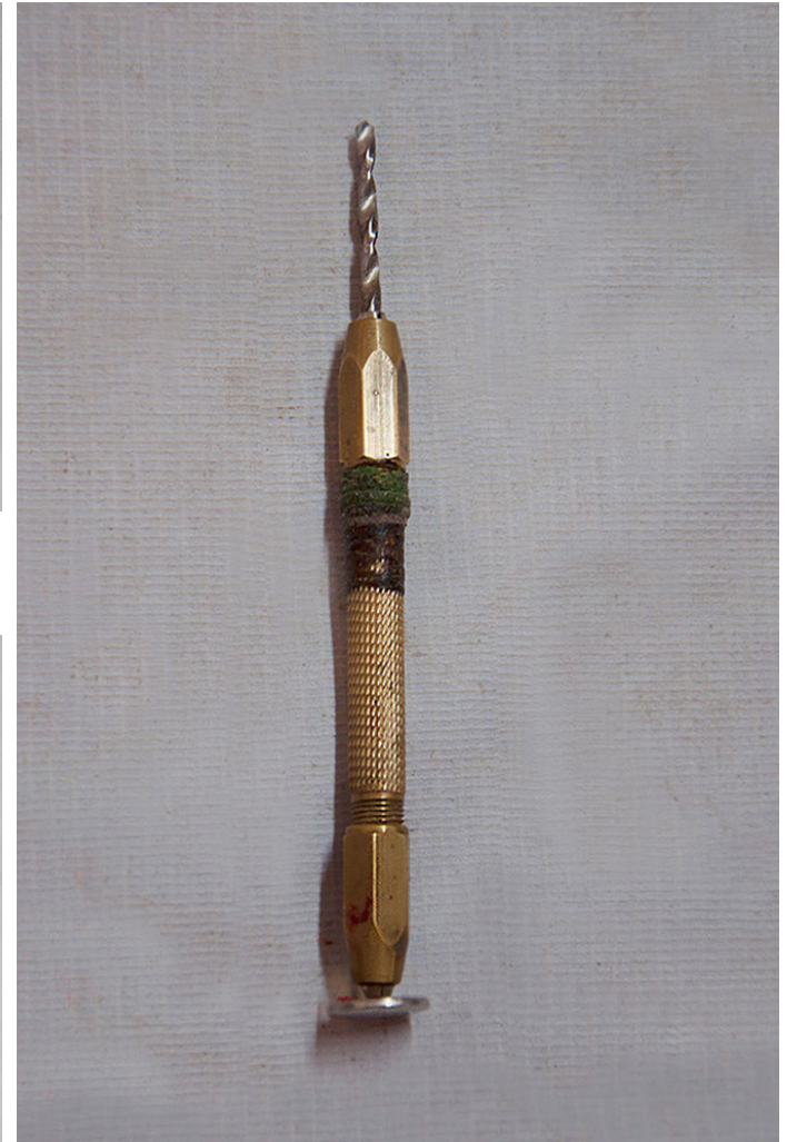
Drilling tool used to make a hole on wooden nameplate.
