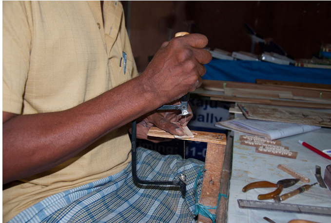
Carving out the name with the help of coping saw.
