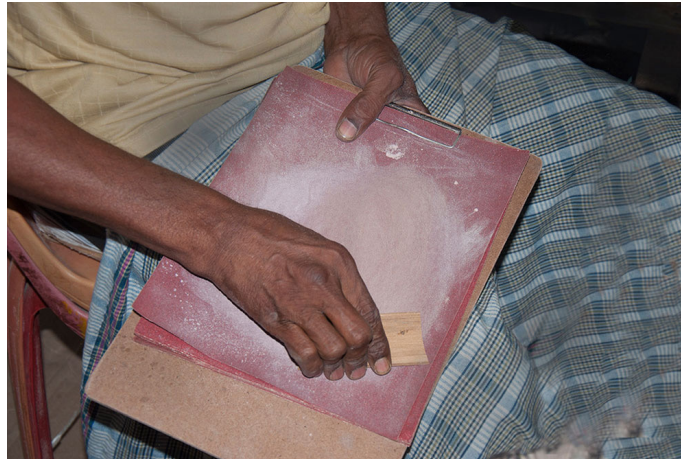
Rubbing the wooden nameplate on sand paper to smoothen the surface.
