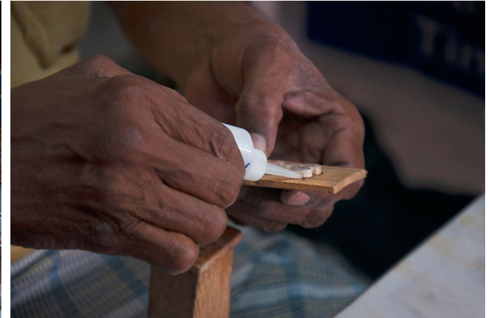
Gluing the cut wooden nameplate on another small piece of flat wooden plank.
