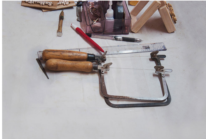
Pair of coping saws to carve and get cut out of names for the nameplate key chains, scale and pens.
