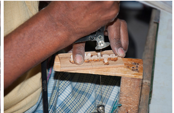
Cutting along the name with help of coping saw.
