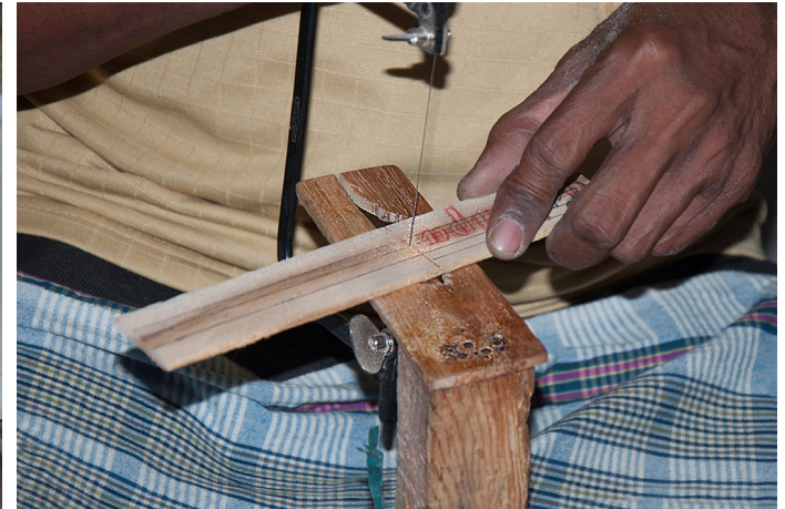
A wooden stand with a hole to help handle coping saw well.
