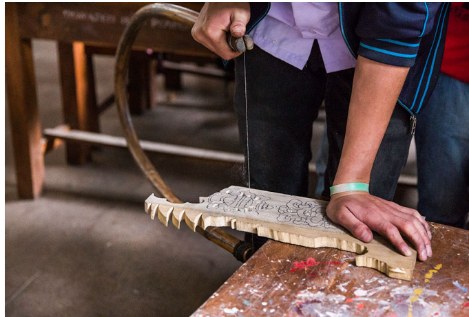
Cutting the wood using jue (wire).
