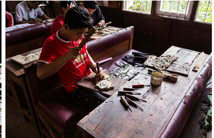
A special wooden hammer is used sometimes to carve hard areas.
