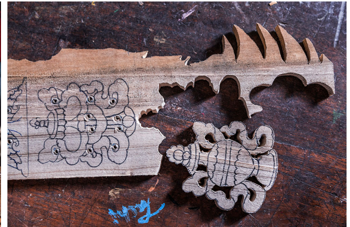
Wood cut using wire.
