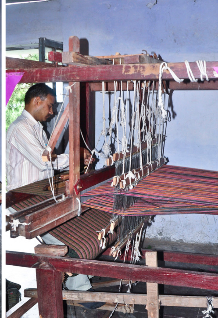
Woven cloth is wound onto weavers beam, which is near pedals.
