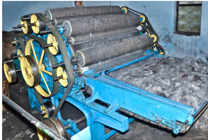
This process is done to separate the wool individually and arrange in parallel.
