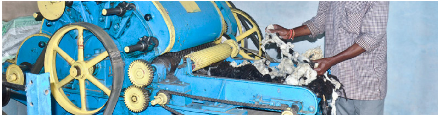
Raw wool is passed through willow carding machine.
