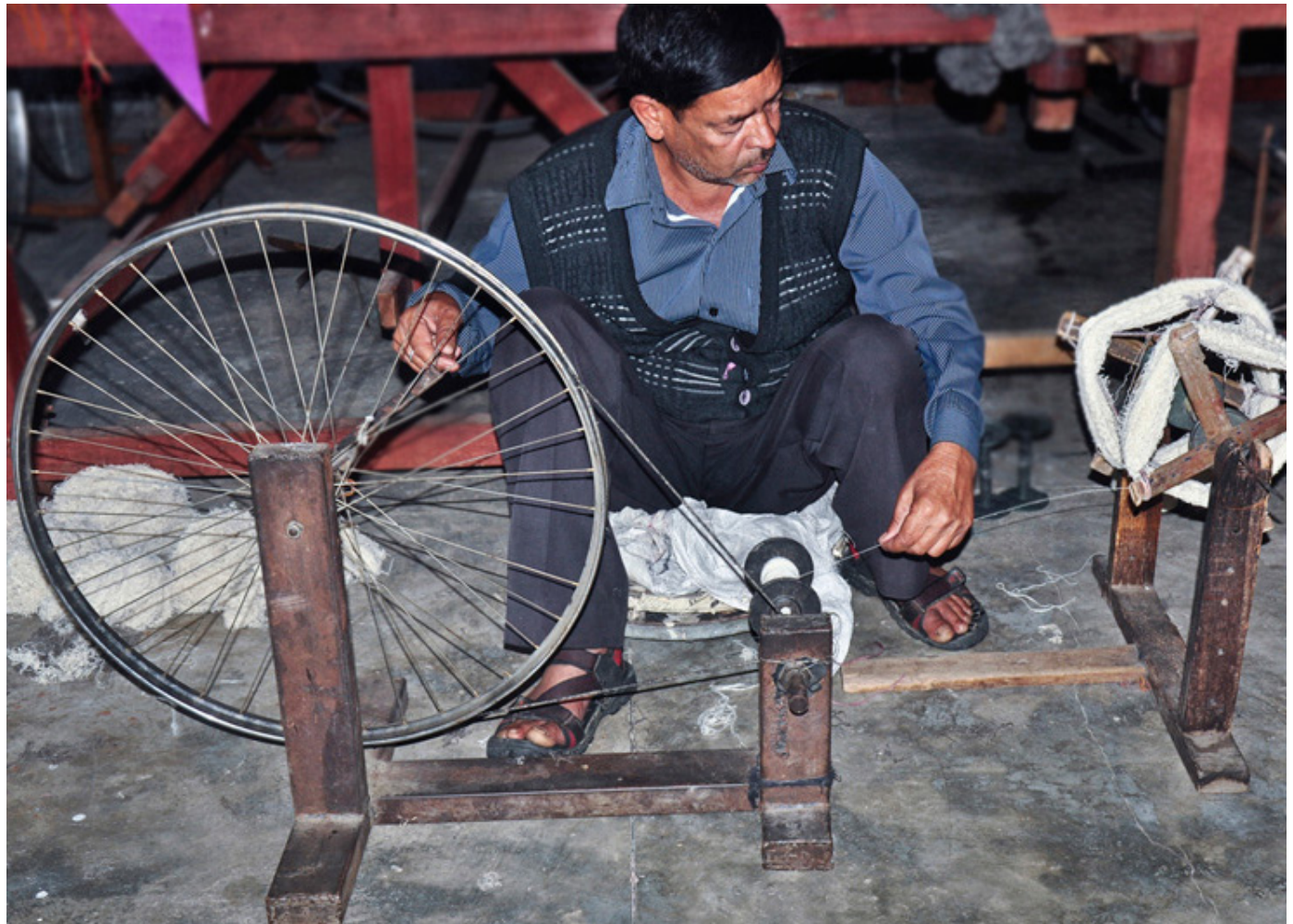
Manual spinning of wool with charkha (spinning wheel).
