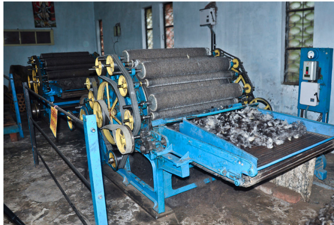
Carding process done using three carding machines.
