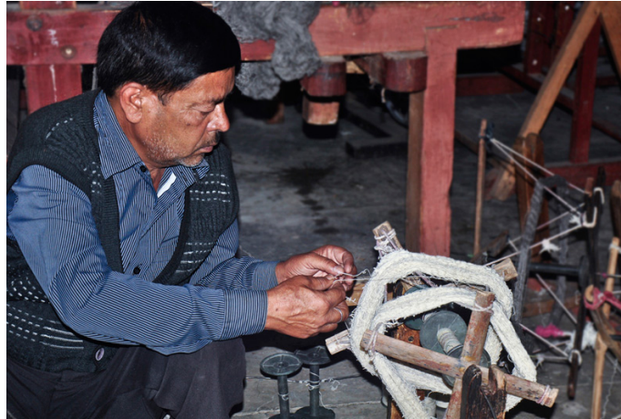
Strand from the wool bundle is taken and connected to spool.
