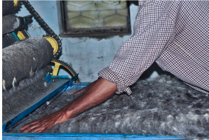
Wool sheet is placed in the tray of beaker carding machine.
