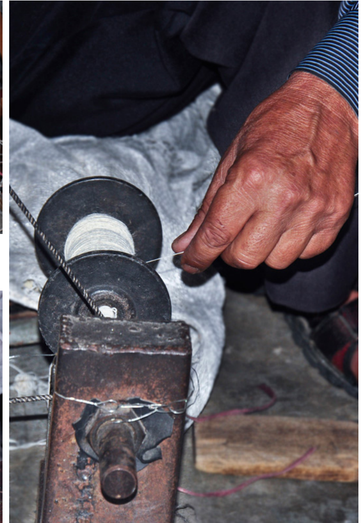
Wool from bundle is being reeled onto spindle.
