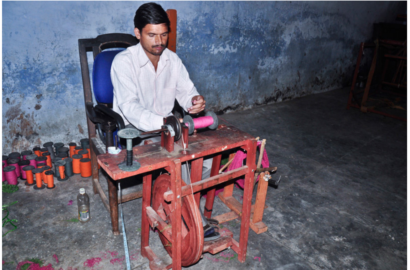
A different type of spinning machine operated by peddling.
