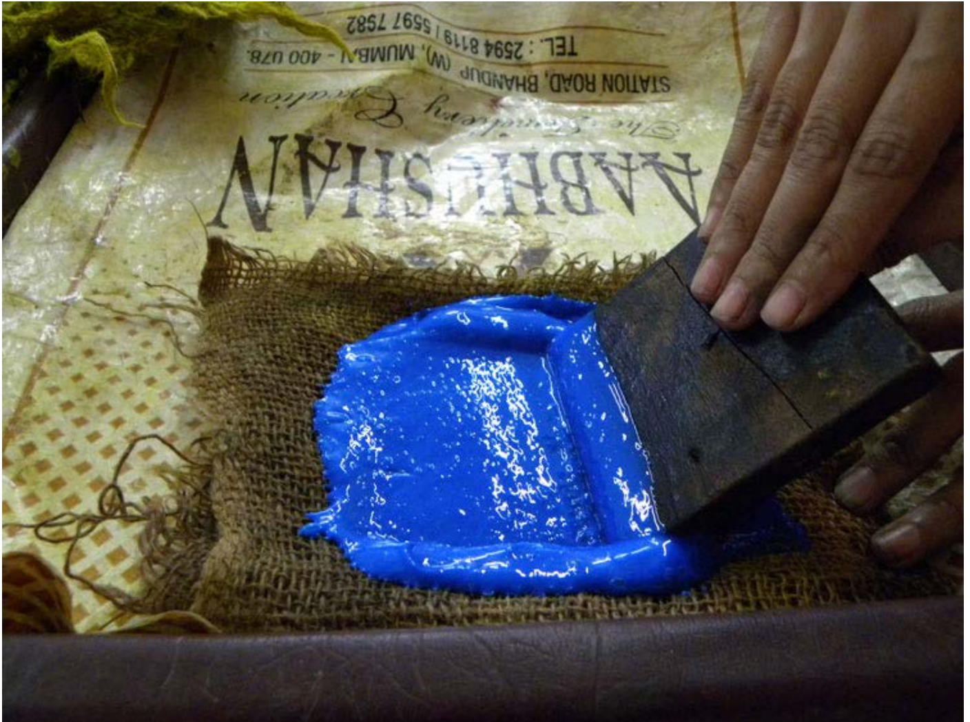
Mixing colour with binder and fixer and making colour pad to get a print.
