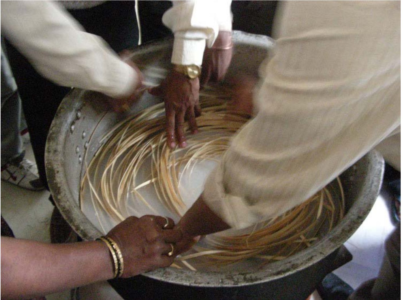
The strips are treated with boric acid in boiling water.
