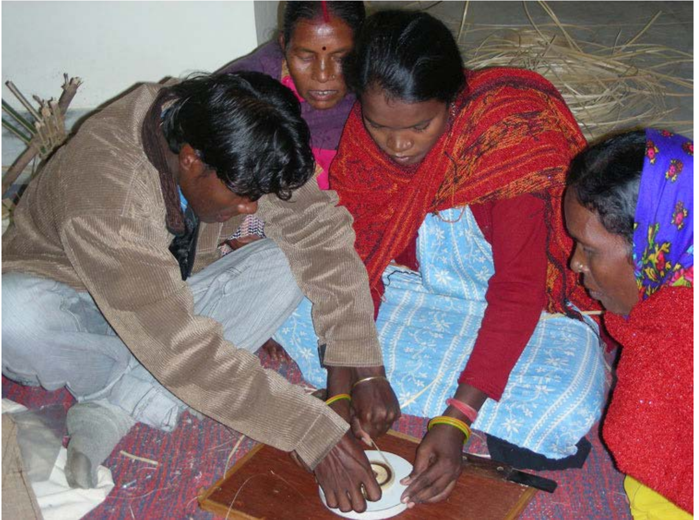
Thin long strips are pulled along circular die to make tea coasters.
