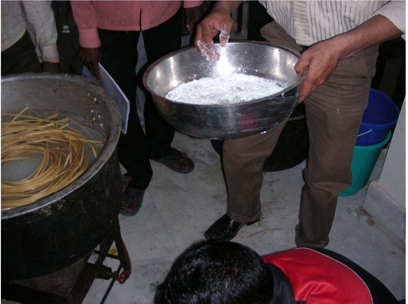
The strips are further treated with alum to impart anti fungal properties.
