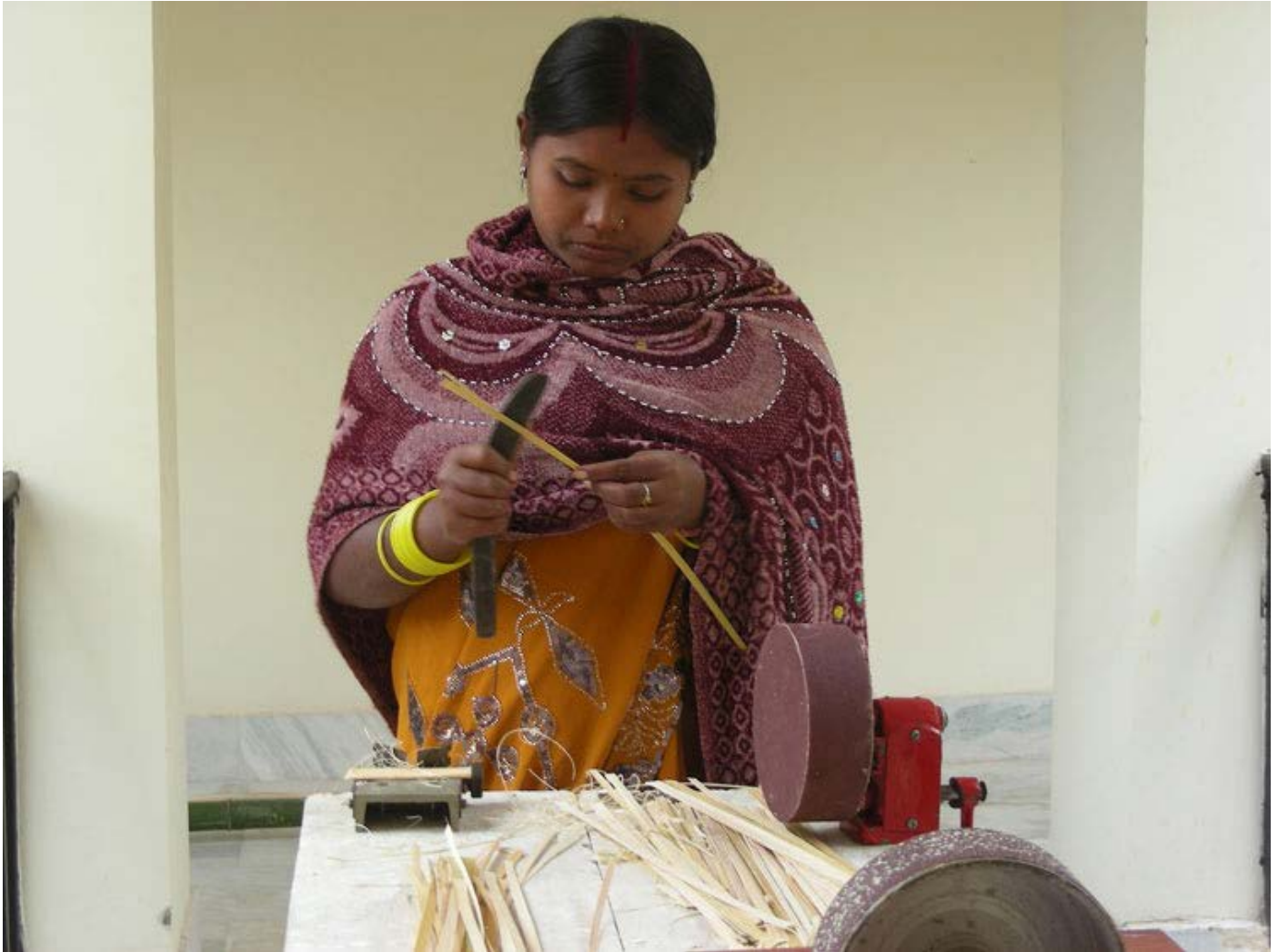
The bamboo strips are further given finer finish on a milling roller.
