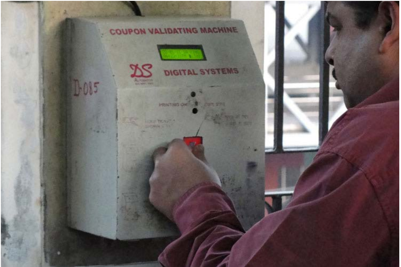
Mumbai Suburban Railway system – Coupon Validating Machine - The Coupon Validating Machine is used for punching (validating) the Ticket.
