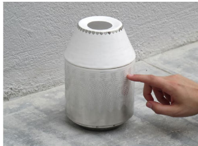
Metallic patterns are not only ornamental elements but play a functional role in the object. Each motif matches a particular setting : on/off, volume and frequency
