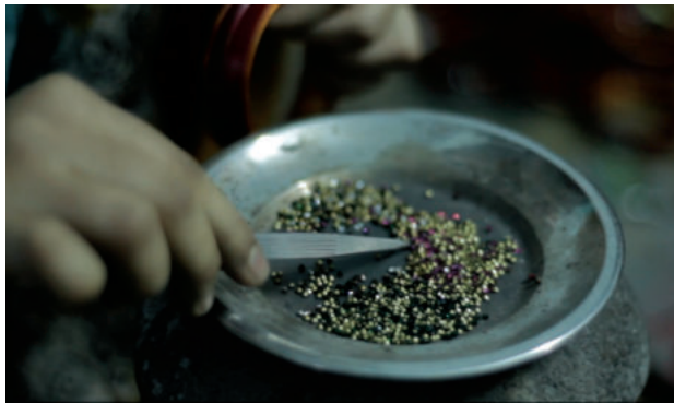
Fig. 9H: Heating the stones on a metal plate
