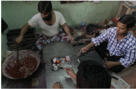
Fig. 7: Heating the Lacquer, Mixing the shining powder in to the lacquer, Molding the bangle, Preparing the aluminium wires for bangles.
