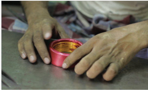
Fig. 9C: Wrapping the lacquer around the rings
