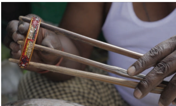
Fig. 10B: Self prepared tool for handling the bangle
