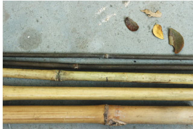
Image5. Showing different diameter bamboo which can be used for making the frame
