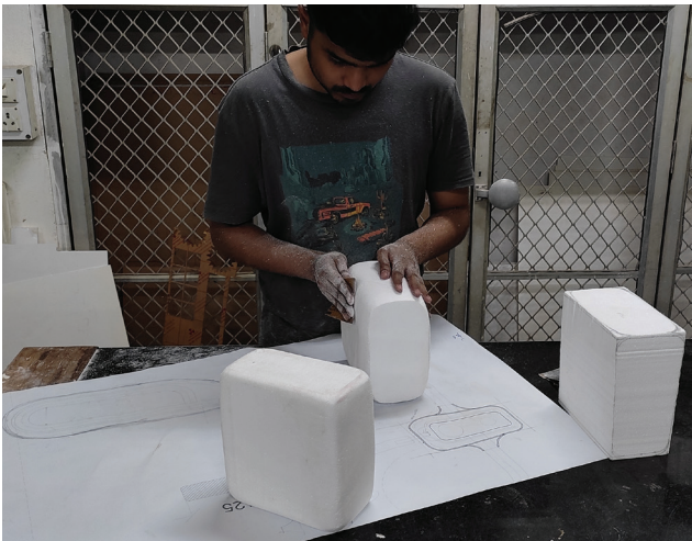
The central mechanism unit was carved out of thermocol, different shaped were explored.
