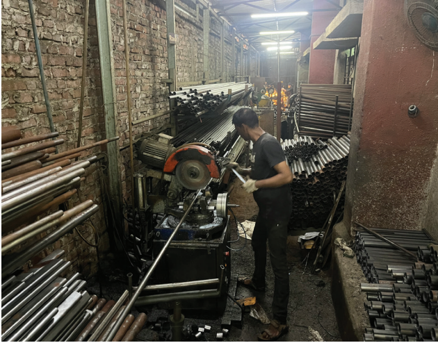
25mm dia and 2mm thick ms pipes were cut as per the desired sizes.
