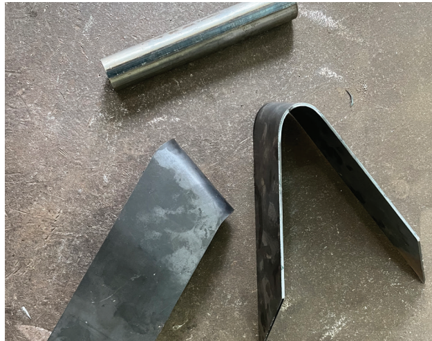
2mm thick ms sheets were laser cut and bend to form the brackets.
