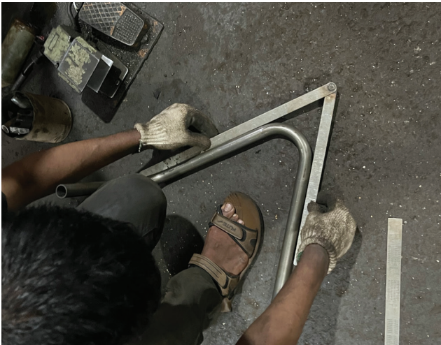
The bend degrees were crossed checked as per the drawings.
