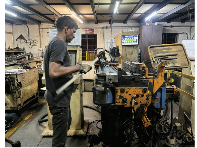
Data was feeded in the machine, which executed the bending.
