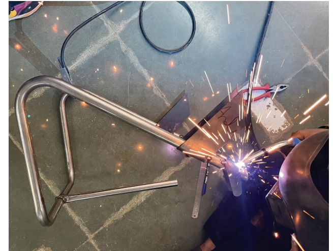
Meg welding was used to fix all the parts.
