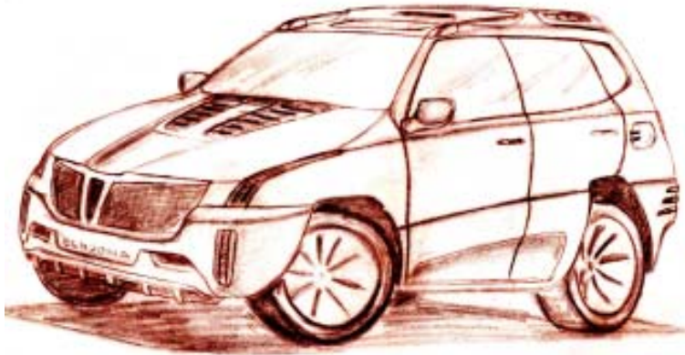
Alternative 1 No side claddings, narrow vertical long head lamps to give it a dynamic looks. Grille is massive and brings robustness. Air intake slits are provided in the bonnet that adds to the energy of the vehicle.
