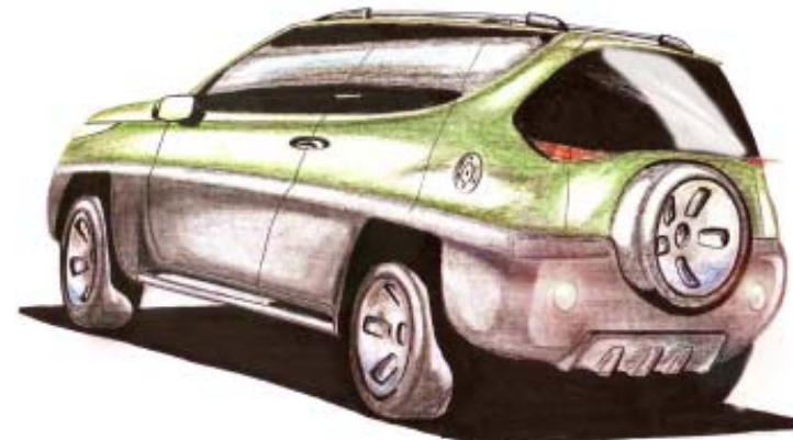
Alternative 4 Claddings going inward and reinforced steel tube tried out as side step. dynamic window line with tail lamps assisting the form to come out. spare tire sits firmly on the rear fenders. skid plate exposed in the rear.
